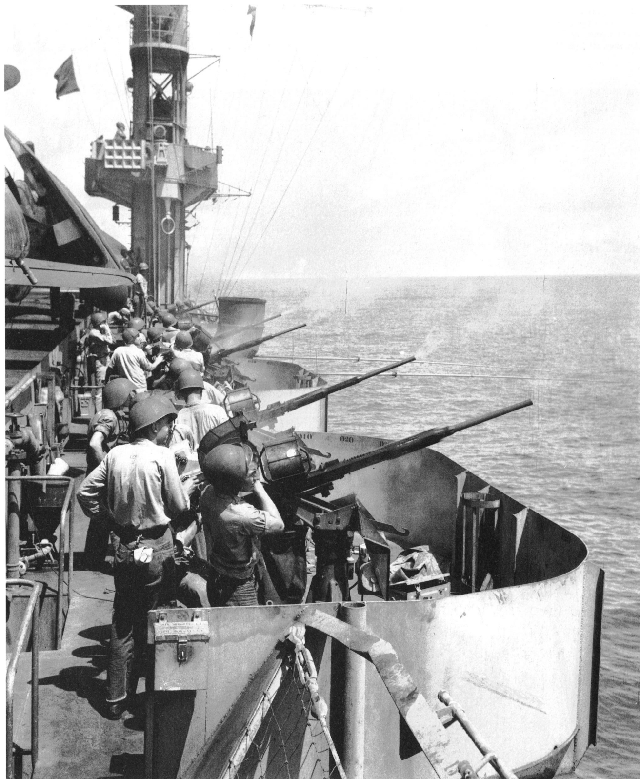
Gambier Bay and her sisters normally carried twenty 20mm Oerlikons in tubs on either side of the gallery deck. (National Archives 80-G-262716)
