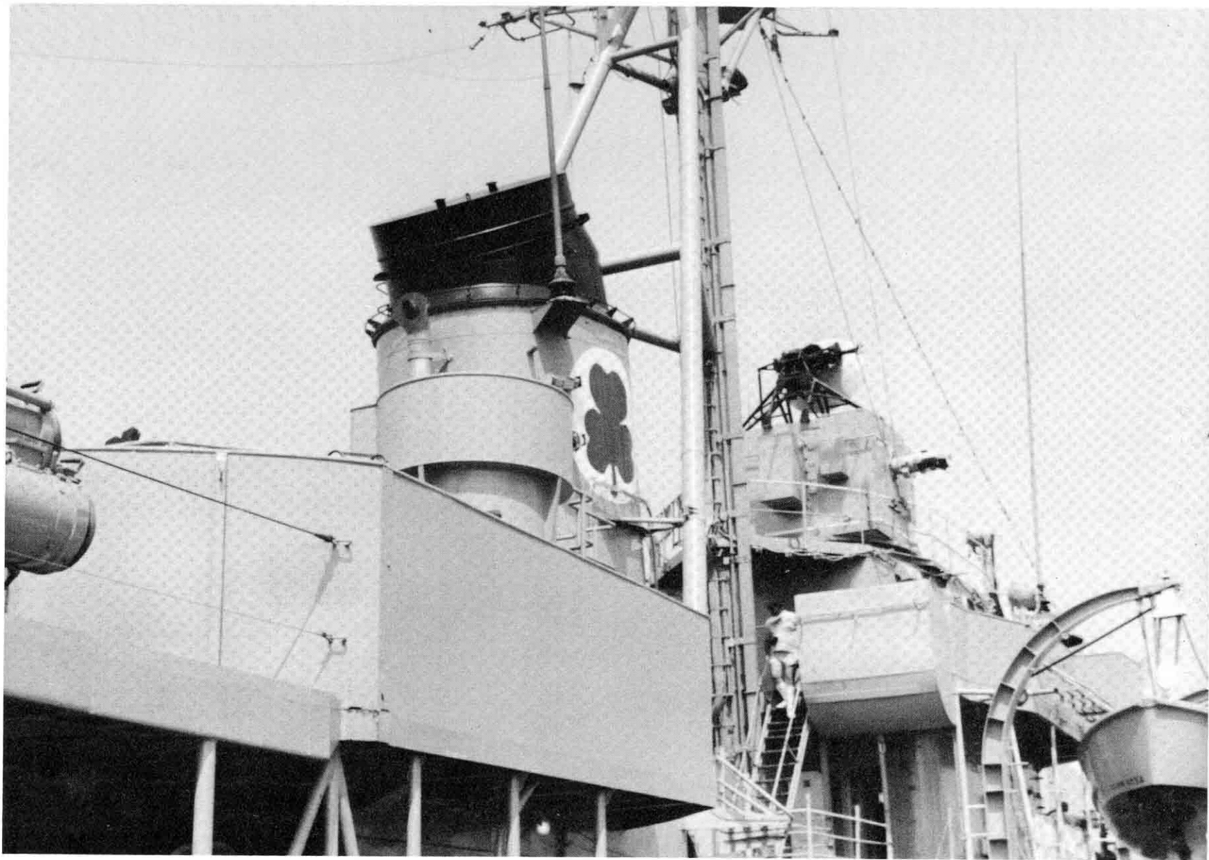
18. Back of the bridge showing tripod mast and forward stack details.
