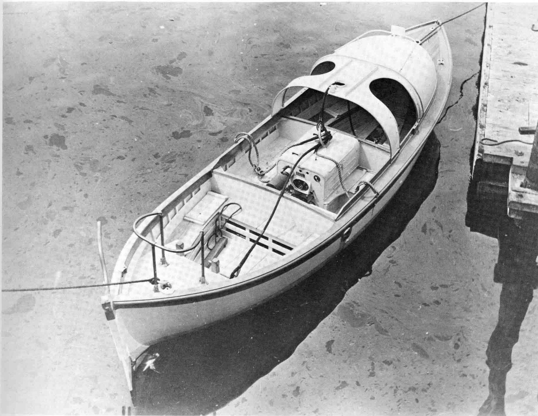
22. The Sullivans carried two 26ft motor whaleboats Mk 1 throughout World War II. This particular boat is an earlier version with a light sheet metal canopy and a more rectangular engine cover, but is essentially the same as The Sullivans' boats.
