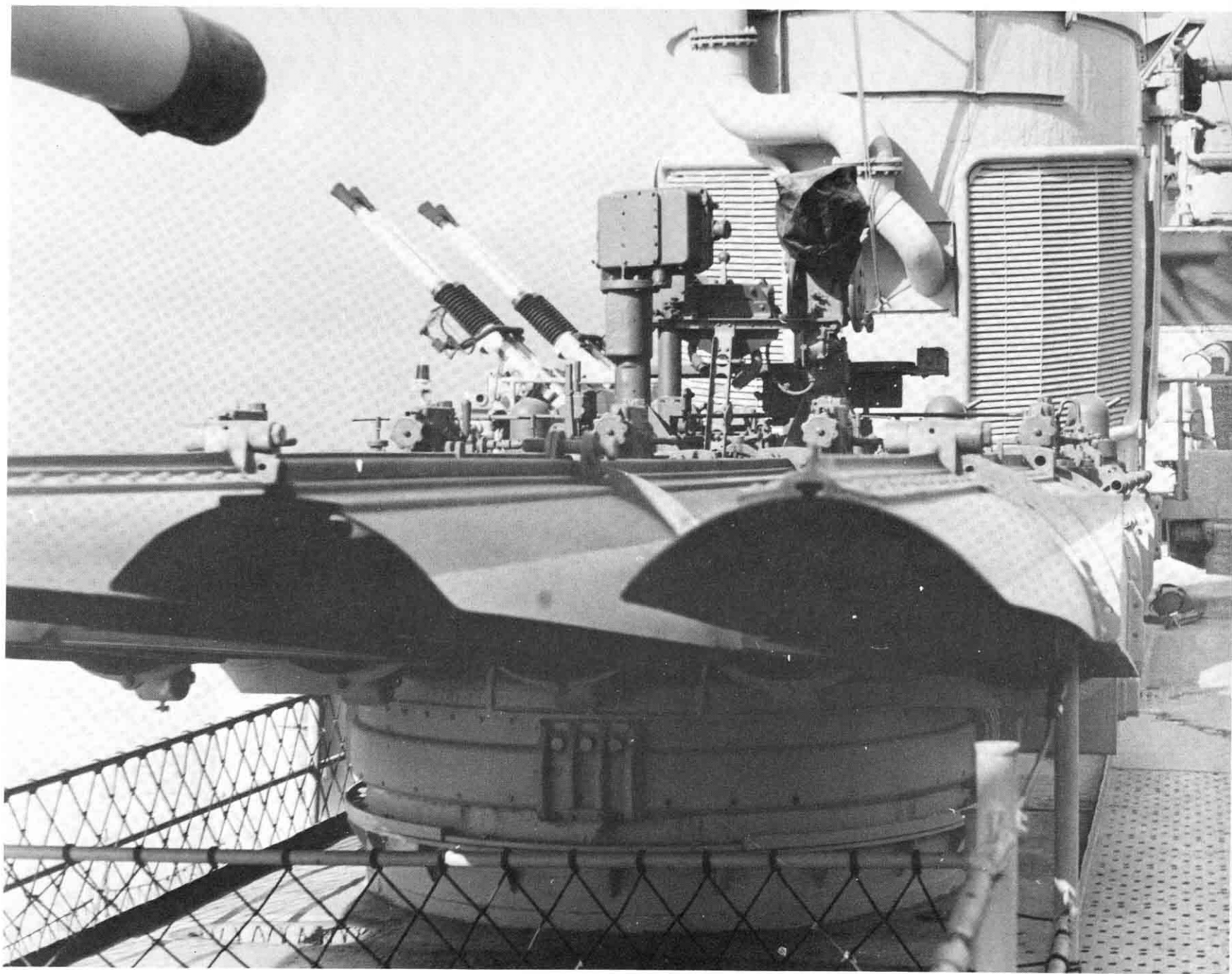
12. An interesting view of the quintuple torpedo tubes. The T-shaped slot visible in the end of the spoon extension is for a guide lug on the torpedo.
