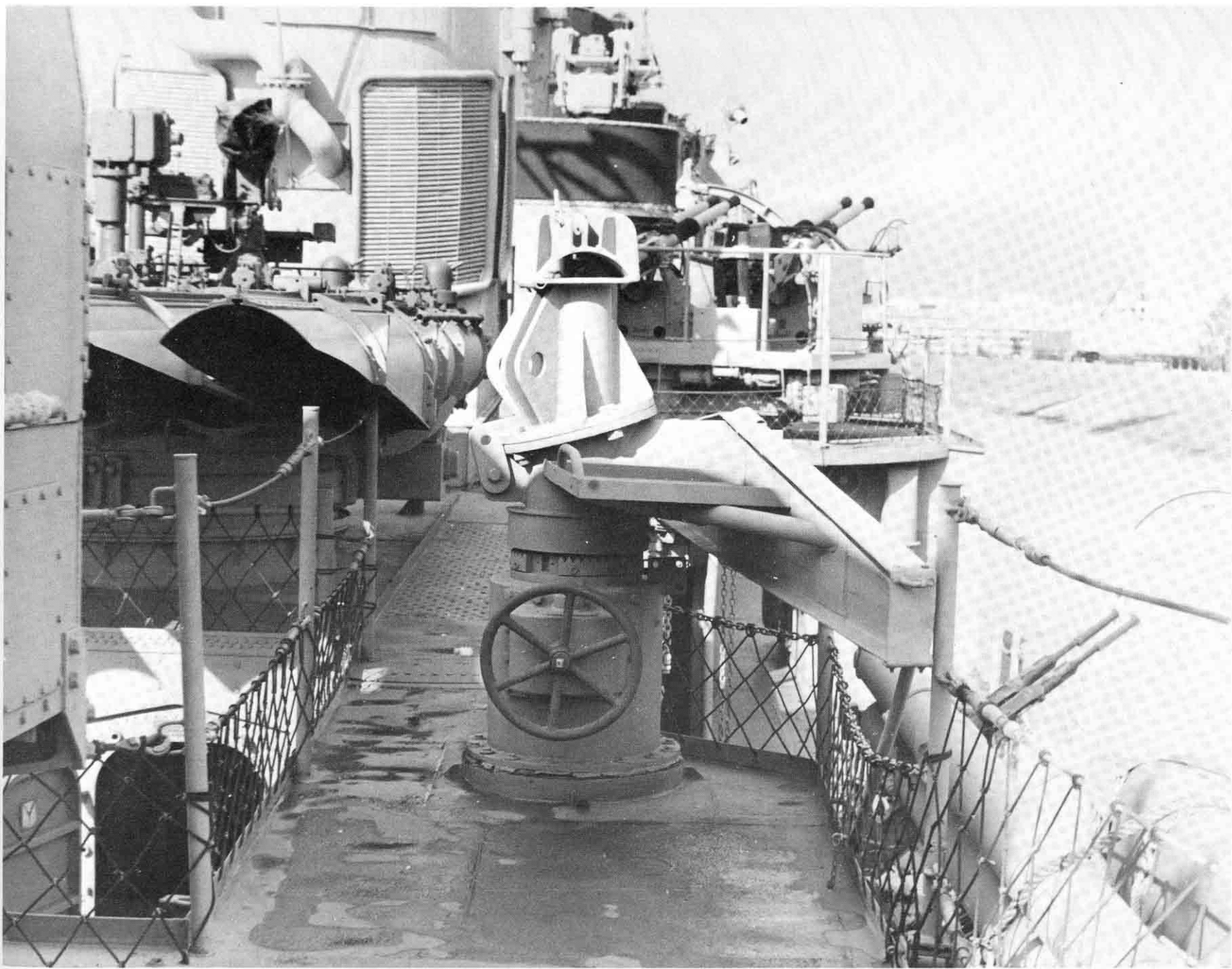
13. Aft torpedo handling crane in lowered position, showing mount for refueling-at-sea gear on top of the pedestal. This particular shot was taken aboard Kidd in 1986, but is identical to the unit carried by The Sullivans .
