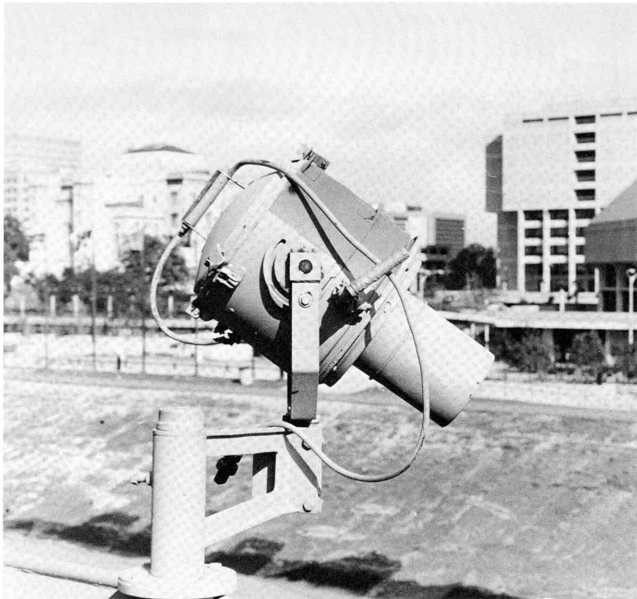
19. Detail view of the 12in signal lamp on the bridge wing.
