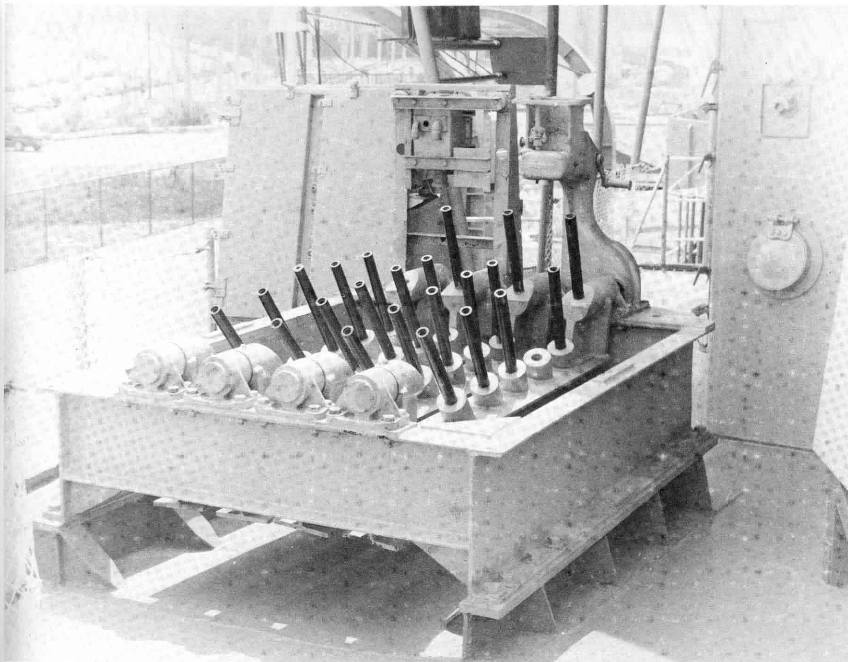
15. Starboard Mk 10 Hedgehog launcher and ready service locker for the 7.2in projectiles onboard The Sullivans , 1987. The circular, hinged cover to the right rear of the launcher is a passing scuttle for the projectiles.
