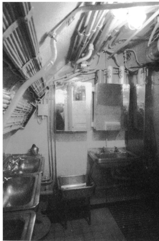
93. A view into the washroom of U-Wilhelm Bauer . On the left are three wash basins, and behind them a foot bath, a further wash basin and above it a water heater. Adjacent on the right is the shower.
