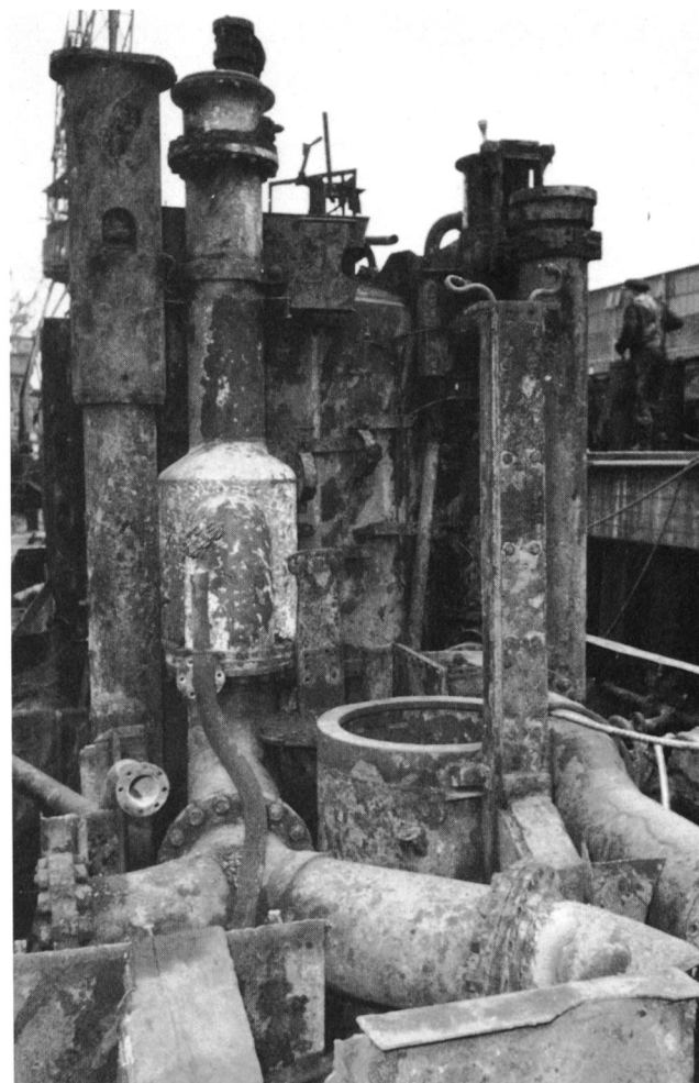
43. U2540 after raising, with the conning tower casing already removed. From left to right are the guide tube for the retractable rod aerial, the air exhaust and the outer schnorkel pipe. In the foreground is the opening for the galley hatch.
