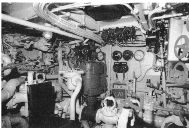
74. A view into the 'pump cellar' of U-Wilhelm Bauer . On the left in the background is the shallow bilge pump, in front of it the filter for fine flooding, the contents gauge for the regulating cells and adjacent on the right the valve for flooding and emptying the regulating cells. On the extreme right is the air inlet distributor for the regulating cells.
