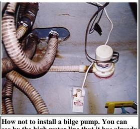
How not to install a blige pump. You can see by the high water line that it has already failed. The hoses at left were restraining the float switch and the wire connections were laying in the bilge water. They were moved prior to taking this photo. The builder installed it this way.
