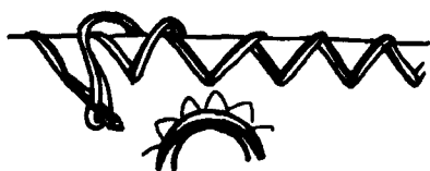
B. A last-ditch alternative, cross stitching a corner or edge of a sail where it's chafing.
