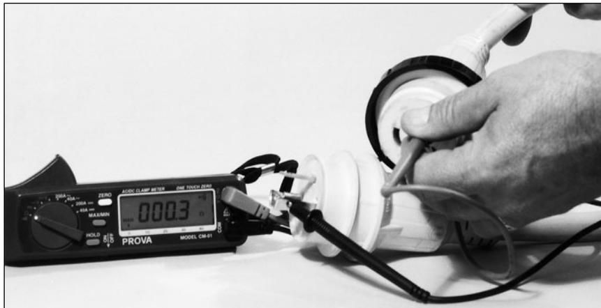
Fig. 11-14. The “wiggle test” on a shore-power cord.
