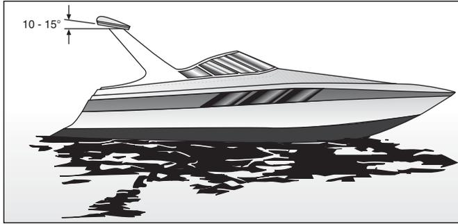
Fig. 12-15. Static angle for powerboat radar antenna installation.
