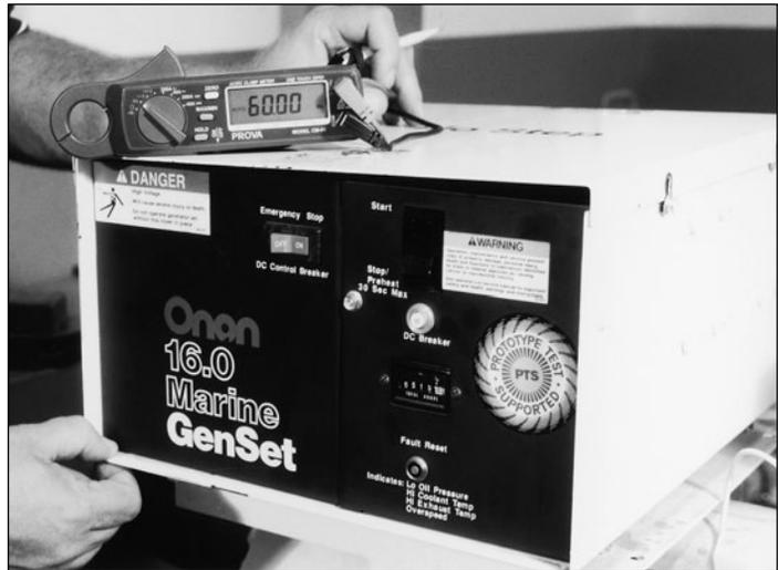
Fig. 11-22. Checking frequency with the multimeter.
