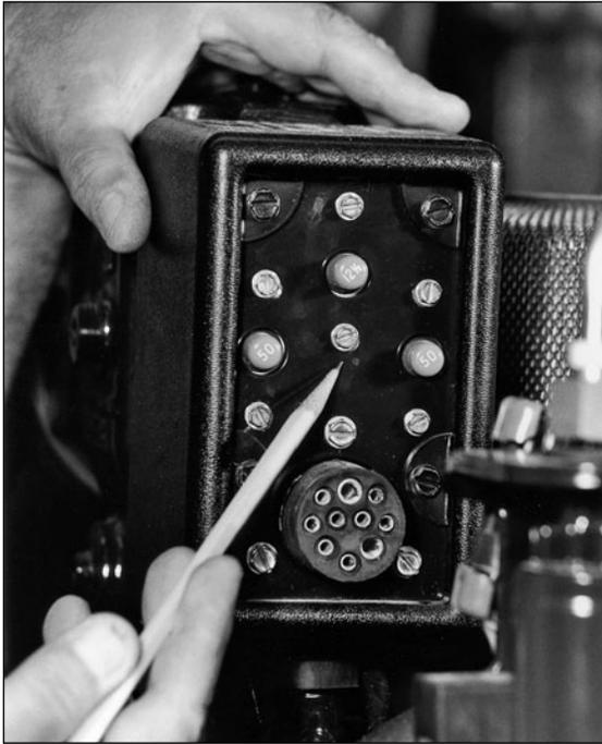
Fig. 6-6. Engine-mounted circuit breaker.
