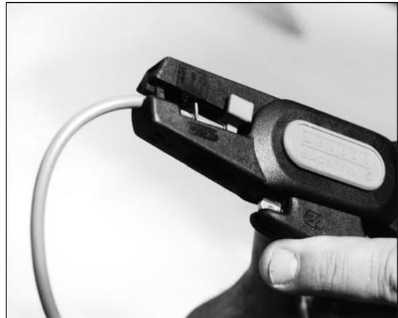
Fig. 4-26. End stripper in use.
