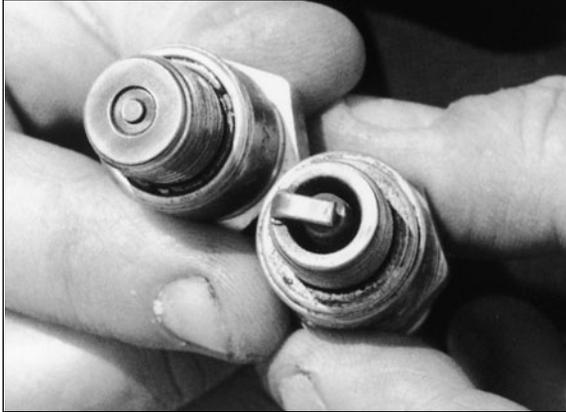
Fig. 7-11a. Surface gap and traditional spark plugs.
