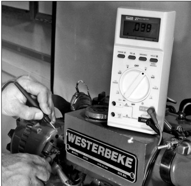
*Fig. 6-10. AC ripple-voltage test. Your black meter lead should be connected to a known good ground and the red lead to the B+ (output) lead on the back of your alternator. Remember to make sure that your meter is set to the AC volt scale.*
