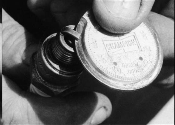
Fig. 7-11b. A spark-plug gapping tool.
