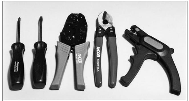
Fig. 9-6. Electrical tools needed for a bilge-pump installation.
