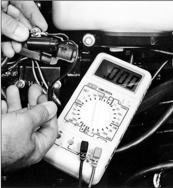
*Fig. 7-21. Mercury tilt switch. This switch is designed to prevent engine starting with the prop out of the water. If it malfunctions (open-circuits), your engine won't start with the prop in the water, either! In this picture I've removed the switch and am testing its function with a multimeter set to check continuity when the switch is tilted manually. I'm verifying with the meter that the switch turns off and on.*
