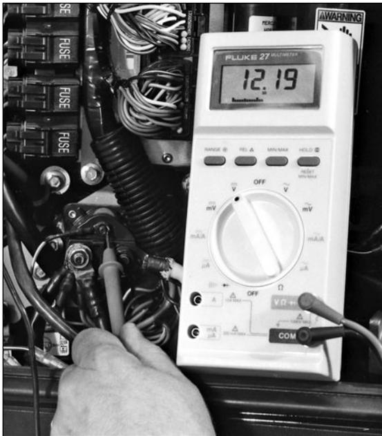
Fig. 8-9a. Checking voltage supply to an outboard-engine solenoid with the key in the start position. Remember, with the key in the start position, if the engine is cranking, the voltage reading will drop down to as little as about 9.6 volts.
