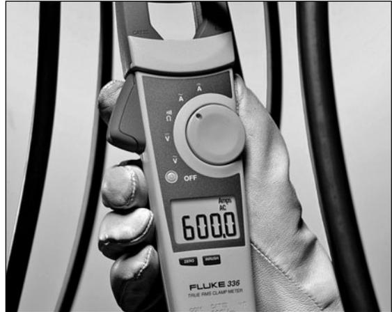
Fig. 3-3. Fluke Model 336 clamp-type meter. This is a true RMS (root-mean-square) meter that can read up to 600 AC or DC amps. This is an excellent choice if you do a lot of AC work. Its shortcoming is that its ohms scale is not as sensitive as other meters I've used. This model sells for about \$275.
