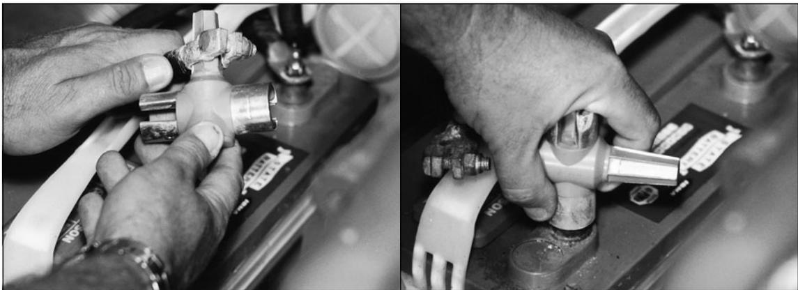
*Figs. 5-6, 5-7. Steps to cleaning the battery post and clamp, using a battery service brush. Use these tools until you see shiny surfaces on both the post and inside the clamp. Figure 5-6 shows the terminal being cleaned; figure 5-7 shows the battery post being cleaned.*
