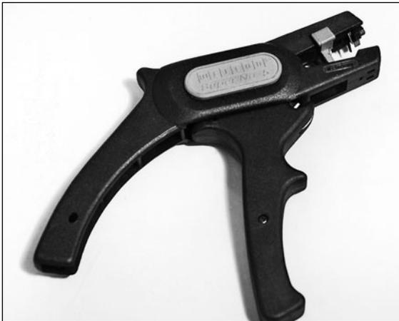
Fig. 4-25. End stripper. I love these tools because you can adjust the amount of insulation to remove for a really good match to the crimp connector. One drawback is that they only work on wire up to 10 AWG.
