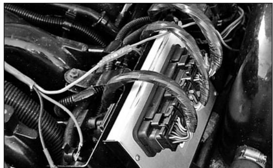
Fig. 10-10b. Engine-mounted computer.
