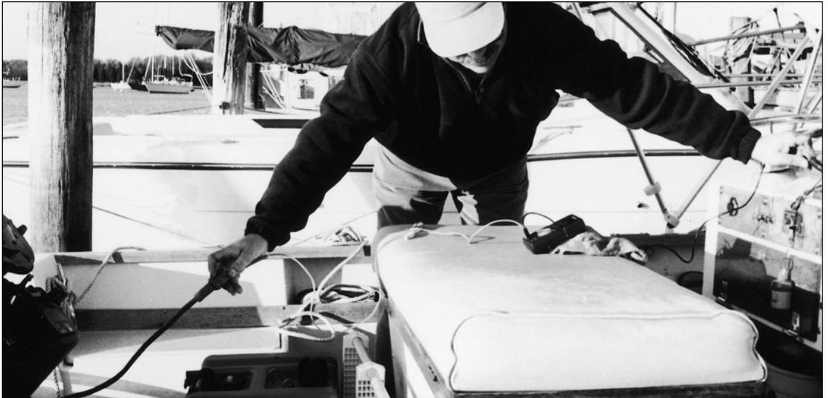
*Fig. 8-8. Checking the wiring harness for continuity between the remote control and the engine. In this picture I've disconnected the plug at the back of the ignition switch and at the engine, and am using my ohmmeter to check for breaks in the wiring harness.*
