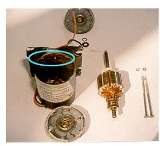
Dismantled view of motor. The circled area denotes area of heavy corrosion that was inhibiting the motor rotation. Once cleaned up, the motor ran freely.
