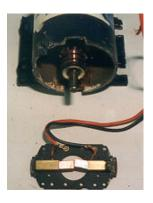
Having gotten the motor apart, we want to see what the problem is. In this case, water got in and caused corrosion. Whether or not the the motor can be repaired is going to depend on how badly it's corroded. The armature is the large rotating part in the center with all the copper windings around it. If this is very
