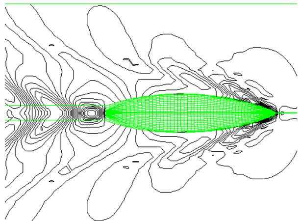
FIGURE 14: Wave contours from a non-linear potential flow calculation for an IACC yacht
