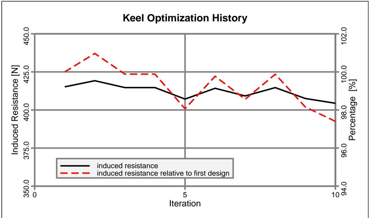
FIGURE 12: Optimization history for the induced resistance of a keel-bulb-winglet configuration
