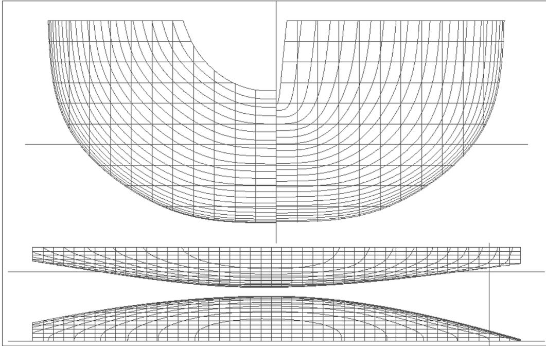
FIGURE 4: IACC canoe body designed by parametric modeling
