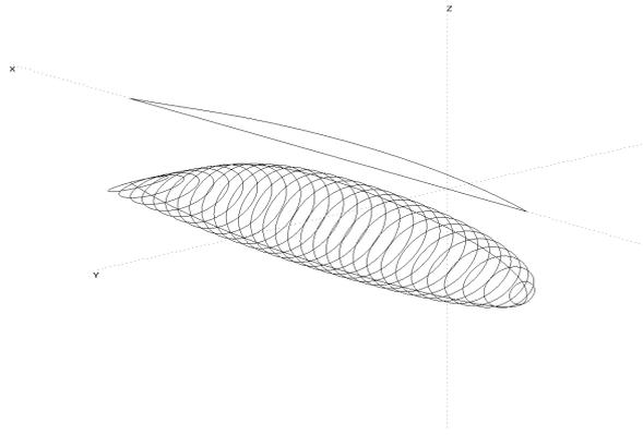
FIGURE 7: IACC keel bulb with natural vertical centroid (neutral centroid modifier)
