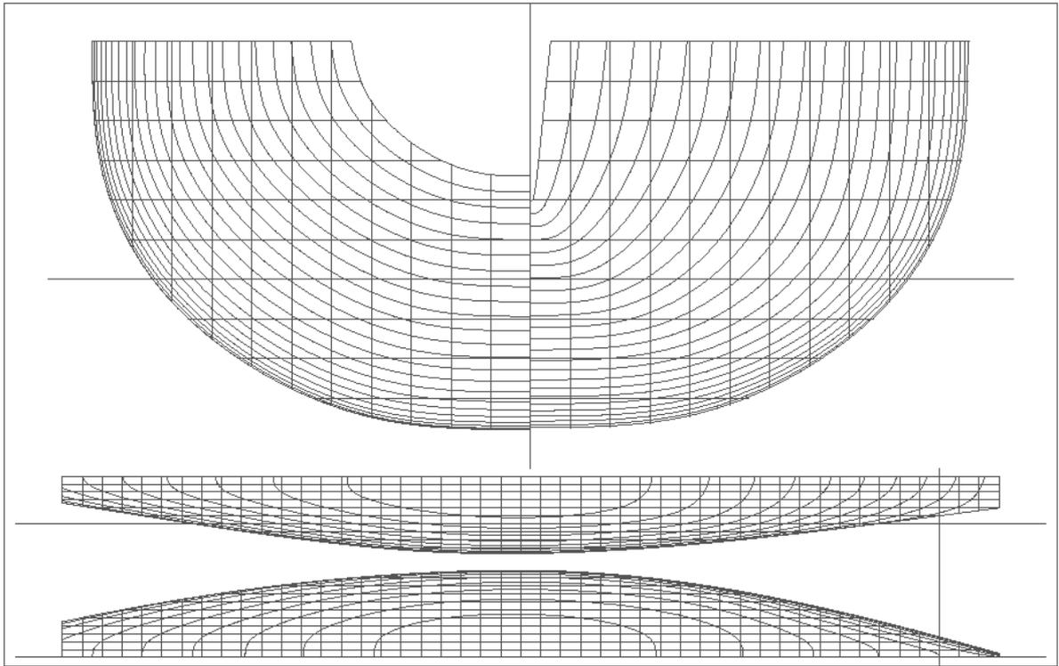
FIGURE 2: Parametrically designed IACC yacht with circular sections
