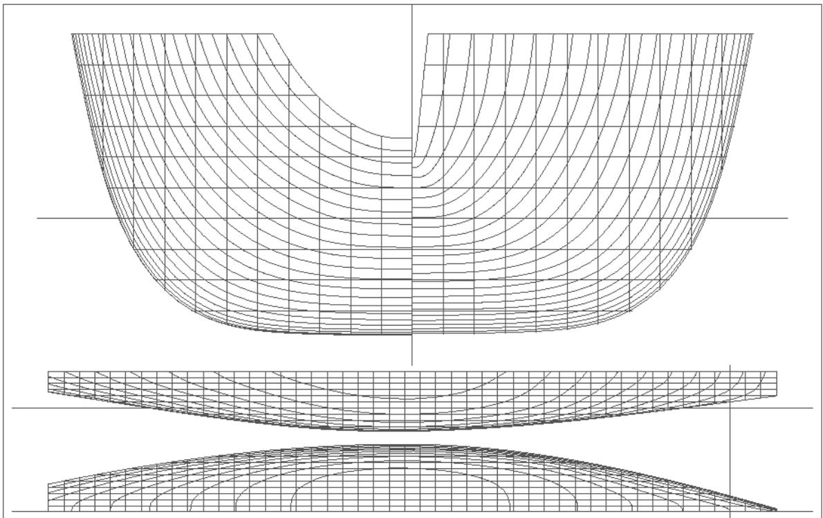
FIGURE 3: Parametrically designed IACC yacht with trapezoidal sections
