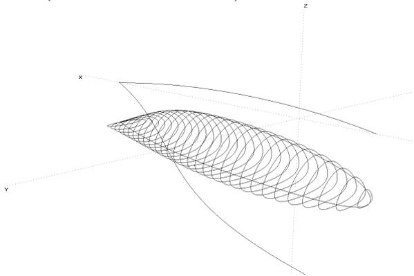
FIGURE 8: IACC keel bulb with modified centroid – low to neutral
