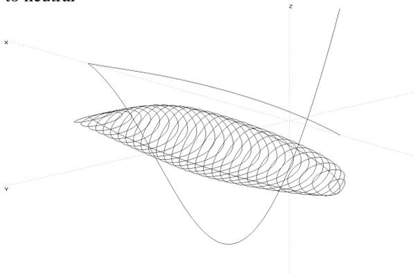
FIGURE 9: IACC keel bulb with modified centroid – high via low to neutral
