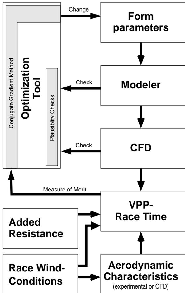
FIGURE 16: Complete optimization process for racing yachts
