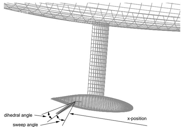
FIGURE 11: Keel-bulb-winglet configuration used for analysis of induced drag (neglecting keel flap)
