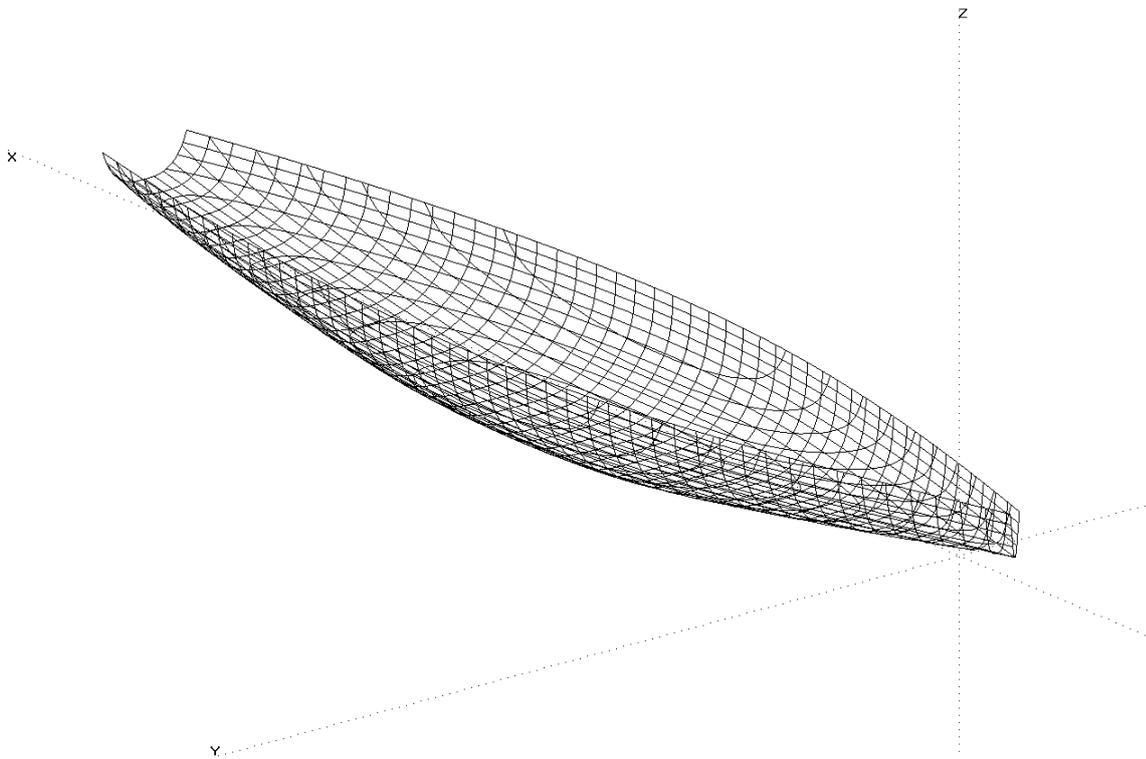
FIGURE 5: Perspective view of an IACC canoe body designed by parametric modeling
