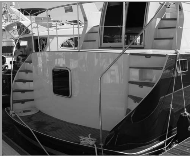
Transoms can be customized to suit the owner's needs. Boarding from the dinghy was a major concern for the owner of this Voyager 495, which we overcame with transom steps.
