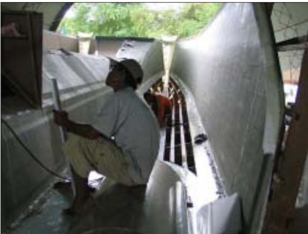
TOP: This view shows the panels which have the core material laminated to the inner surface now in place in the mold former.
