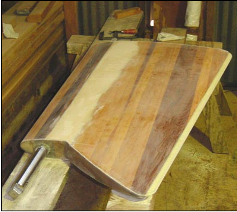
The rudder timbers are laminated around pre-prepared stainless steel webs that are welded to the rudder shaft.
