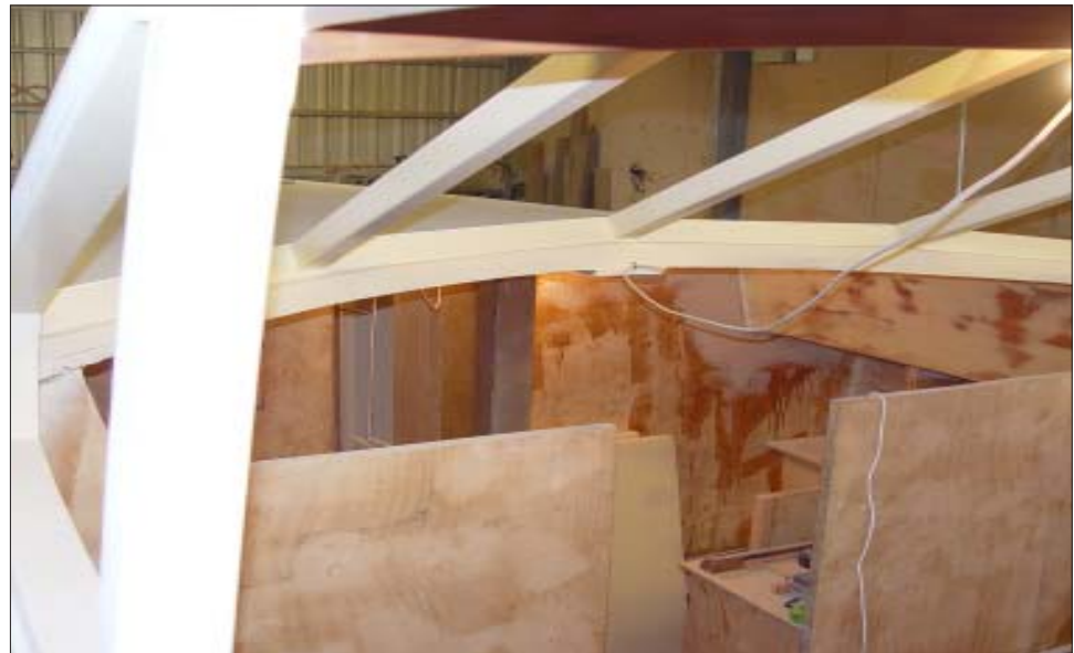
Here is another view of the pilot house, bulwark and trunk cabin. Note the fine finish that has been achieved by Graham Andrew in building and finishing this Roberts 370 strip plank hull.
