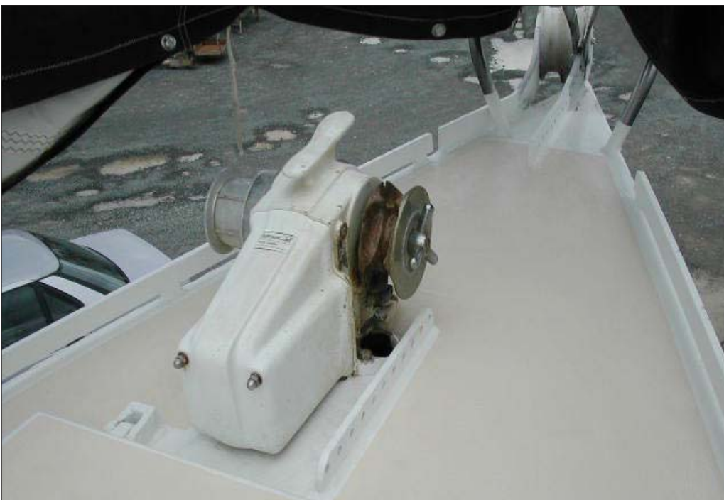
LEFT: Functional anchor winch that will handle both anchor chain and rope
