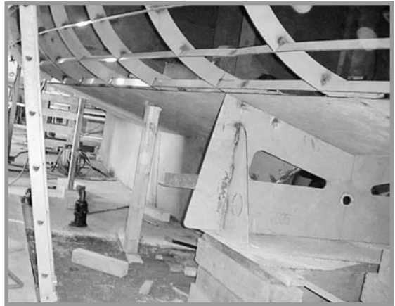
Another view of one of the setting-up jigs that supports the bottom plates.
