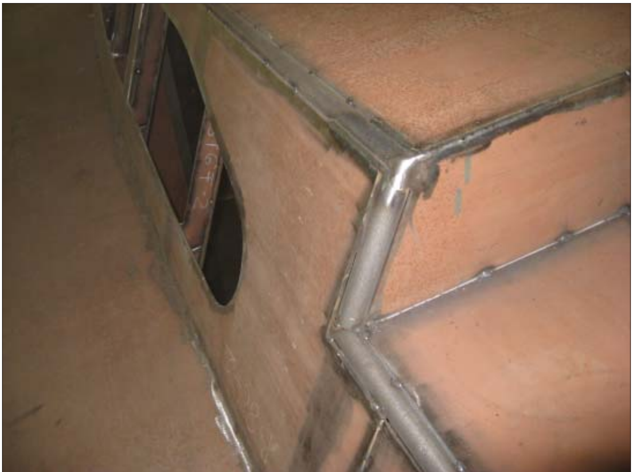
BELOW: Close up of rounded corners where deck salon sides meet top on the Voyager DS 440.
