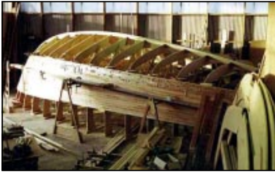
Modern strip plank hulls are planked with the hull inverted.
