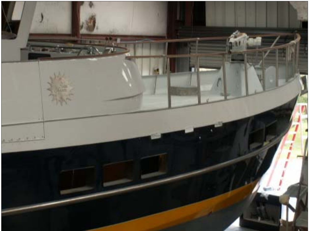
This Spray 52 built by Gil Davenport clearly illustrates both adequate bulwarks and life rails that are designed to keep you safely on board under all conditions.
