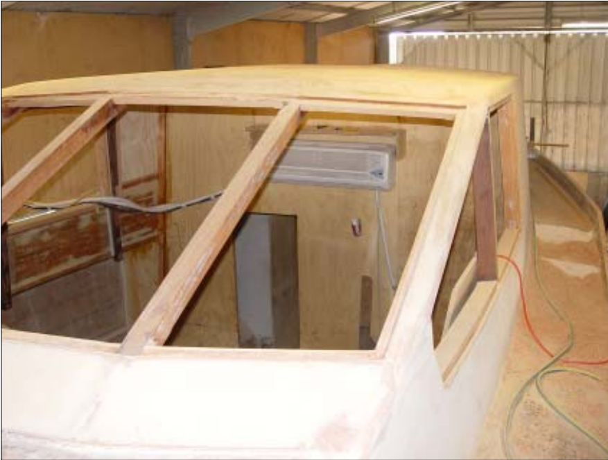
Here is a close up of the pilot house framing. Note the areas in the mullions and the area surrounding the window aperture that have been rabbeted ready to receive either armour plate glass or high quality Perspex or Lucite glazing.
