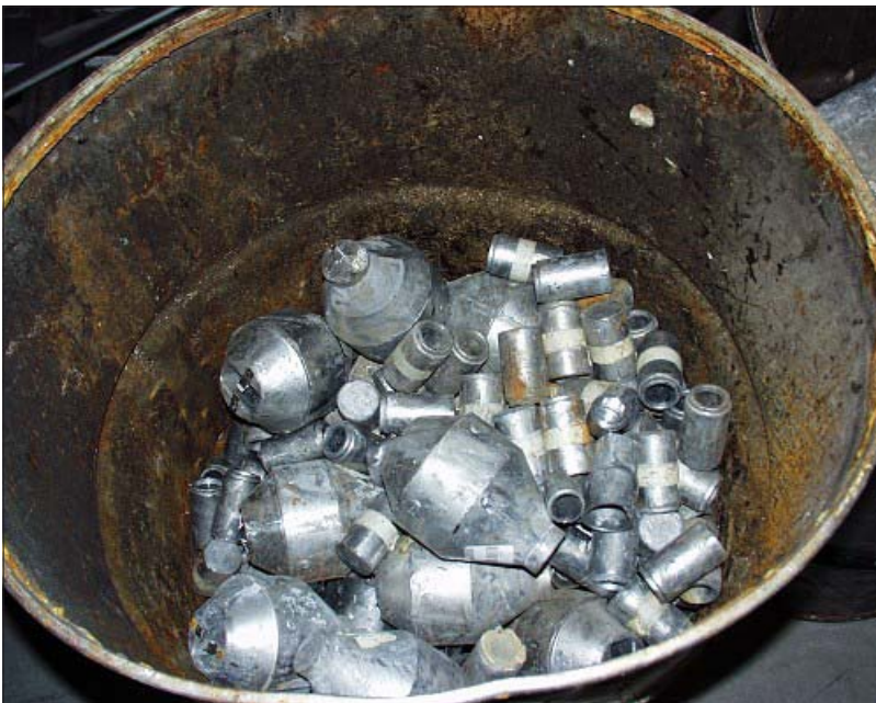
LEFT: Here is some lead scrap that will be melted down to form the cement between the larger pieces of ballast.
