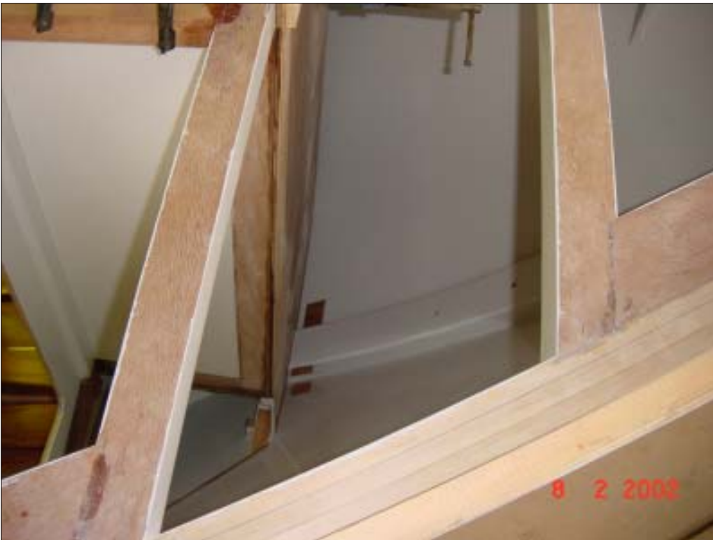
Close up on the deck beams.
