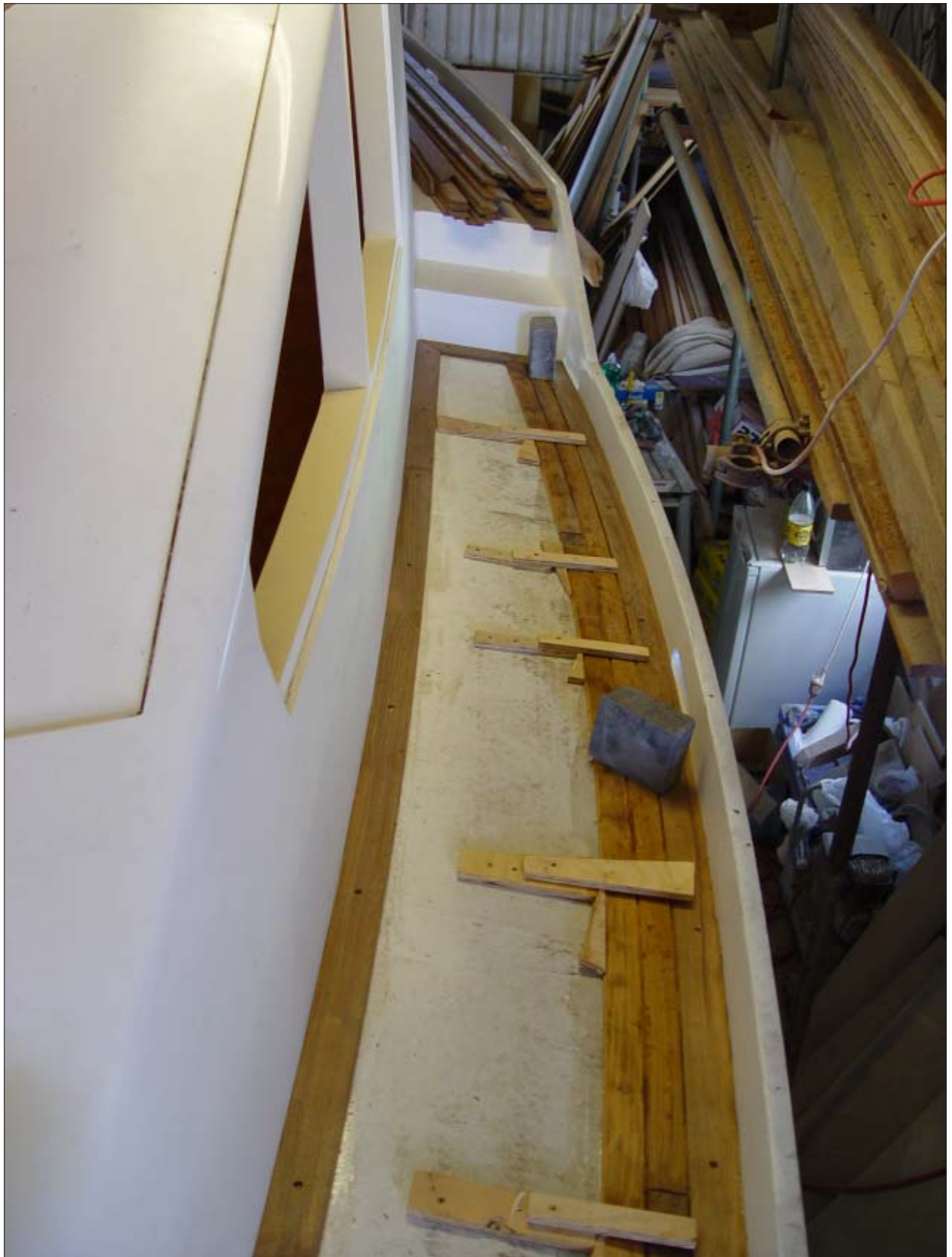
This photograph shows the side deck planking proceeding at a steady pace. Graham Andrew worked over the weekend to take these shots and allow us to see most of the deck planking in place.
