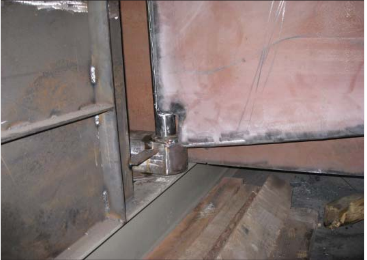
ABOVE & BELOW: Two views of the rudder tube and shaft where it exits the hull (top) and sits on the bearing in the heel (bottom) ; note that the top of the tube should be above the static waterline
