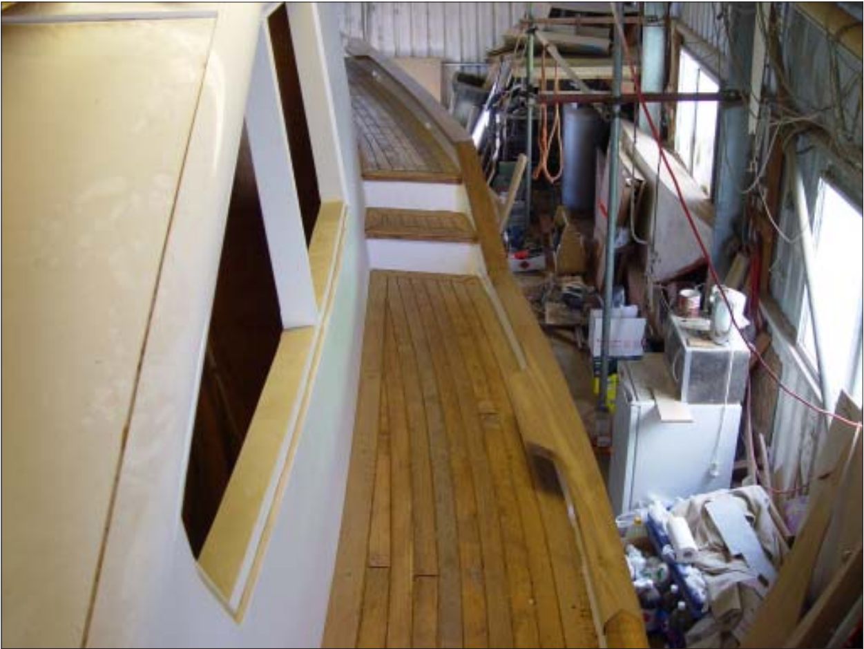
Here we see the completed side and cabin top laid decking - All that is left is to add the caulking.
