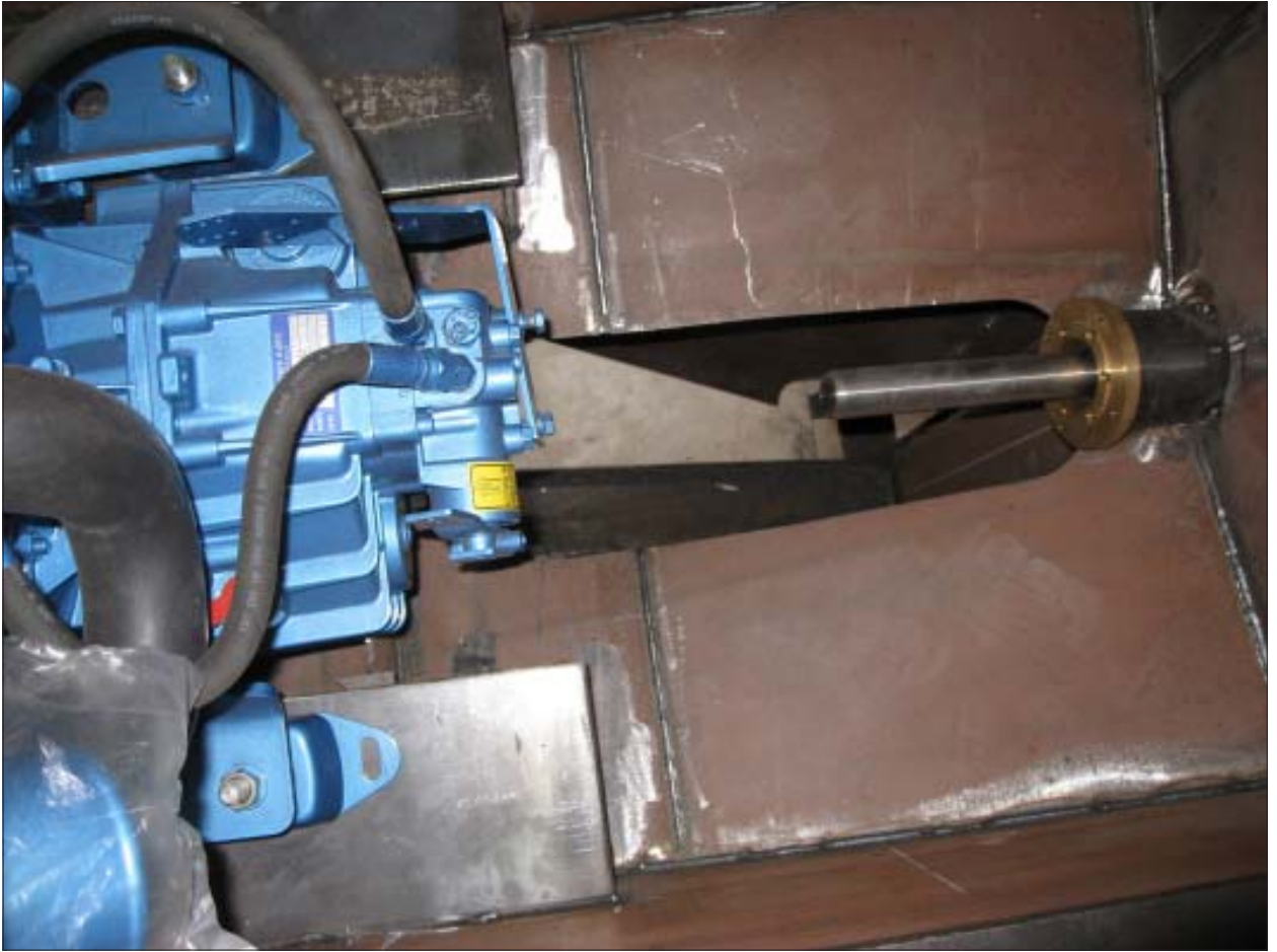
ABOVE & BELOW: Two views of the prop shaft and where it exits the hull via the aft end of the keel. Always study the plans that come with your cutting files or kit.
