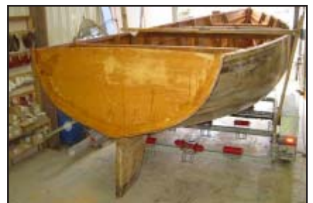
Here we see the process of building a Wood / Epoxy Roberts 25 hull
