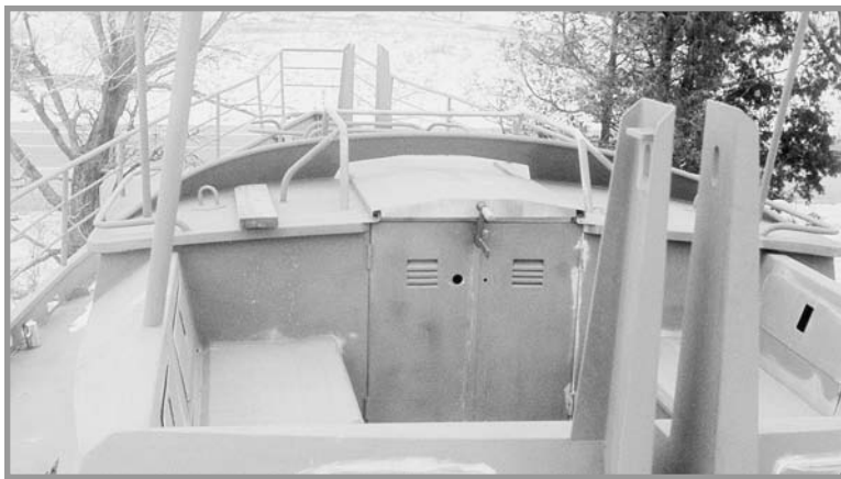
The sturdy tabernacle on this Roberts 53 is in keeping with the rest of this beautifully built boat. It's built to go anywhere.
