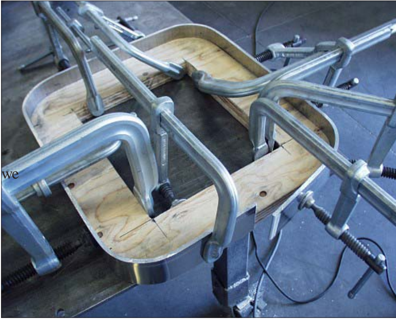
LEFT: Here we see pilot house window frames being constructed
