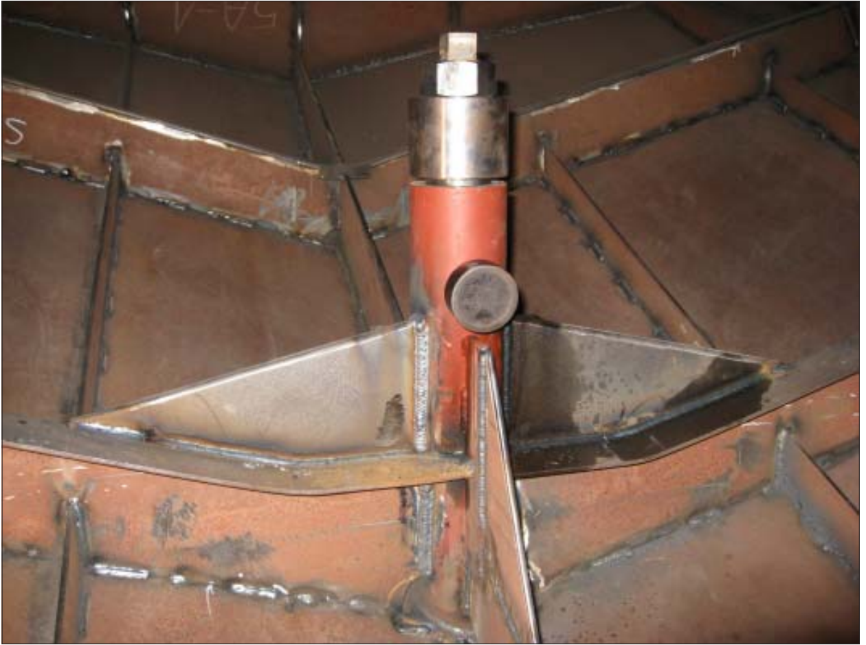
ABOVE & BELOW: Two views of the rudder tube and shaft where it exits the hull (top) and sits on the bearing in the heel (bottom) ; note that the top of the tube should be above the static waterline
