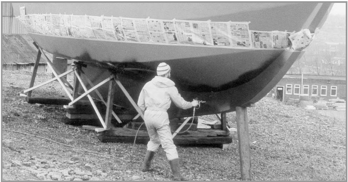
Careful masking of the various parts of the boat will play an important part in ending up with a professional-looking paint job.
