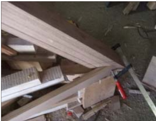
Above we see Graham taking off the frame shapes from the full size patterns and getting started on setting up the hull framework.
