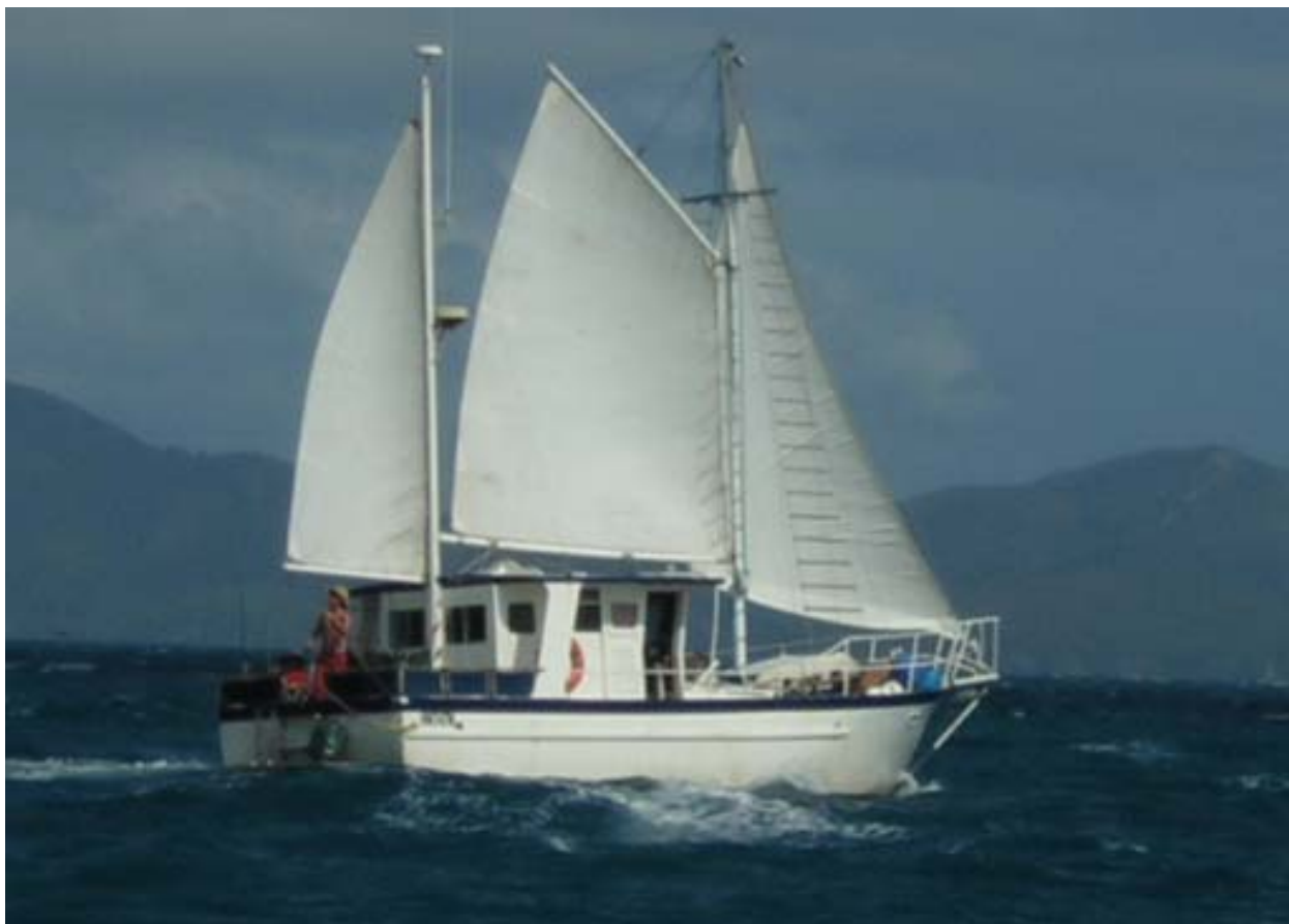
ABOVE: Not all motor sailers are this obvious, the 'Pacific Coast Fisherman 40' as its name suggests is based on a displacement fishing boat hull. One recently 'sailed' from Australia to Ireland.
