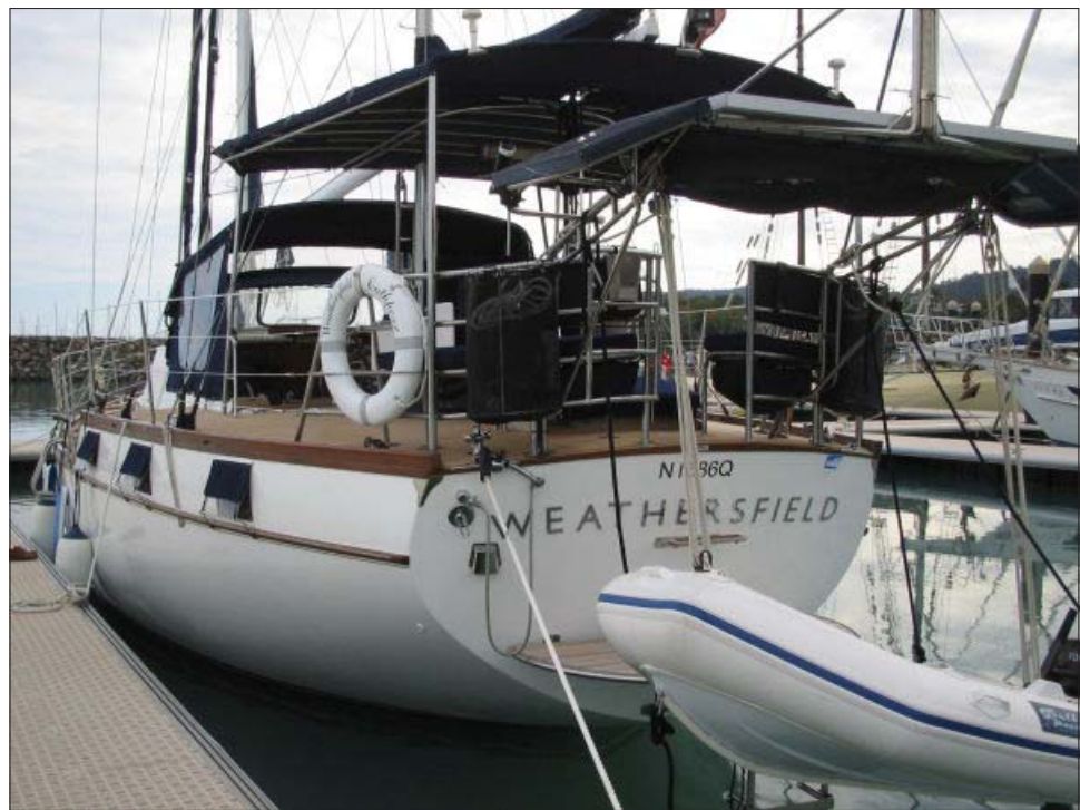
RIGHT: Some builders have installed a traditional transom on their Roberts 58's; this does add extra deck room and interior space but you lose the boarding & swim platform & also be careful of the additional weight aft
