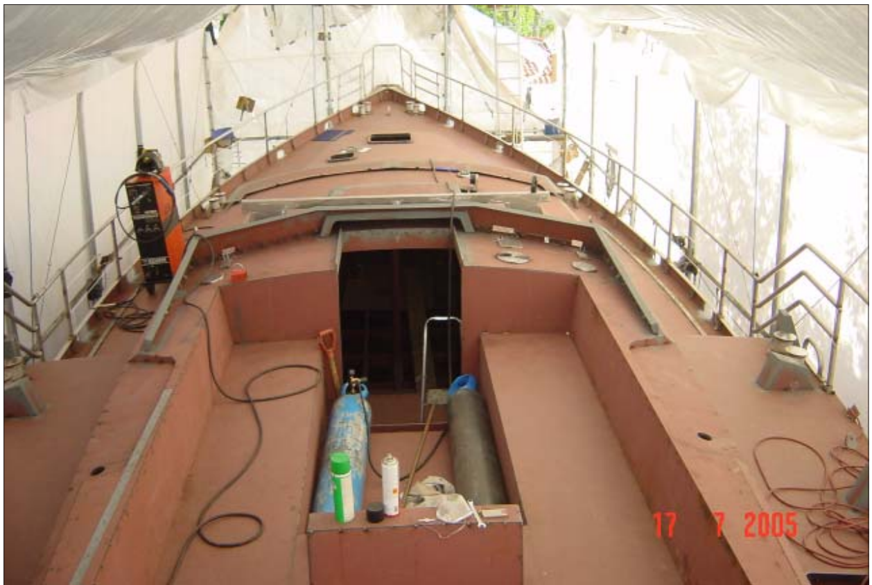
ABOVE: In these photos you can see the fairing built over and just ahead of the companionway to accept the windscreen and bimini that may be added to give extra protection to those in the cockpit; these features are very popular in Europe where this Voyager 542 was constructed from our kit.
