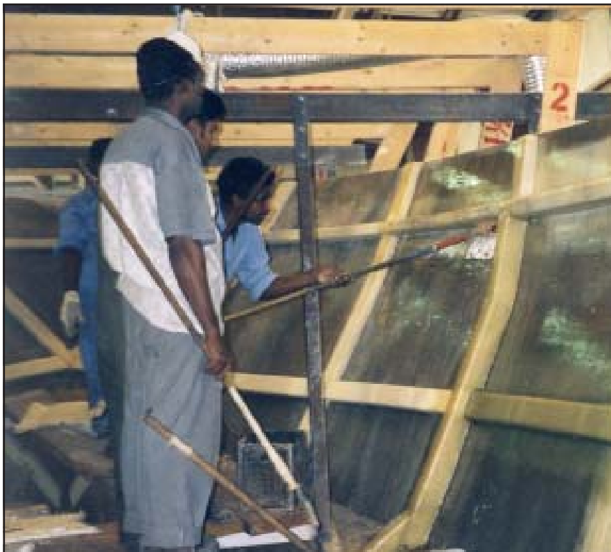
Here we can see the foam core for stringers and ribs being installed in a fibreglass hull..
