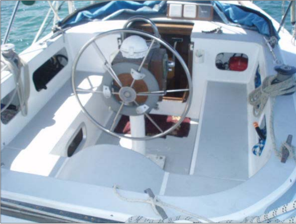
LEFT: Note the spacious cockpit is a feature of the flush deck Roberts 35
