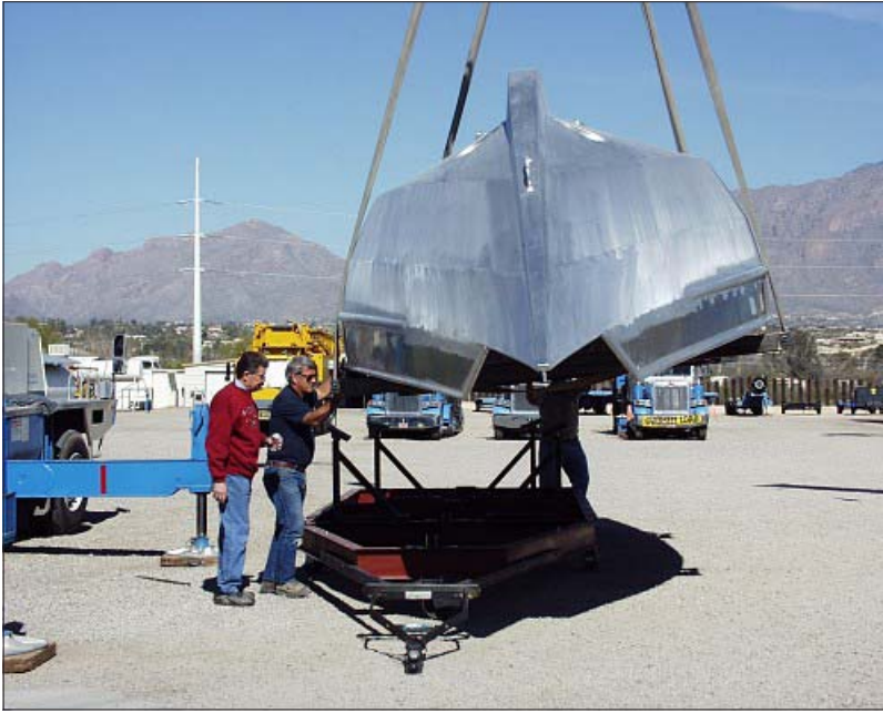
LEFT: Preparation of the turn over operation; the boat is suspended in two endless slings.
