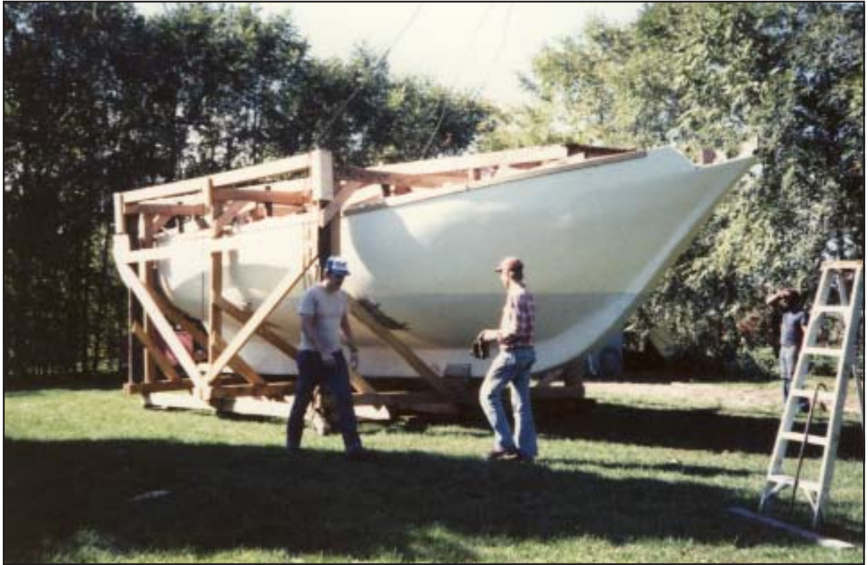
Adam and Barbara Szczurowski photo of their Spray 36 fibreglass hull. If you are building a Bruce Roberts designed boat then your plans will show this type of turning over cradle. This arrangement has worked for all types of sailboat, powerboat and even catamaran hulls.
