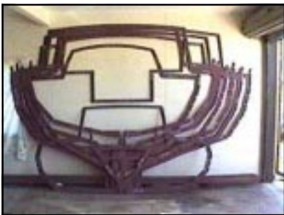
The frames have been tacked together ready to be erected once keel and hull bottom plate have been laid.
