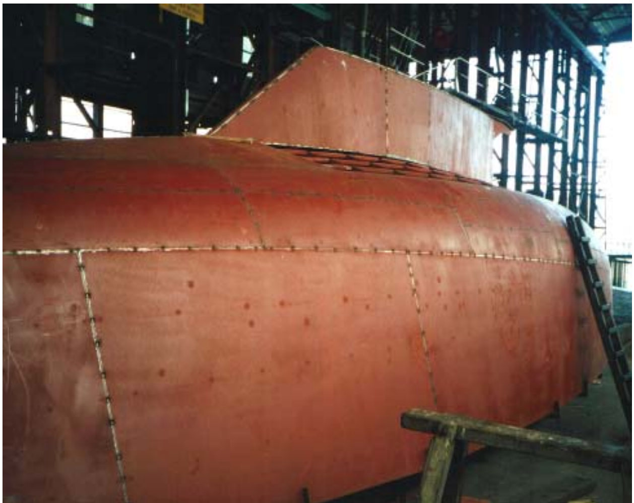
ABOVE: Roberts 432 radius chine hull. Note all TACKED together before full welds are run.
