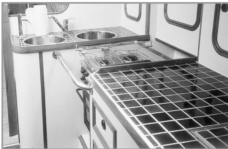
A rail protects and steadies the cook in front of this stove.
