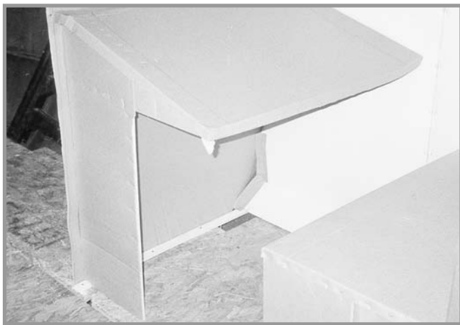
One builder used inexpensive cardboard to mock up his joinery; if you want to try out a piece of furniture, this looks like a great idea.
