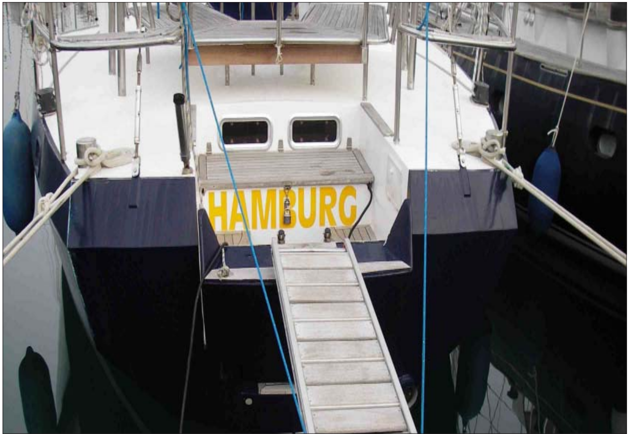
ABOVE and BELOW: The fold down section of the transom combined with a boarding plank makes a nice arrangement especially if you are cruising in Europe where stern to mooring is commonplace.
