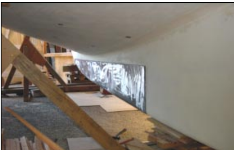
External cast lead ballast bolted in position.
