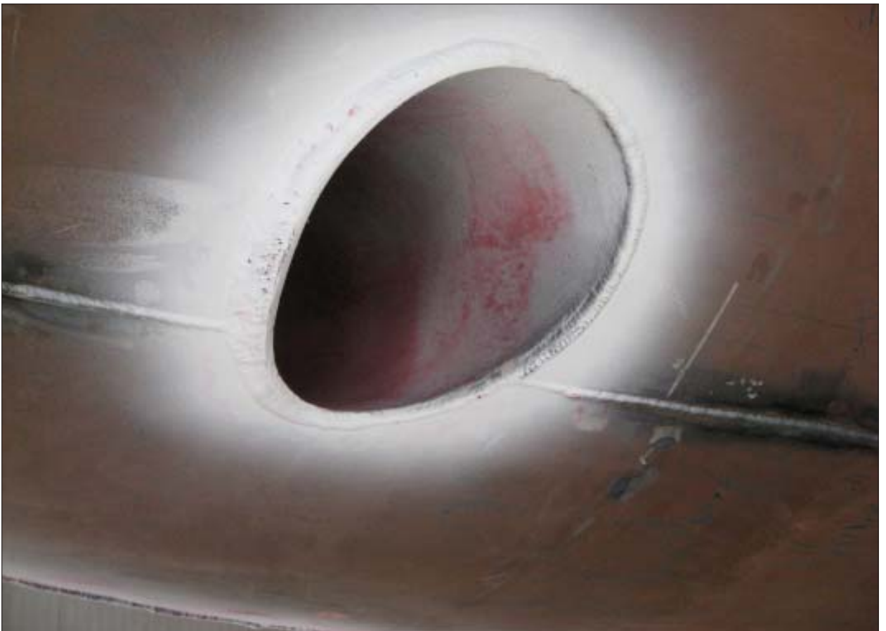
ABOVE & BELOW: Two views of the bow thruster tube; note the touch up of the primer to prevent rust getting a foot-hold on the welded areas of your hull. Welds will be ground above the waterline but unground below the waterline.
