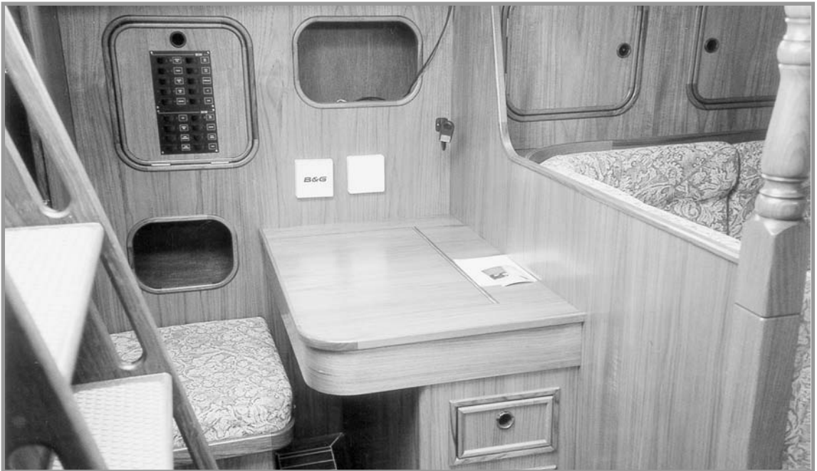
Note the comfortable forward-facing navigation station tucked out of the traffic in the walk-through on this Roberts 434. A selection of repeater instruments was added to this area.
