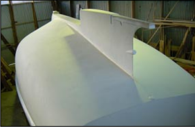
Final fairing completed the hull is now ready for turn-over. Photograph by permission of Rob McGill and Nina Morissette
