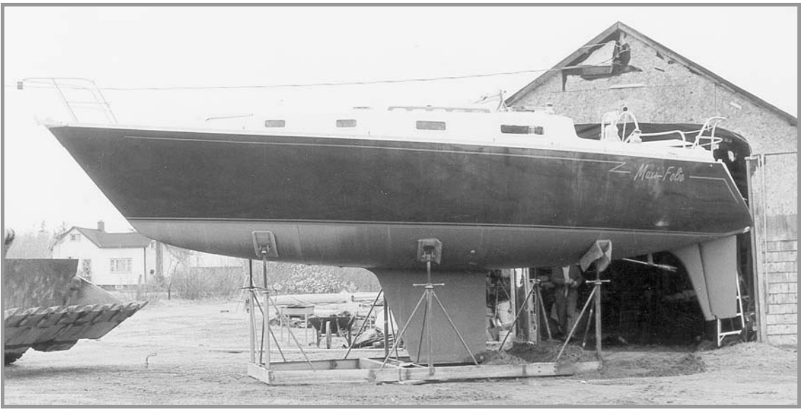
This Roberts 342, built in Europe, is a fine example of what you can achieve using the radius-chine technique to build in either steel or aluminum.
