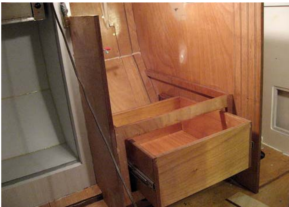
LEFT: Make sure that all drawers have strong runners and also have a means of preventing them from coming open in a seaway.
