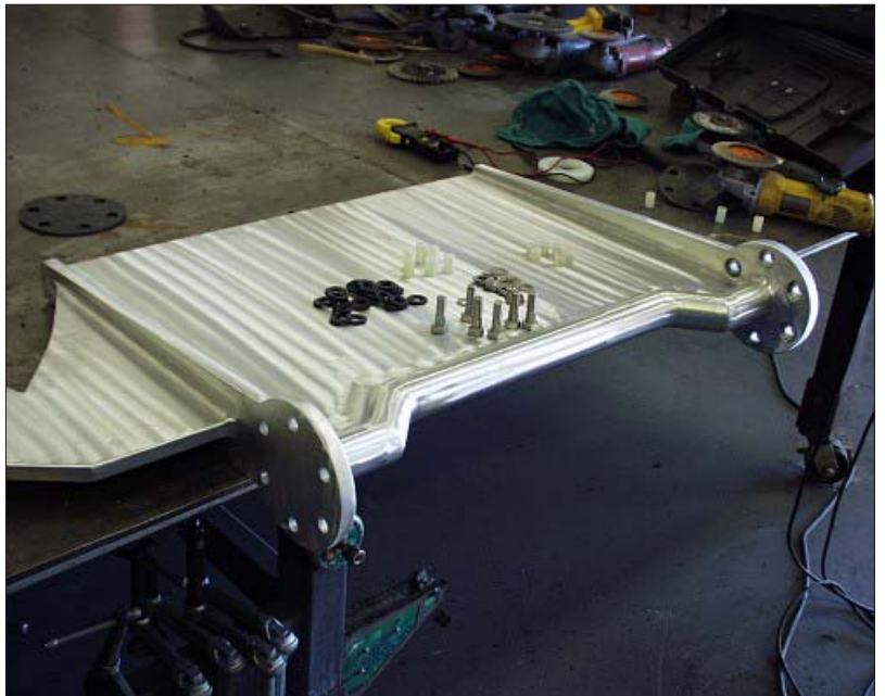
RIGHT: Here we see the rudder complete with the flanges used to connect it to the rudder shaft and to the stub shaft into the heel.
