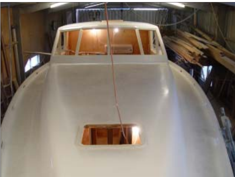
Next the strip plank was covered with two layers of fibreglass cloth set in epoxy and sanded to a fine finish. A little 'elbow grease' or as much as is needed can pay handsome dividends as will be seen in the fine finish shown in this photograph.
