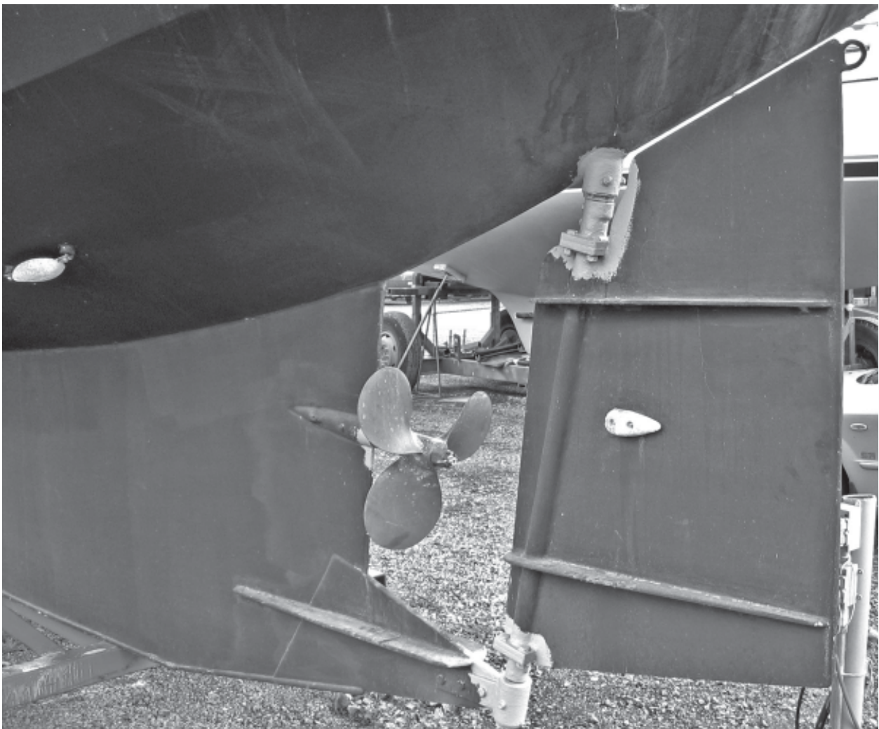
ABOVE: This type of rudder is a BAD idea on a sailboat. You should build your rudder so it is airfoil shaped in section; this rudder could be greatly improved by plating each side of the webs.
