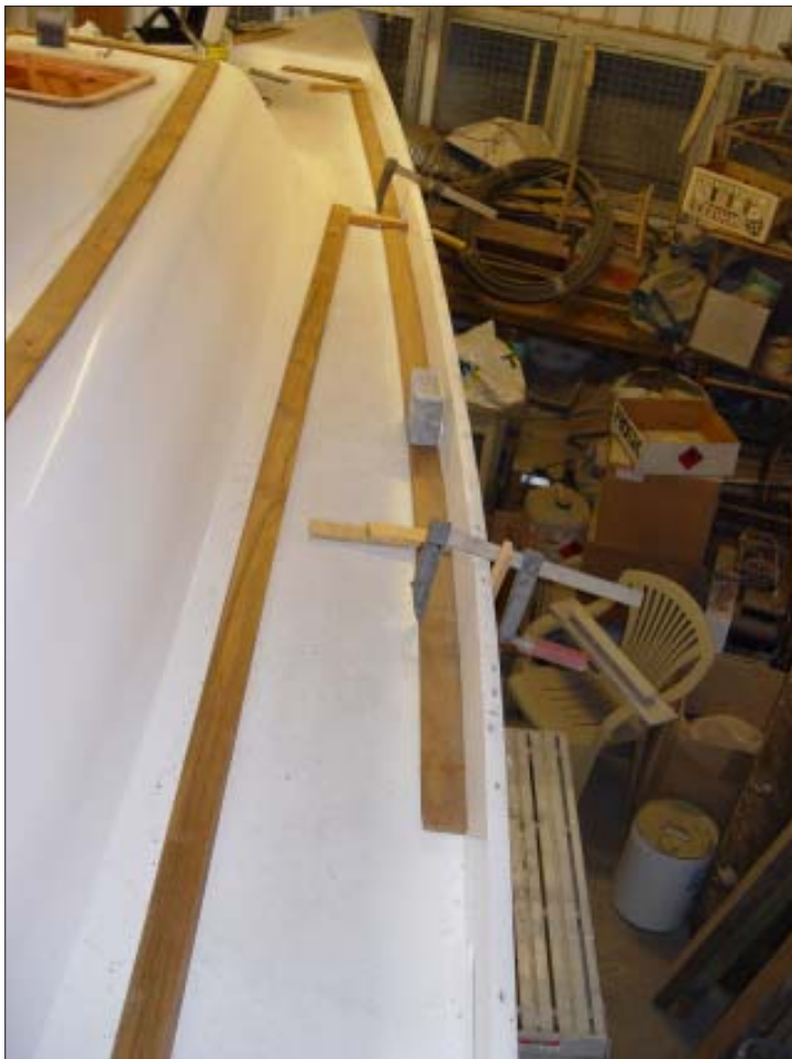
Graham is beginning to install the teak deck. The margin planks are the first to be installed all round the perimeter of the decks and cabin top
