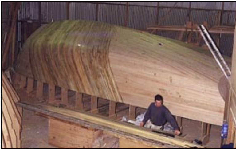
Many times your plans will call for either strip plank, double diagonal planking or a combination of the two as is shown here.
