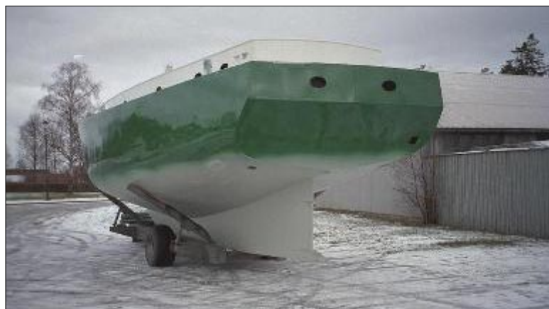
Centennial Spray 38 stern view - note heel and propeller tube - makes for clean water flow and efficient powering.
