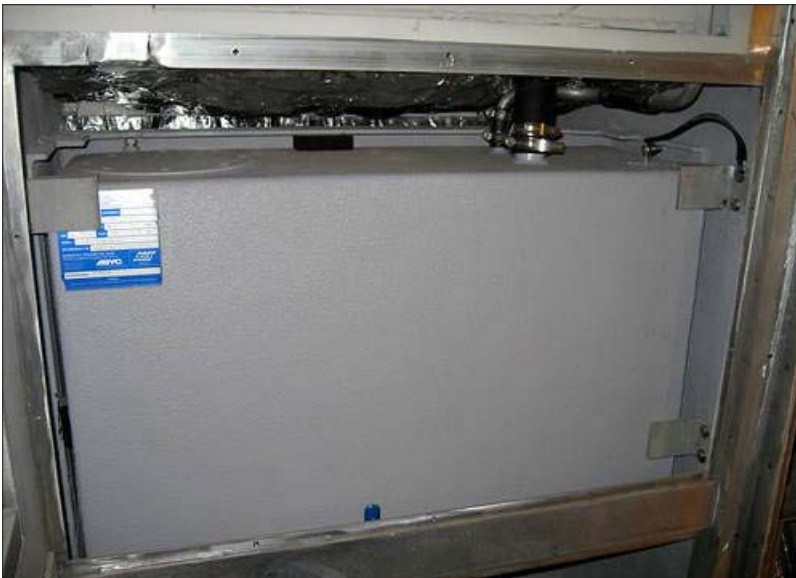
LEFT: Tank snugly in place, make sure that all tanks are firmly and strongly attached to the hull as a tank breaking loose in a sea-way is a disaster !
