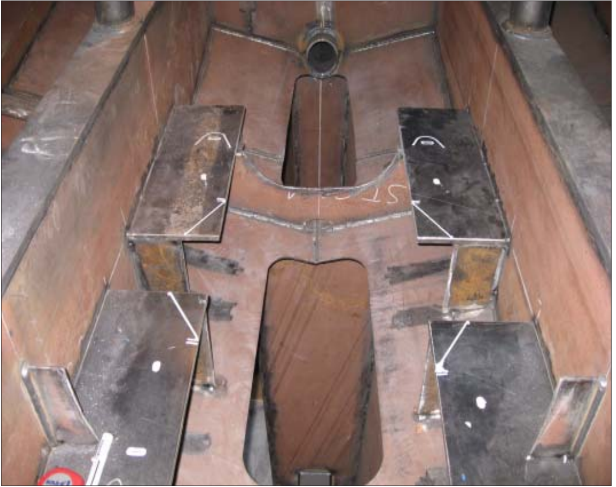
ABOVE & BELOW: Two views of the engine beds which are included in the kit and cutting files but can be modified if required to suit your particular engine.
