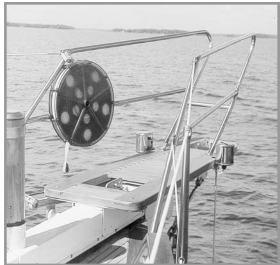
This arrangement combines a bowsprit, a sturdy pulpit, a jib boom, and an anchor-line reel for the second an-
