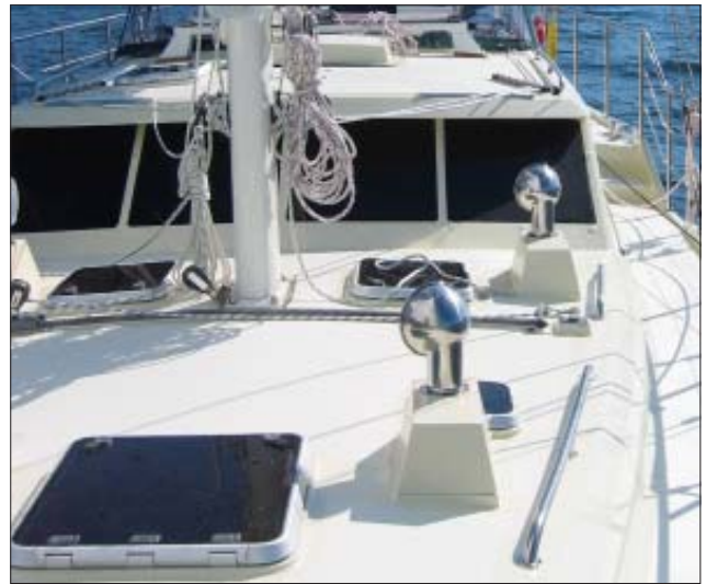
Hatch is correctly hinged on forward side on the fore-cabin of this Voyager 542
