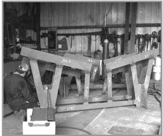
Most kits come with three or four setting-up jigs as part of the cut-steel package.
