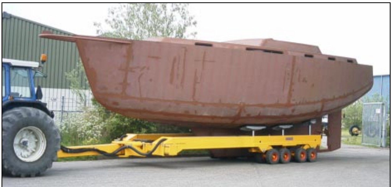
This Voyager 432 was assembled in Holland from one of our pre-cut kits. Here we see the finished hull being towed to the joinery shop on a low loader. Remember you need access to your building site to move your completed hull.
