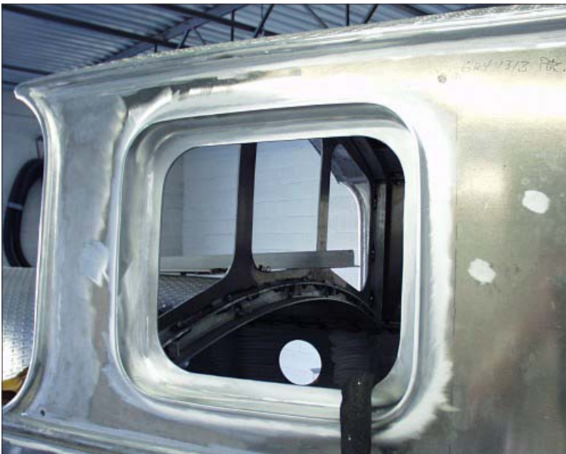
LEFT: The first of the window frames is now installed in the pilot house side.
