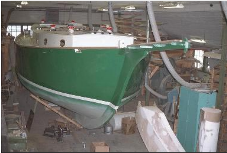
The round bilge steel Centennial Spray 38 shown here was built in Sweden.
