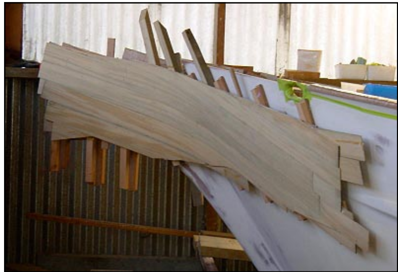
Laminated timber in place to form the shape of the trail boards.
