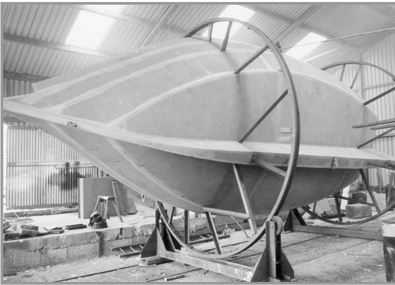
Many builders have fabricated various turning-over devices. These sophisticated turning wheels are ideal if you're building more than one boat.
