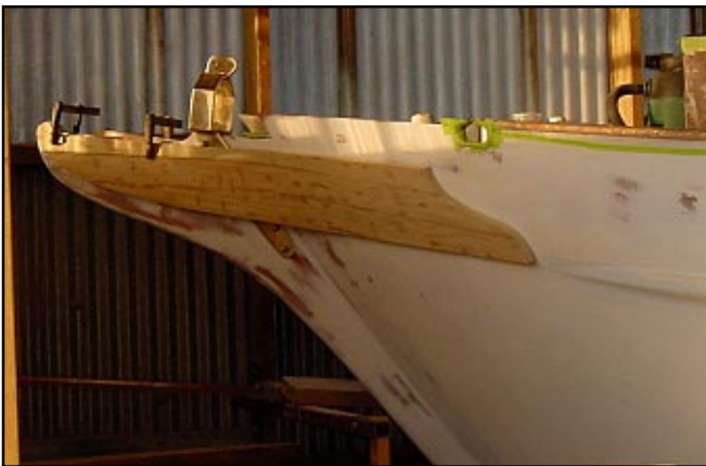
Trail boards marked to shape and trial fit for final trimming to shape
