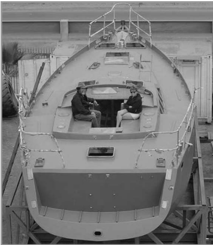
This Voyager 495 was cut in Chile using cutting files and assembled with the aid of the comprehensive plans that accompanied the files by owner/builder Bernie Loyer.
