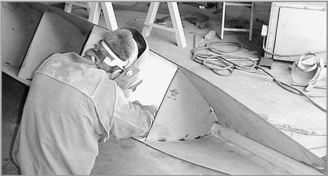
Keels are assembled either in place or separately, as shown here; your plans will advise you of the best method to use.
