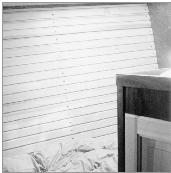
Ceiling (timber planking) is a popular way to line the interior of the boat. Correctly installed, this material will allow air to circulate behind the planking and help keep the boat free of condensation.
