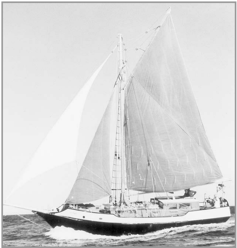
Note the rigging arrangement used on the cutter Spray of Del Quay, a steel Spray 40.
