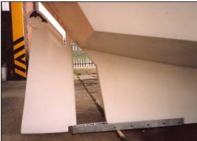
This photo illustrates a typical rudder and supporting heel. The heel can be steel or steel or timber encased in a heavy fibreglass laminate, about the same weight of glass is used on the bottom of the keel. Note the nice touch by way of the fancy fish on the top of the rudder.
