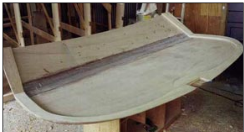
The transom is often fabricated off the hull and added before or after turn-over, check your plans for details.
