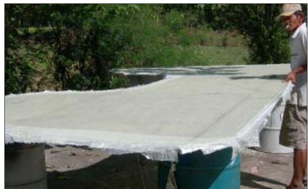
TOP: This view shows the panels which have the core material laminated to the inner surface now in place in the mold former.
