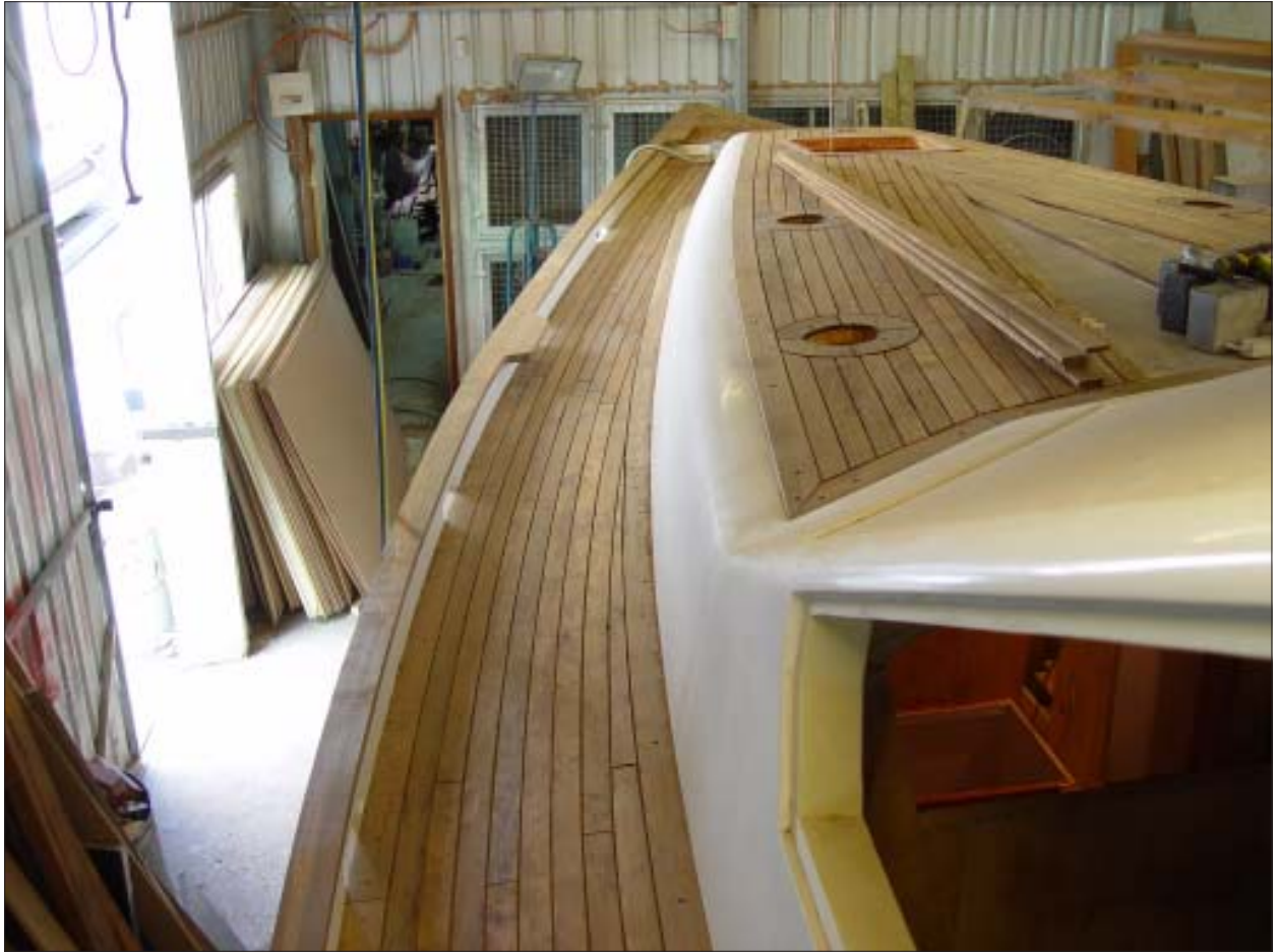
This section has the caulking material applied - Later all will be sanded to give the desired finish.
