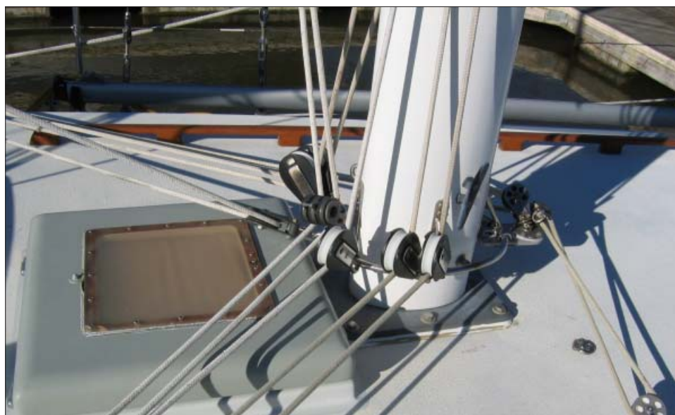
LEFT: Leading the halyards and some sheets aft to the cockpit make for easier handling especially during inclement weather.
