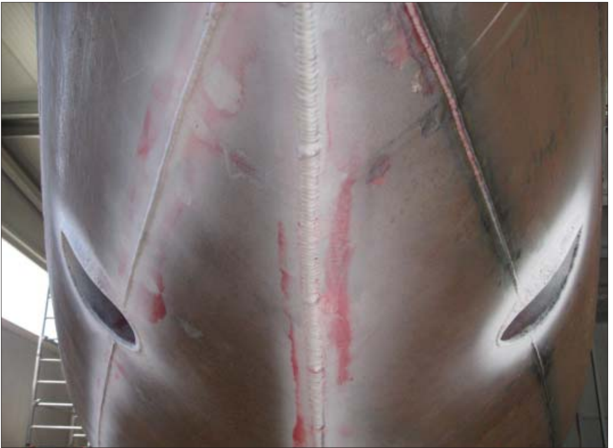
ABOVE & BELOW: Two views of the bow thruster tube; note the touch up of the primer to prevent rust getting a foot-hold on the welded areas of your hull. Welds will be ground above the waterline but unground below the waterline.
