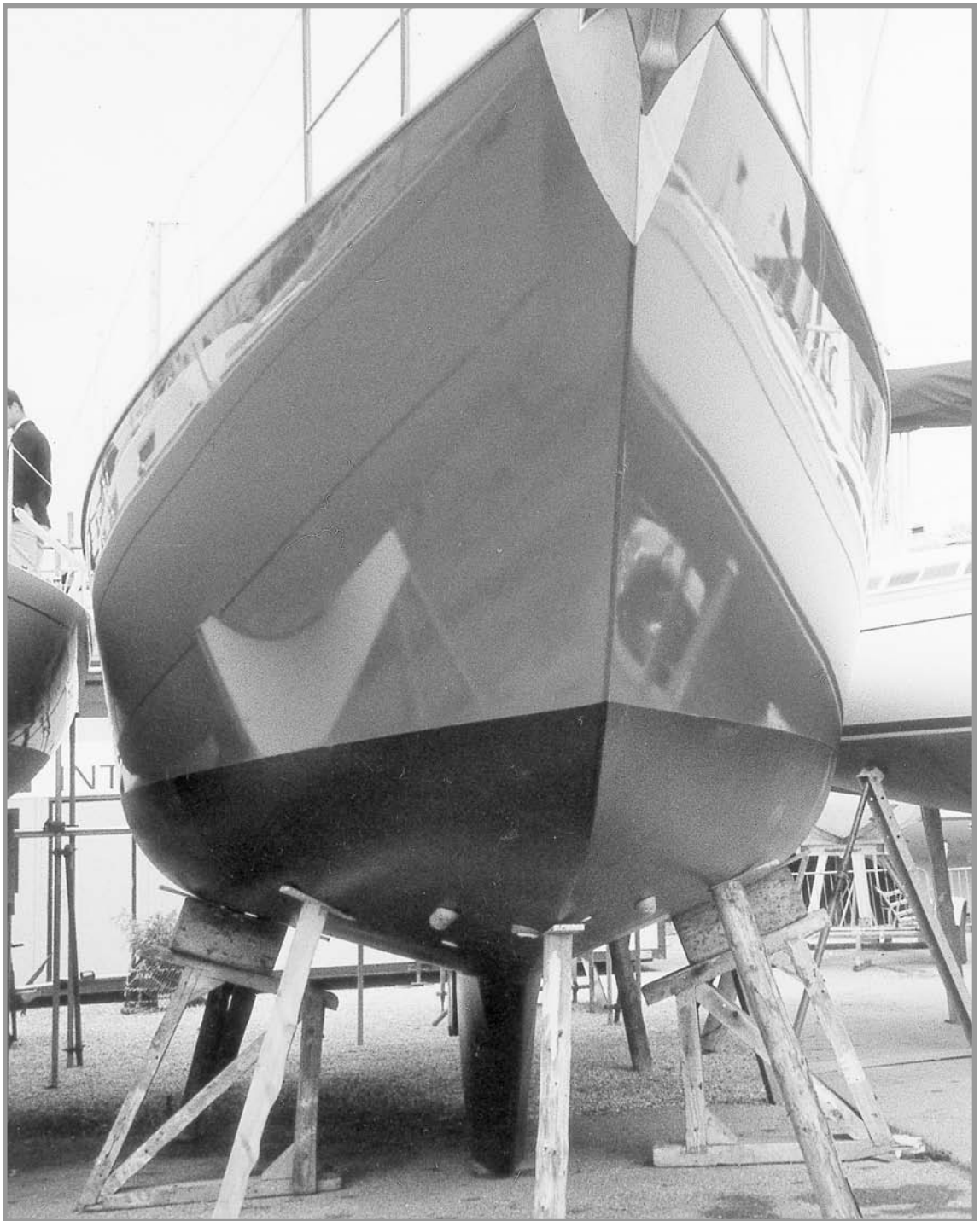
This beautifully painted radius-chine steel Roberts 434 shows the excellent finish that can be achieved on a well-built steel boat. This hull has no filler.
