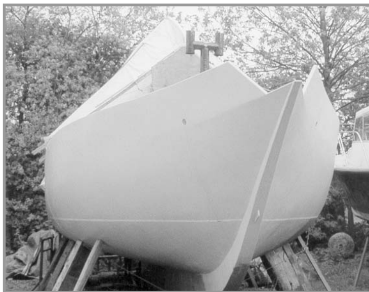
John Reid built this Centennial Spray 36 in England. Reid used a garden roller to roll the plates—no mean effort, even considering his considerable boatbuilding experience. This perfectly fair hull was being fitted out at Iron Wharf Boatyard, in Faversham, Kent, England.
