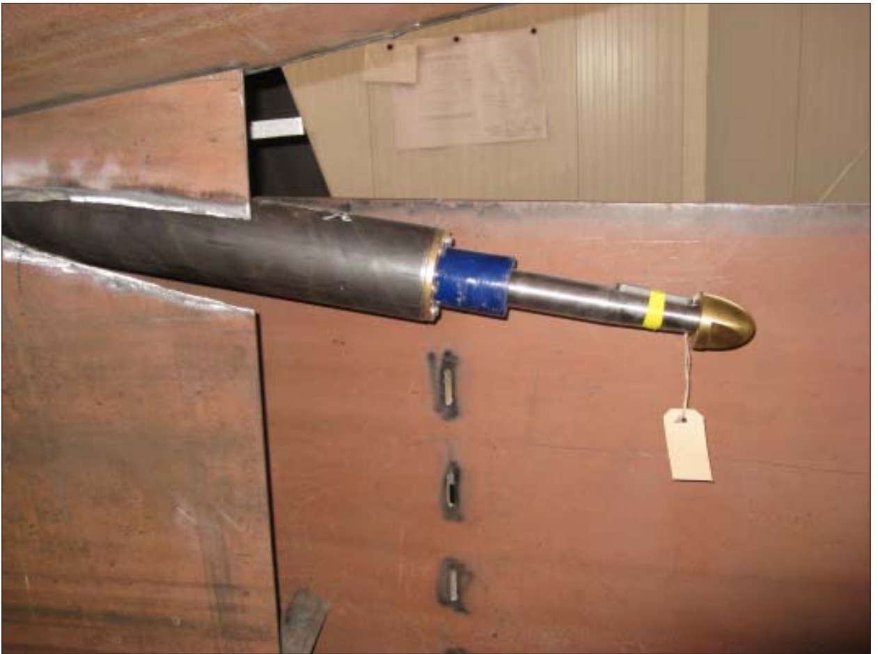
ABOVE & BELOW: Two more views of the prop shaft and where it exits the hull via the aft end of the keel. Always study the plans that come with your cutting files or kit.
