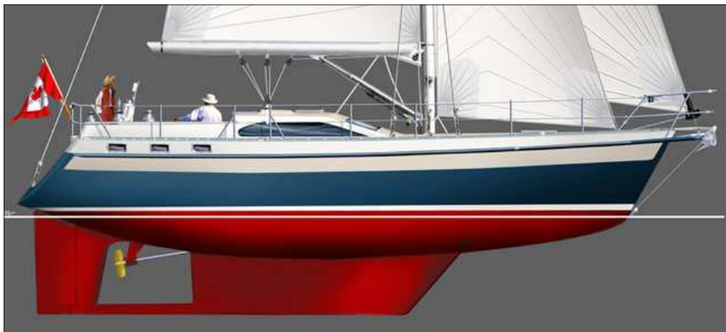
ABOVE: Roberts Safety Skeg is recommended if you build a boat incorporating a skieg and a long fin keel. Available on Roberts designs.
