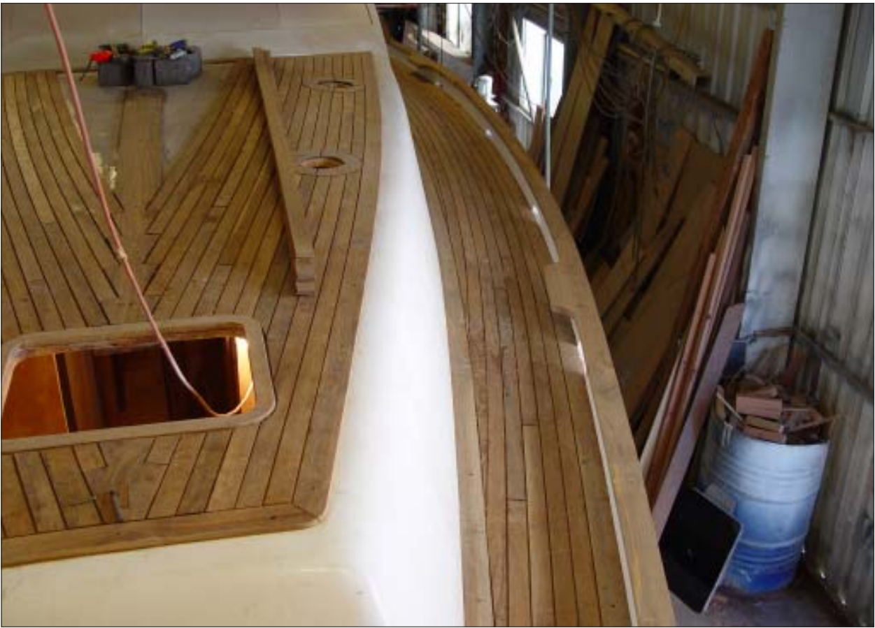
Here we see the completed side and cabin top laid decking - All that is left is to add the caulking.
