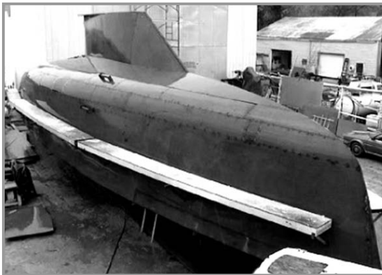
A rain shower shows up the fairness of this New York 65 radius-chine hull built by Howdy Bailey.
