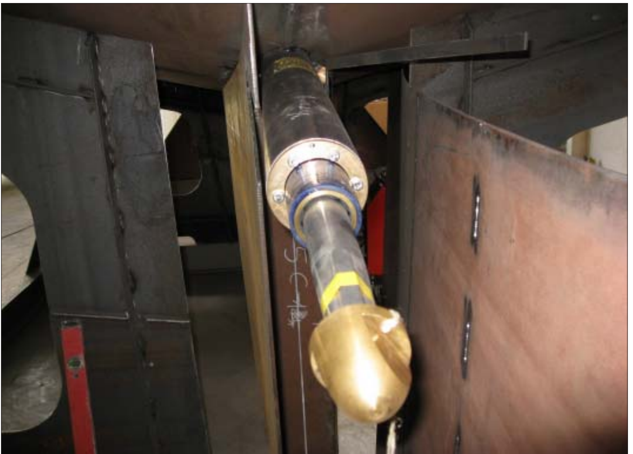
ABOVE & BELOW: Two more views of the prop shaft and where it exits the hull via the aft end of the keel. Always study the plans that come with your cutting files or kit.
