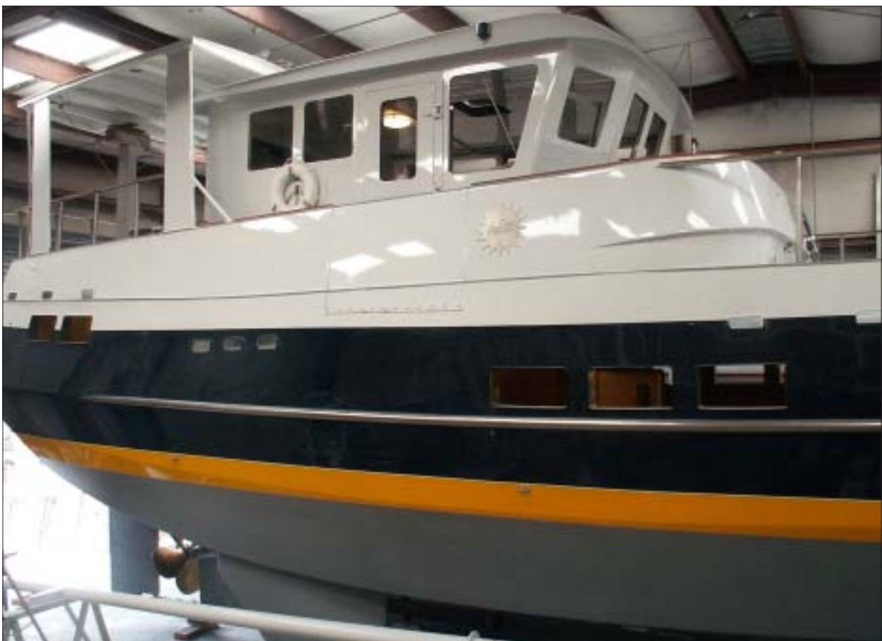
Above is a view of the fine Spray 52 built by Gil Davenport. This design features a steel hull and deck and an aluminum pilot house and makes a fine family sailboat in the style of a sailing trawler.
