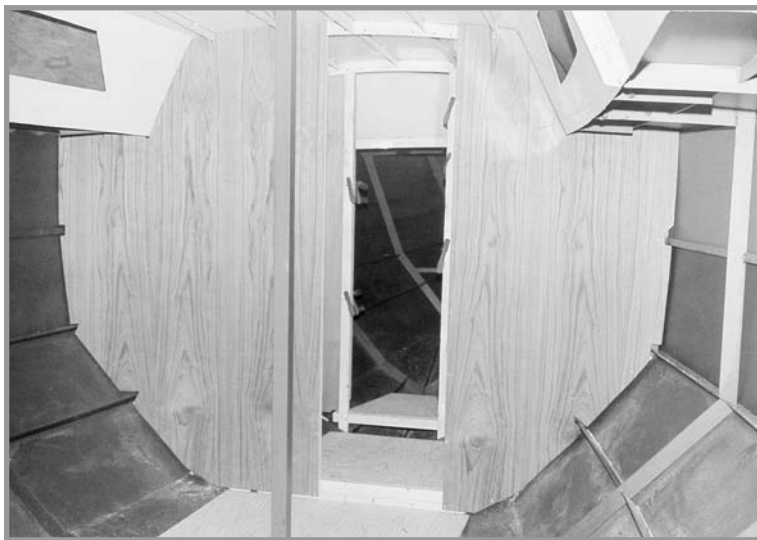
Plywood bulkheads can be attached to frames or to tags especially installed for the purpose.
