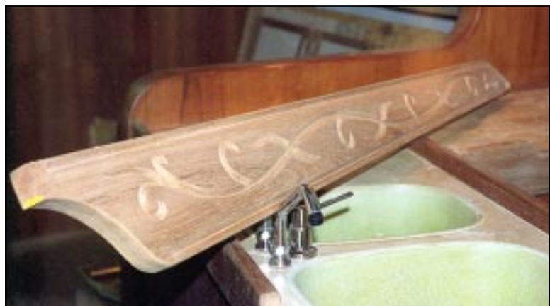
The finished trail board, carved with attractive traditional pattern and ready for final finishing and attachment to the bow.
