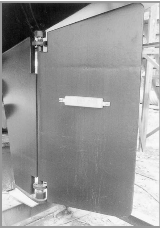
When laying out your anodes, don't forget the rudder.
