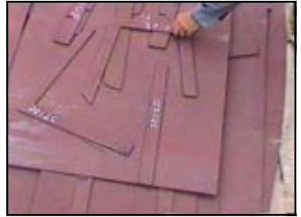
All pieces are marked with code numbers that match with those shown on the plan.
