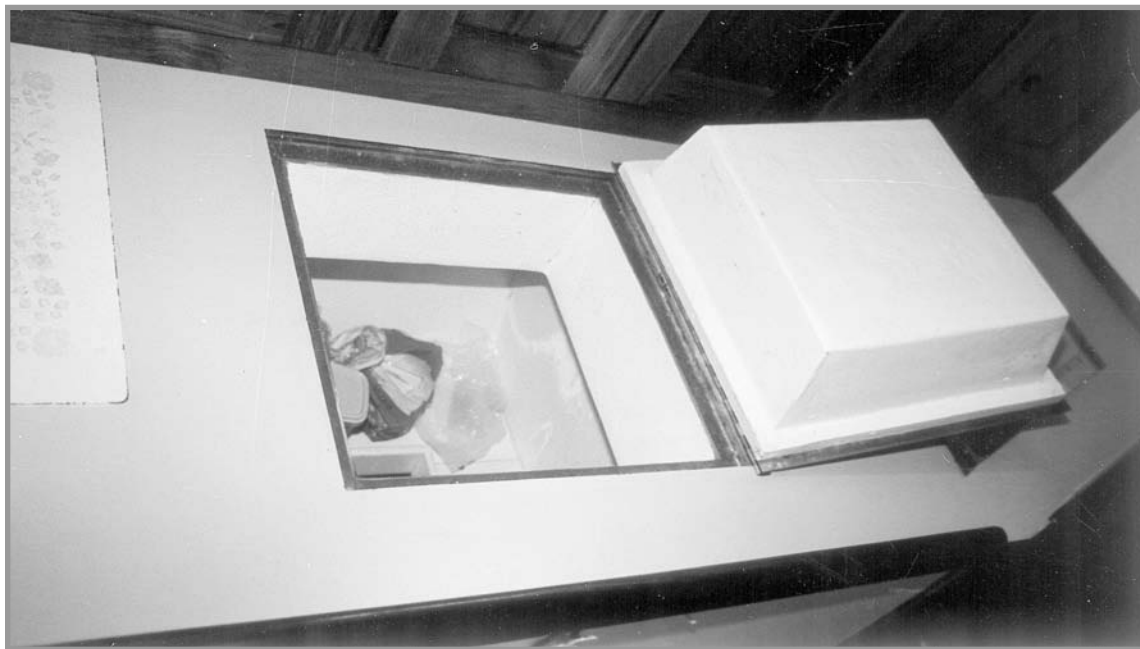
This shows a good design for an owner-built icebox, or built-in refrigerator, a welcome addition to any boat.
