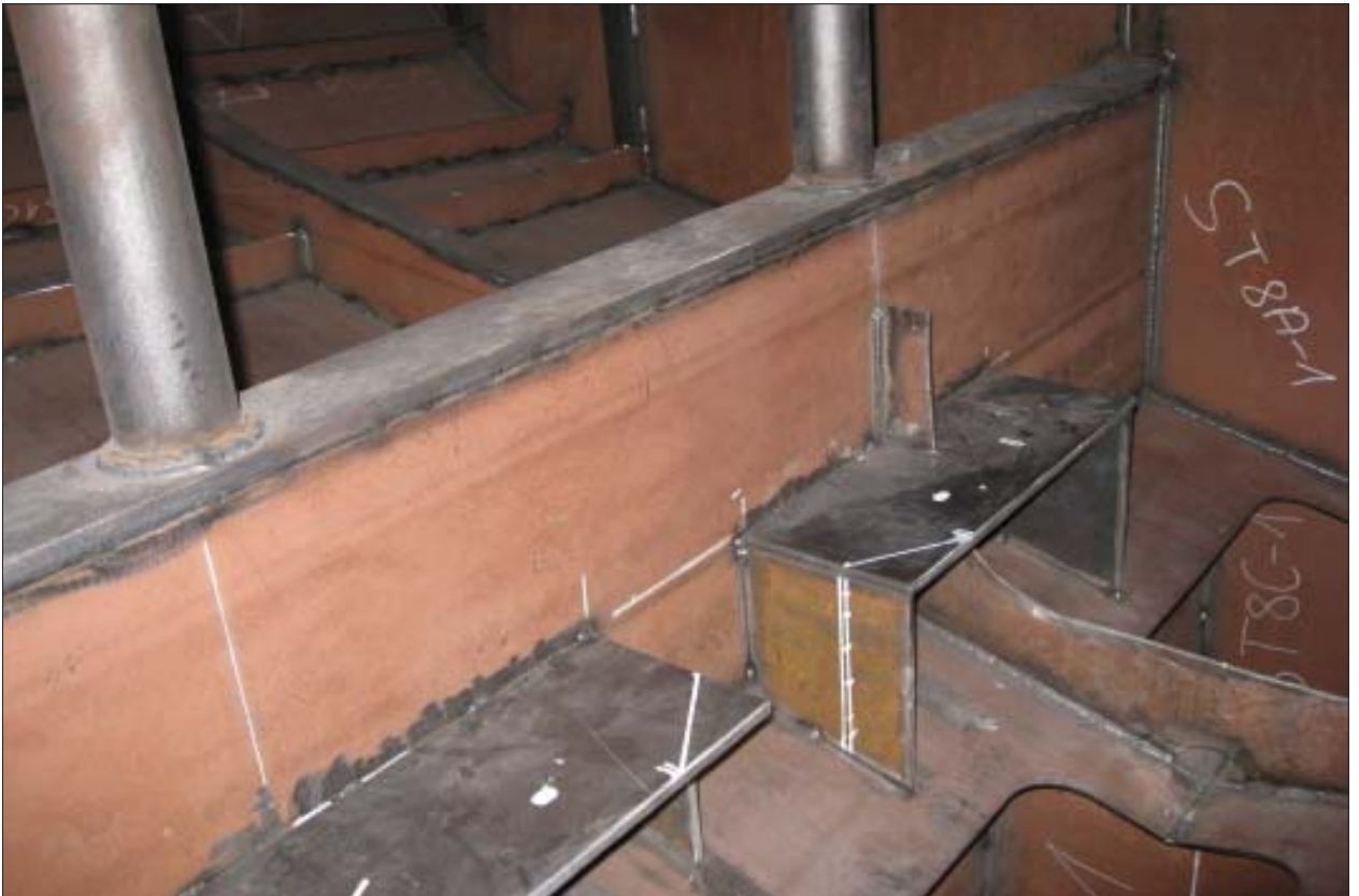
ABOVE & BELOW: Two views of the engine beds which are included in the kit and cutting files but can be modified if required to suit your particular engine.
