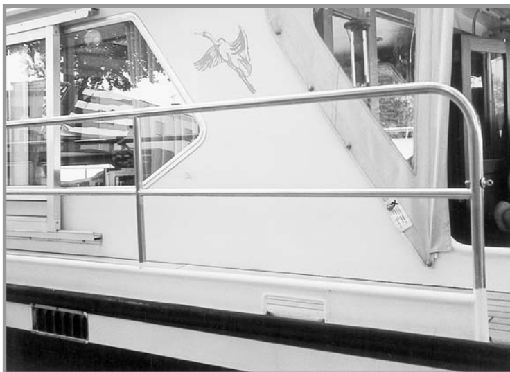
Stainless steel pipe rails, pulpits, and pushpits are recommended on all metal powerboats and can be a great asset on larger sailboats.
