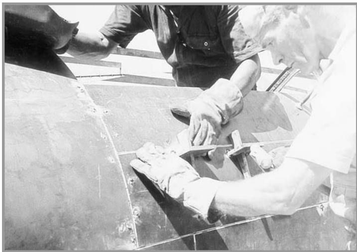
Radius-chine panels around the center of the hull need to be split lengthwise before being fitted.
