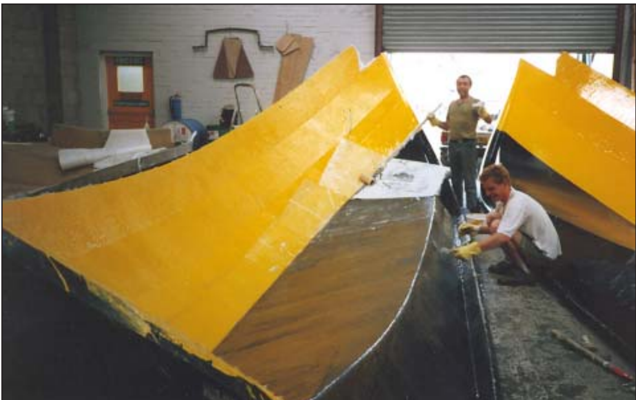
Here we see gelcoat being applied to a Spray 28 female mould.
