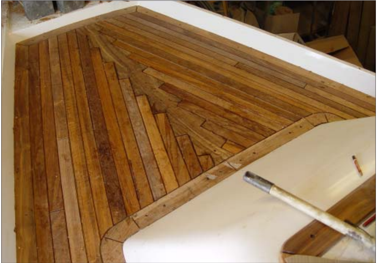
The king plank has now been 'nibbed' to accept the side and foredeck planks as they intersect the centreline plank.
