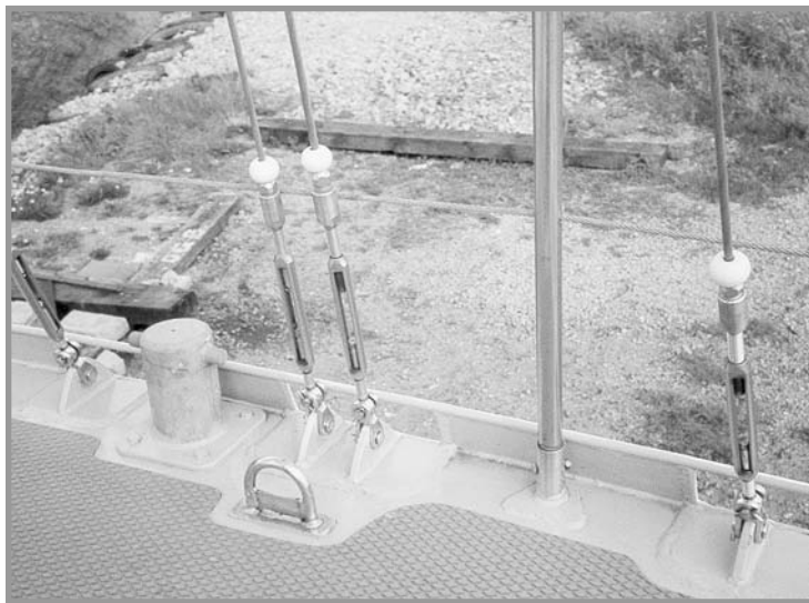
Reinforced chainplates and deck fittings. Note that the Treadmaster deck covering is kept clear of the fittings to allow the free flow of water off the decks.
