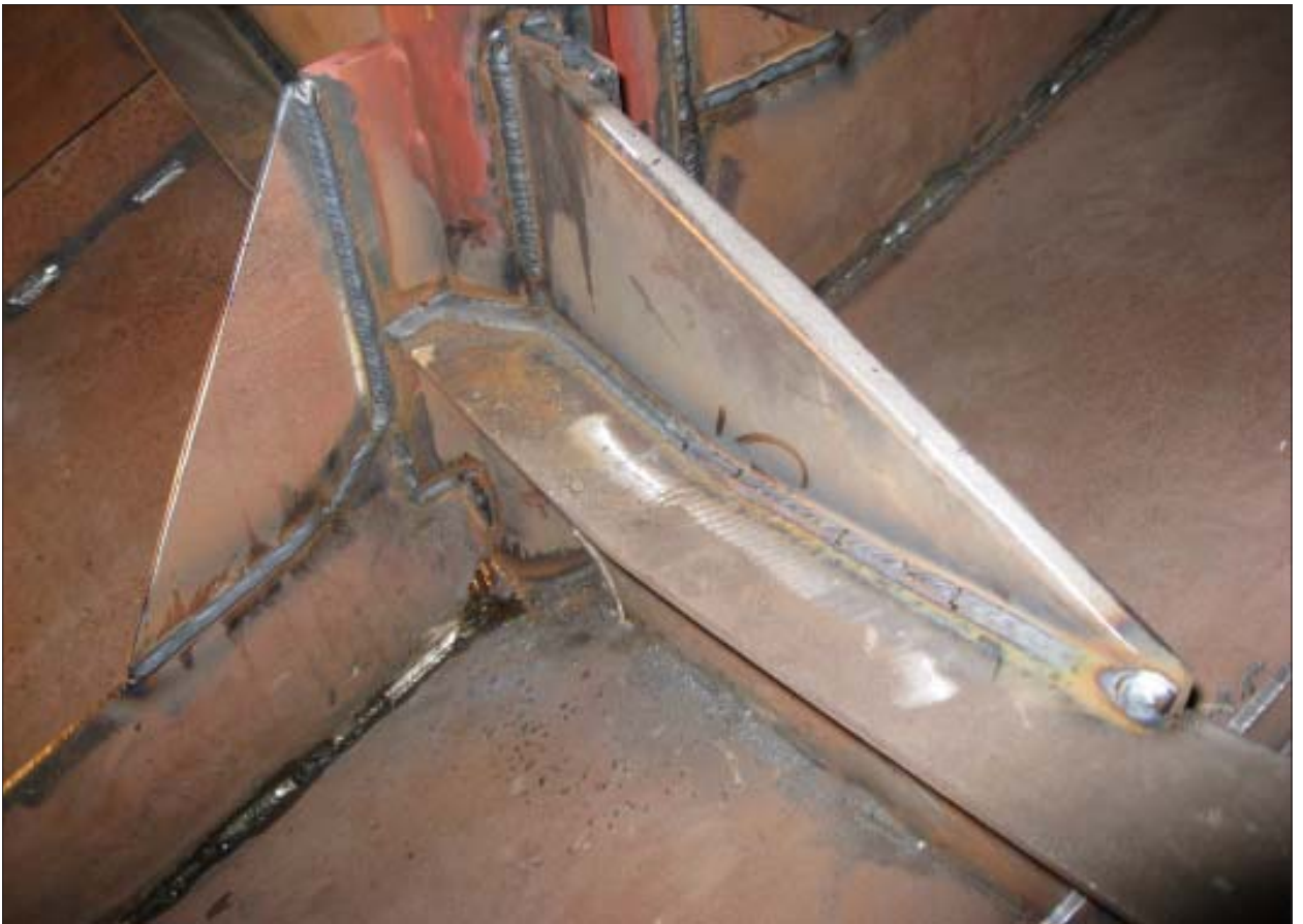
TOP: View of the rudder shaft where it exits the hull; there will be a short tube to carry the shaft. BELOW: Close up view of the rudder shaft with the webs needed to spread the loads in this area.
