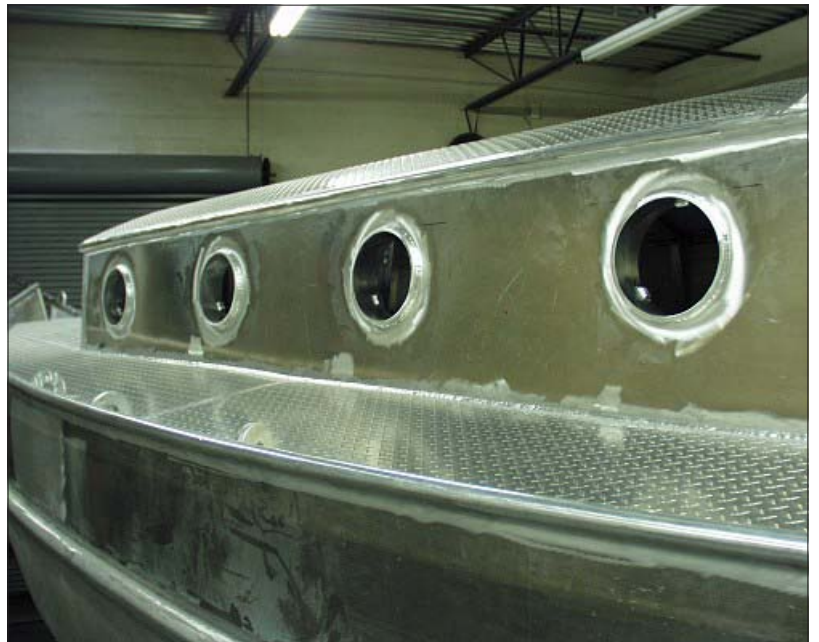
RIGHT: This sequence of photographs is complete when we see the ports installed in the fore-cabin side.
