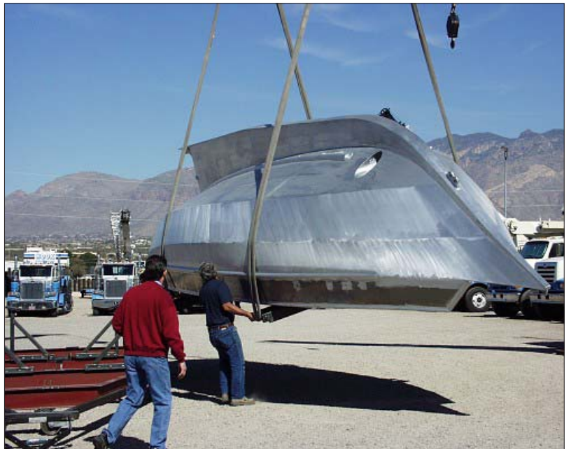
LEFT: Over she goes; only a small amount of man-power is required and in some cases a restraining line is also necessary.
