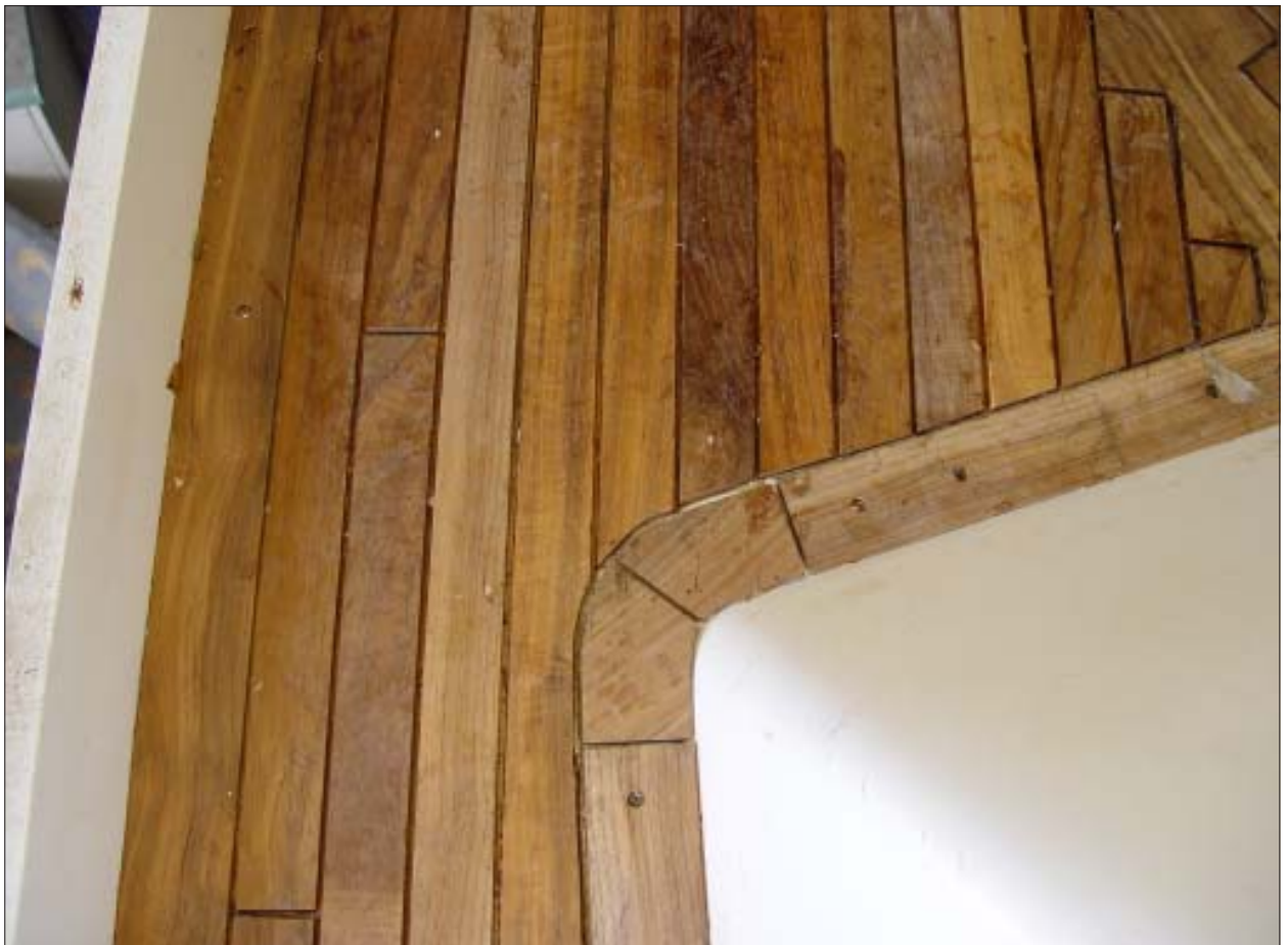
The king plank has now been 'nibbed' to accept the side and foredeck planks as they intersect the centreline plank.
