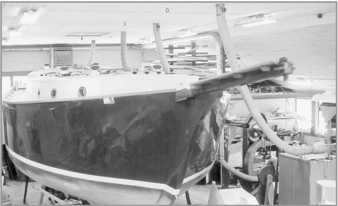
Most Spray designs will accept scrap-steel ballast, thus considerably reducing the cost of the hull. This round-bilge steel Centennial Spray 38 was built in Sweden.
