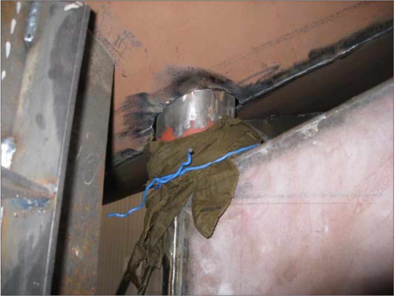
TOP: View of the rudder shaft where it exits the hull; there will be a short tube to carry the shaft. BELOW: Close up view of the rudder shaft with the webs needed to spread the loads in this area.
