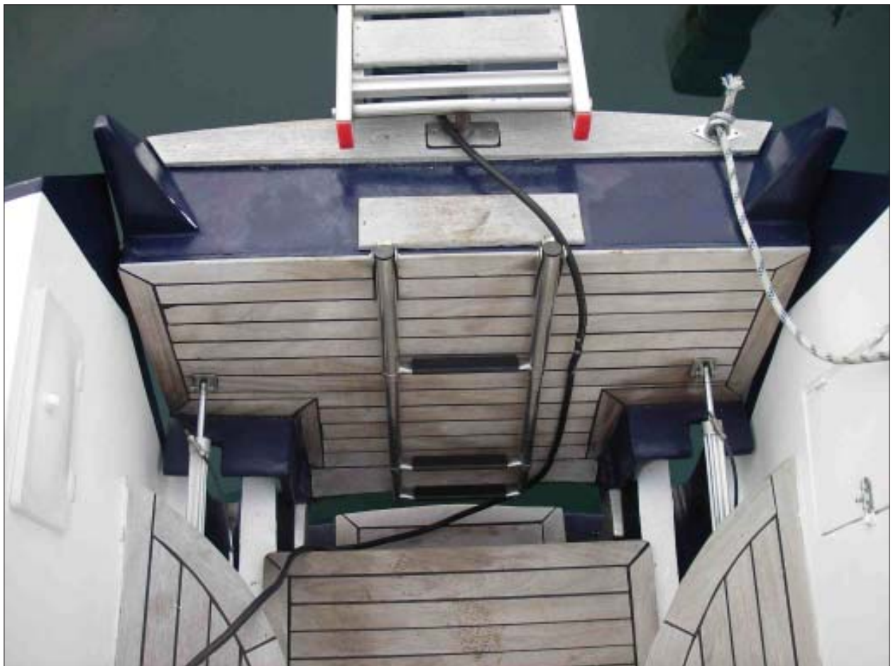
ABOVE and BELOW: The fold down section of the transom combined with a boarding plank makes a nice arrangement especially if you are cruising in Europe where stern to mooring is commonplace.
