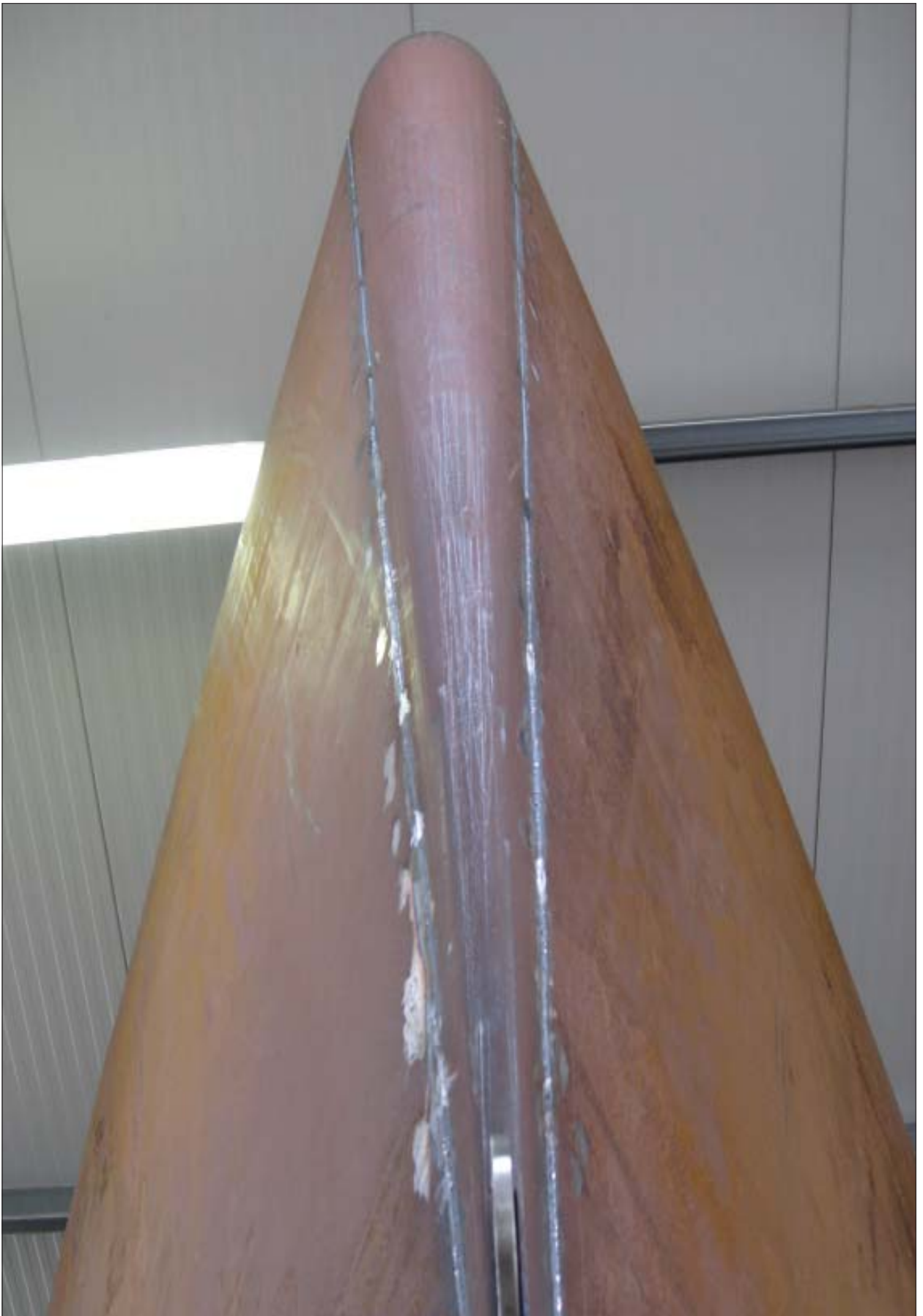
ABOVE: Here we see the bow cone and it is obvious that this type of bow gives a much improved appearance with minimum amount of additional plate forming and welding. The rounded portion is developed as a true cone and made slightly oversize so that it is easy to shape and fit to the hull.
