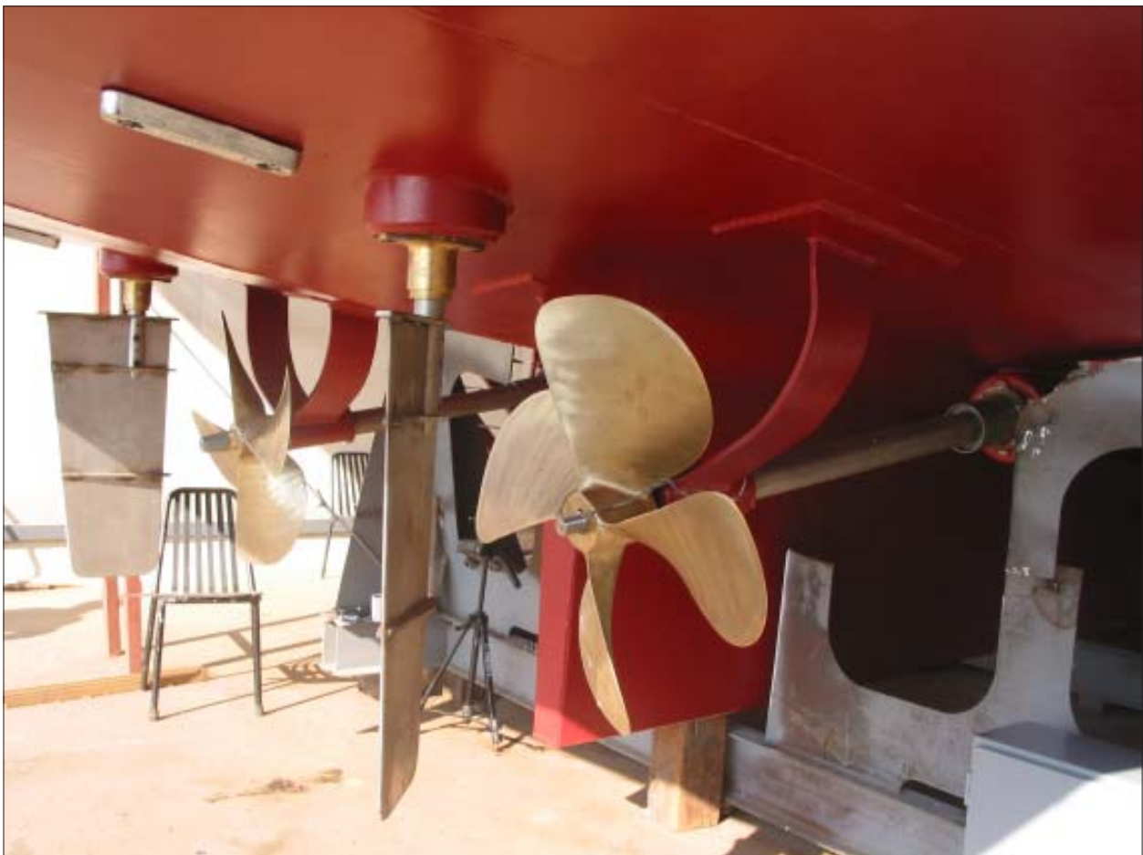
ABOVE: Here we see SPADE rudders which in my opinion are best suited to powerboats !
