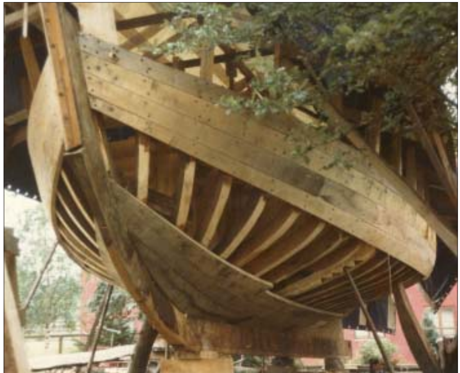
Bow area of a traditionally planked Spray hull, note bent ribs, stem and outer planking.
