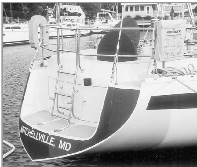
The transom arrangement on this Roberts 53 makes boarding and unloading a dinghy just that much easier.
