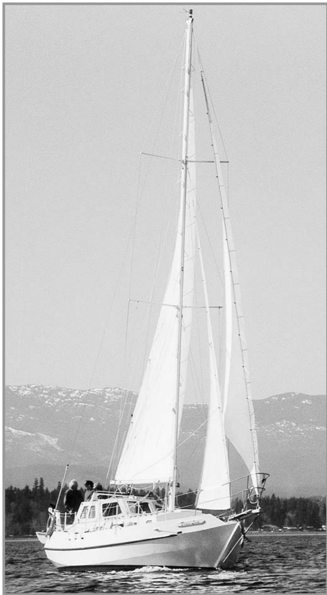
Aluminum was the material chosen by Leuder Kerr for his Spray 33 Brass Loon. This strong hull has successfully withstood contact with many deadheads (near-submerged floating logs) in the Gulf Islands of British Columbia, Canada.
