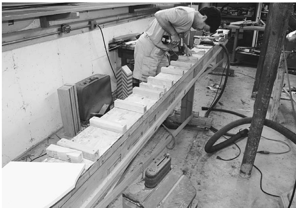
Figure 5-20. Forms are attached to an external strongback with wooden cleats. Mark the strongback with the appropriate spacing with a centerline marked in place. Screw the cleats in place next to the spacing marks.
