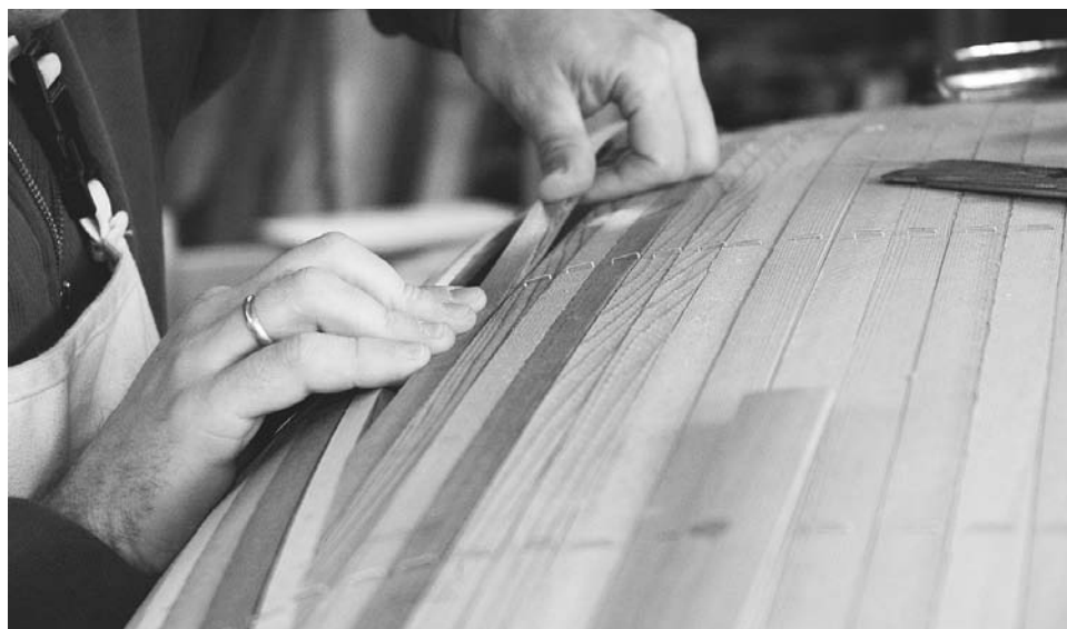
Figure 6-32. With cove-and-bead strips where you are fitting both ends of a new strip, the strip ends up being longer than the visible gap because the strip extends down into the cove of the prior strip. Thus you cannot just drop the fitted strip into place; you must snake it in. It can also be very difficult to remove a strip after dry-fitting it. Instead you will want to rely on accurately making the alignment mark described in Figure 6-27. When you have successfully dry-fitted each end separately and the alignment mark lines up perfectly, add glue to the strip, insert it at one end, then bow it up in the middle to shorten it enough that you can slide the second end in place. The strip should then snap into place.
