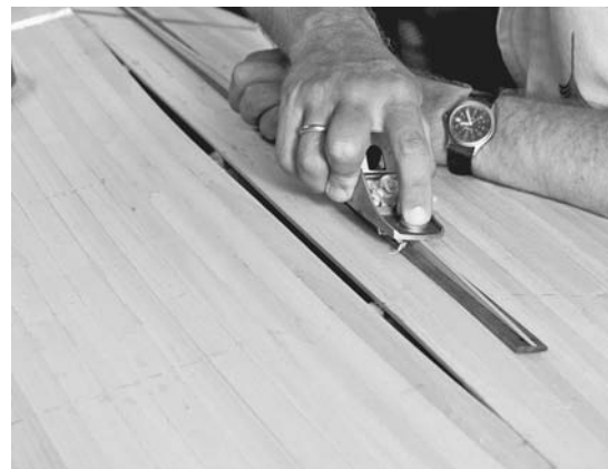
Figure 6-40. Start tapering the strip at one end. Here a piece of scrap protects the boat while allowing me to work right where I need the strip. Test the fit at this end, planing farther along as the tip starts to fit well. Try not to go beyond the previously made marks as this will indicate you are losing some of your margin of error for fitting the other end.
