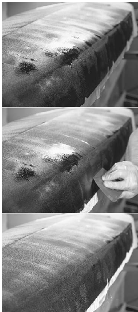
Figure 9-19. After wetting out the glass there are bound to be areas with excess resin as well as some with too little. Starting at the center-line, hold the squeegee at about a 45-degree angle. Pull the squeegee toward the edge, maintaining approximately the same angle as you roll down the side. Clean the epoxy off the squeegee by sliding the edge through a slot in a paper cup.
