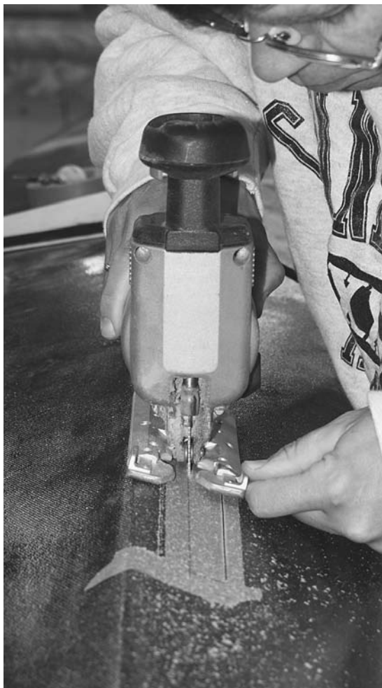
Figure 13-60. I installed a retractable skeg on this boat. This involves installing a skeg box in the bottom of the boat. The skeg is offset to one side to reduce the chance of pebbles jamming it when dragging the boat up a beach. Install the skeg box by cutting a slot in the bottom of the boat. Here it is offset from the centerline to reduce the chance of a pebble getting jammed into it. As shown, the jigsaw is set at an angle to cut an approximately vertical hole. Insert the skeg box through the hole and tack it in with CA glue and fillet, then fiberglass it on the inside and trim it flush on the outside. After trimming, ease the corners and glass over the end grain on the outside.
