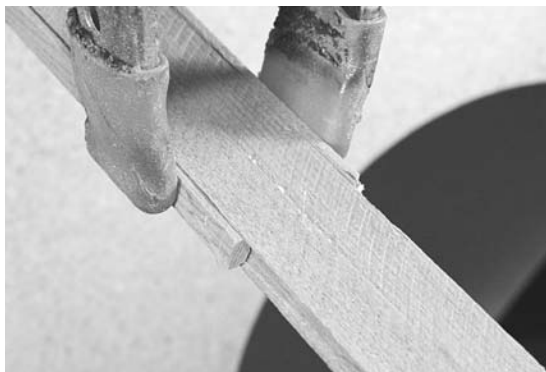
Figure 11-14. Along the centerline using cove-and-bead strips you will want to have coves facing out on both sides. You can quickly clamp together two strips with a spring clamp, but you need to protect the sides of the cove. Some short pieces of strip cut down to just the bead may be fitted in the cove as a flat surface for clamping.
