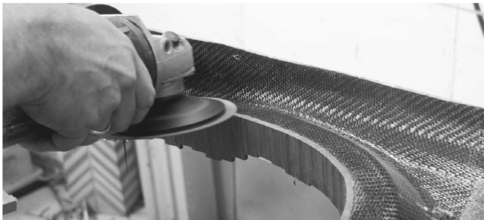
Figure 13-52. When you turn over the deck you can trim off the bottom ends of the coaming riser strips. First clean out any hot-melt glue squeeze-out. The glue will quickly gum up any sandpaper or rasp. I use a high-speed right-angle grinder to bring the strips down even with the deck interior. A 36-grit disk makes quick work of the task even if it does send dust everywhere. You need to be careful, as it will grind through anything without a second thought. The disk may also be handheld to round over the edge after it has been trimmed.
