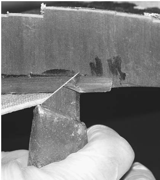
Figure 13-54. Since the laminations are not completely around the front of the cockpit, you need to finish off the front. Trim the ends of the lamination at a tangential angle with the coaming riser, creating a smooth curve across the front. Cut a piece of \frac{3}{16} -inch-thick curly maple to fit across (you could also laminate pieces instead).
