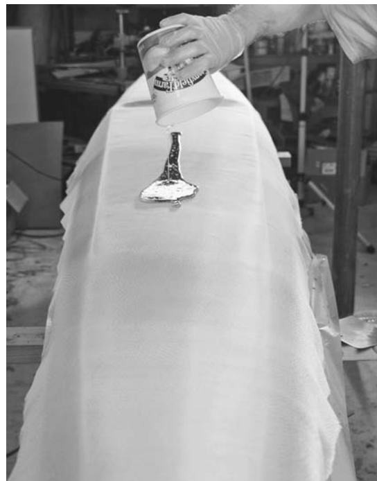
Figure 9-2. Once the epoxy is mixed, the chemicals start doing their thing. The longer they are in a concentrated mass the faster they will react. Dumping your mixing pot onto the boat quickly will slow down the reaction, giving you more time to work.
