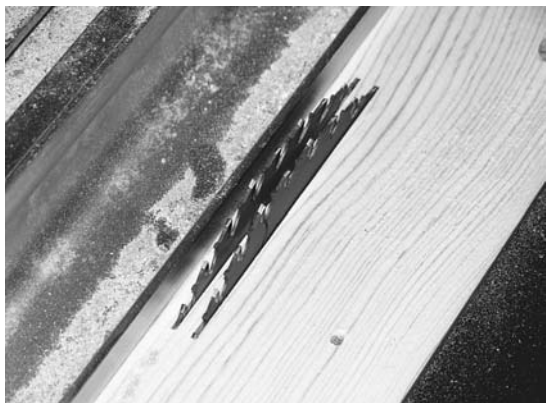
Figure 5-4. You can save some time at the table saw by ganging together several blades on the saw arbor. I use a blade stabilizer as a spacer between the blades. Note that ganging up blades can be very dangerous if you are hand feeding the boards through the saw. I don't recommend this without using a stock feeder.
