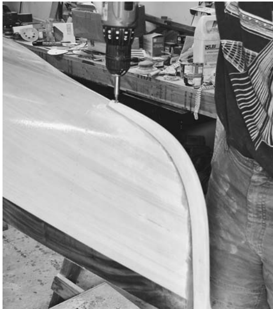
Figure 12-28. It will help if you do some preliminary shaping before installing the stem. Butter up the mounting surfaces with dookie schmutz. A screw at each end of the stem should be enough to clamp it in place. Clean off the squeeze-out before it hardens.
