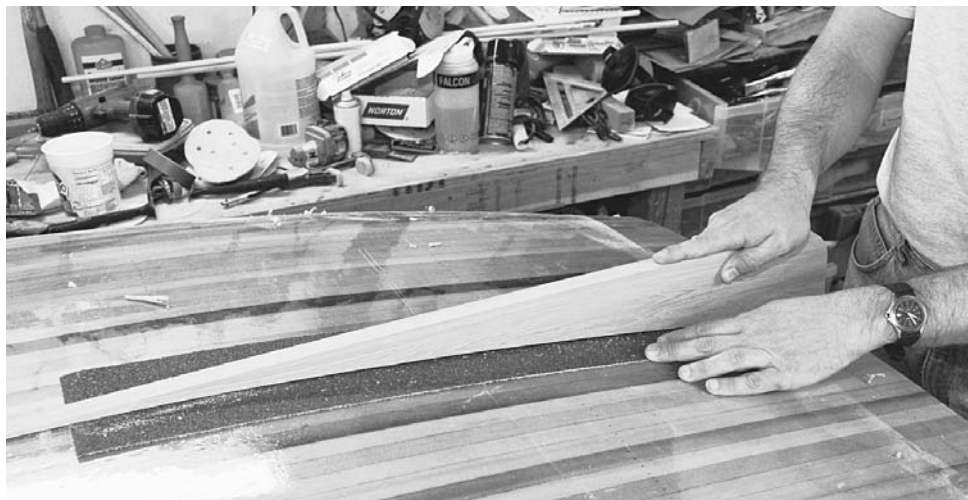
Figure 11-37. Such a short boat needs a little help going straight. A short keel at the stern of the boat, sometimes called a “skeg,” provides this directional stability. Cut a skeg out of some \frac{1}{2} -inch plywood or \frac{3}{4} -inch solid lumber to the approximate shape. Then lay a long piece of sandpaper on the spot where the skeg will be installed and rub it back and forth to create a tight seam. Round off the exposed edges of the skeg with a \frac{1}{4} -inch-diameter router bit.
