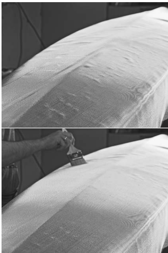
Figure 9-10. After draping the glass onto the boat you will have small wrinkles and bubbles. You want to try to get the cloth as tight to the boat surface as possible before applying resin. Do not run your hand over the surface in an attempt to smooth the fabric. This will tend to cause creases and snags. Instead, use a chip brush to smooth the surface. Start in the middle and work out to the sides and ends.
