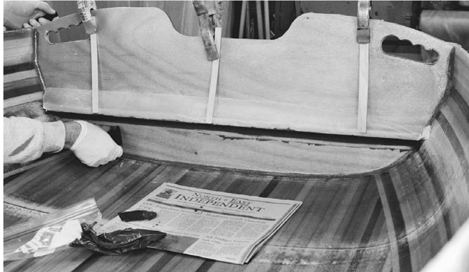
Figure 11-32. The intersection of the backseat and back transom will need some reinforcement. Normally I would create a fillet underneath, but the only access to this area will be a small hole in the seat support. Therefore, I opted to make a fillet before installing the seat. You could glue and screw a cleat of wood into this position, but I like the rot resistance of a fillet in this location. A solid piece of wood as a cleat could be covered with fiberglass and epoxy to protect against rot, but this method is quicker.
