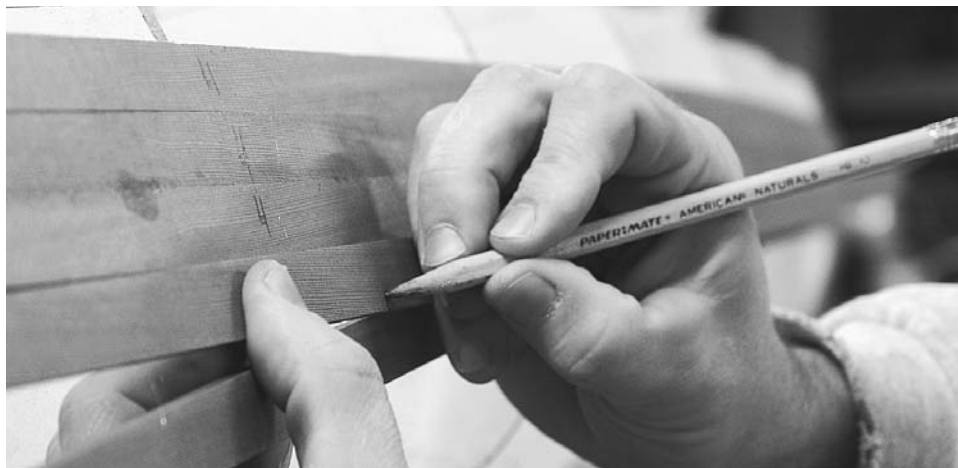
Figure 6-21. Long tapers such as for the cheater-strip area at the ends of a kayak are fitted in the same manner as other tapers. Hold the strip in place with the end aligned with the end of the tapered gap and mark where the new strip overlaps the gap, then whittle off the excess wood and plane the strip to fit. In these gaps the taper is often not a straight line but follows a curve, so the new strip must be slightly concave along its length. A couple of extra strokes with the plane near the middle of the taper is usually enough to create the curve.
