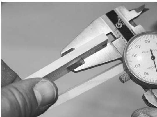
Figure 5-5. A smooth, fair surface on the boat starts with uniform-thickness strips. Check the strips as they come out of the saw to make sure they are at least as thick as you need after thickness planing. Check a few scraps through your thickness planer before running your strips, and spot-check as you go to make sure nothing moved.
