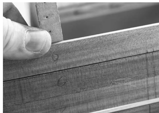
Figure 6-15. With most boats the sides are relatively flat, so very little beveling is required. Most small boats, however, will have some places where gaps will open up if you are using square-edged strips. These gaps may be eliminated by planing a rolling bevel as described earlier. Notice the double lines on the strips near the right side of the photo. These help align the grain while installing strips cut consecutively from the board.
