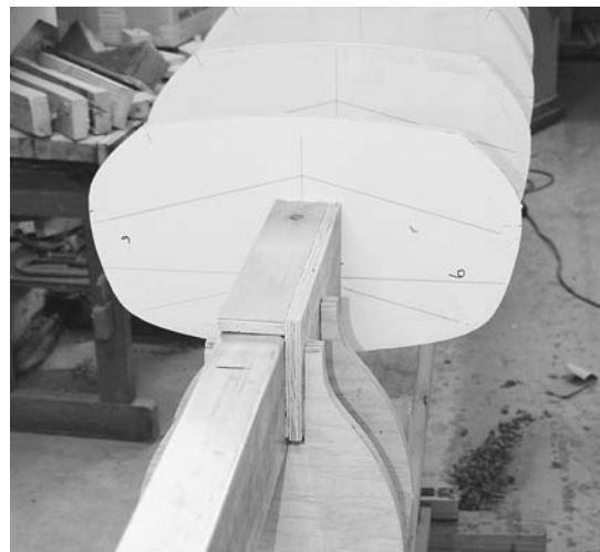
Figure 5-23. With this aluminum strongback, I use L-shaped spacers to hold the forms in place. The end forms are screwed in place, and wedges between the middle forms hold everything tight.
