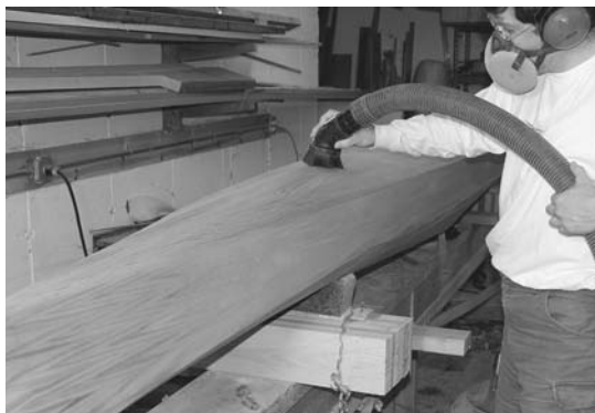
Figure 7-14. Sandpaper leaves a little bit of grit behind that will continue to scratch the boat when you switch to a finer paper. Vacuuming the boat between grits may help you get a better finish. A final vacuuming of any residual sanding dust when you are done will give a cleaner look to the final finish.
