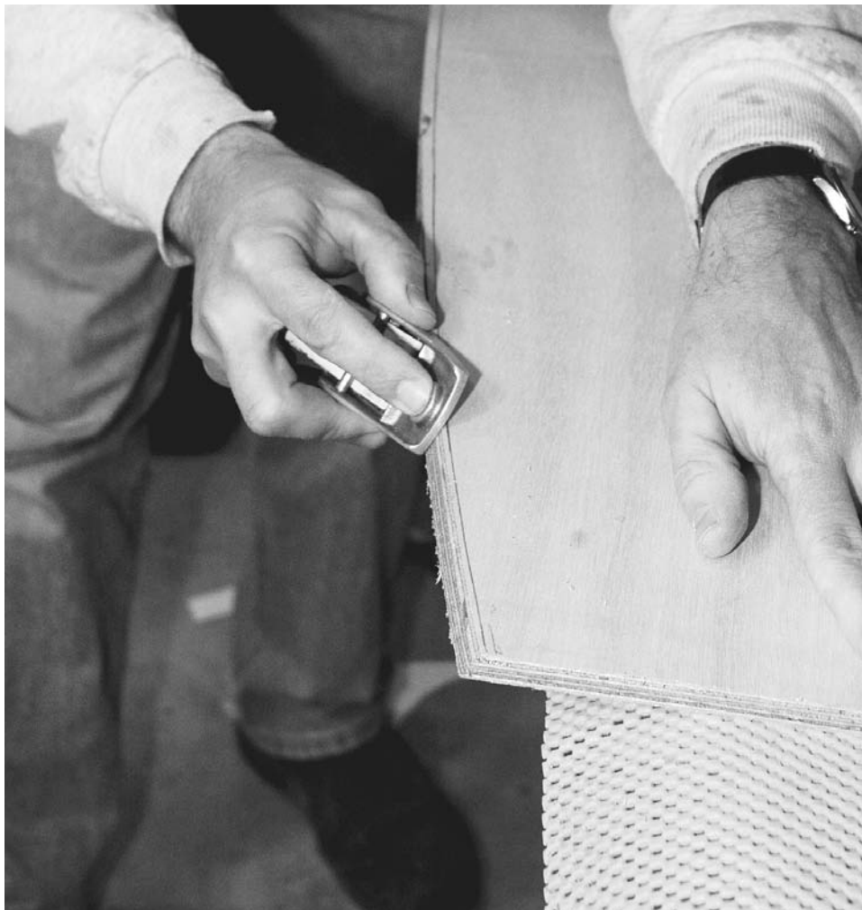
Figure 11-27. The seats are cut from \frac{1}{2} -inch okoume marine plywood. I had them cut with a CNC router, but these pieces could all be cut with a band saw or jigsaw. The bottom edges of the seats need to be beveled to match the curvature of the hull. On the short, curved sides of the backseat the bevel will angle back about \frac{1}{4} inch near the back corner and roll over to a bevel about \frac{1}{8} inch wide as it approaches the forward edge of the seat. The front seat needs more aggressive beveling of the curved sides, starting with a \frac{1}{8} -inch-wide bevel near the horns on either side, rolling over to a nearly 1\frac{1}{4} -inch-wide bevel at the front of the seat. A good sharp block plane makes quick and easy work of this task. Test the fit to see that the seats will sit down in the boat, with the top edge of the seat tight against the side of the boat. If you need to overdo the bevel a little to get a tight fit, that is OK. Do not remove material at the top edge as this will change the outline shape of the part. If you cannot get a tight fit around the edge, you can fill in the gap with dookie schmutz later. A rasp comes in handy for rounding off the corners where they will fit against the fillet between the strips and transom. Start with a \frac{1}{2} -inch-diameter radius and adjust the fit as needed.
