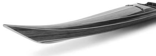
Figure 10-15. You can get results almost as good as spraying by careful brushing followed by rubbing out and polishing the result. This Night Heron was sanded with 600- through 2,000-grit sandpaper and then buffed with polish.
