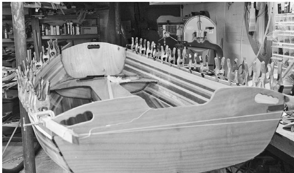
Figure 11-34. I installed an outwale only. Having no inwale makes it easier to drain the boat. Glue the outwales to the sides of the boat by applying a layer of epoxy thickened with colloidal silica. Spread the mayonnaise-consistency glop on both the boat and the gunwale stock. Protect the side of the boat below the gunwale with masking tape so drips won't make a mess. Install the outwale just below the top edge of the strips.
