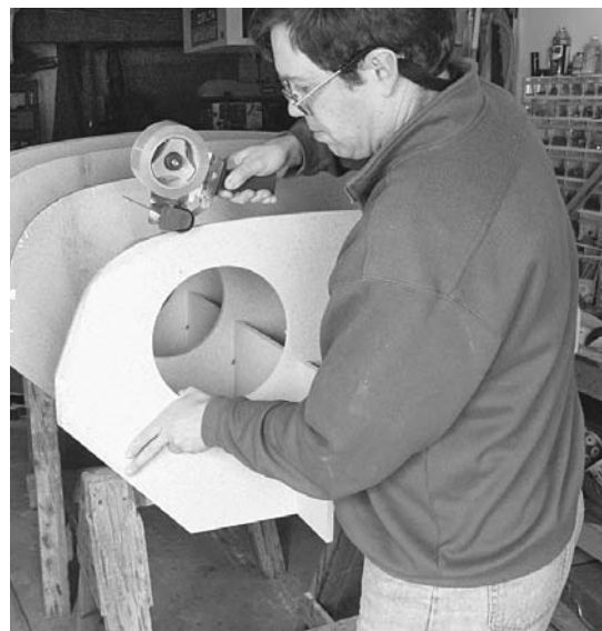
Figure 5-25. Wrap tape around the edges of the forms to keep glue from sticking. This clear packaging tape will assure nothing sticks at all. Masking tape also works well. It allows the glue to help hold the strips to the forms a little bit, but it still lets the glue break free when needed.
