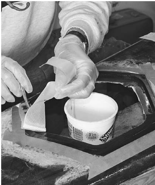
Figure 13-62. The hatches need a spacer between the lip and the deck to allow for a gasket. The spacer is set in epoxy thickened with colloidal silica to make a mayonnaise-like glue. Try to clean up any squeeze-out while the glue is still wet. After the glue has set, clean up the inside edge of the hole.
