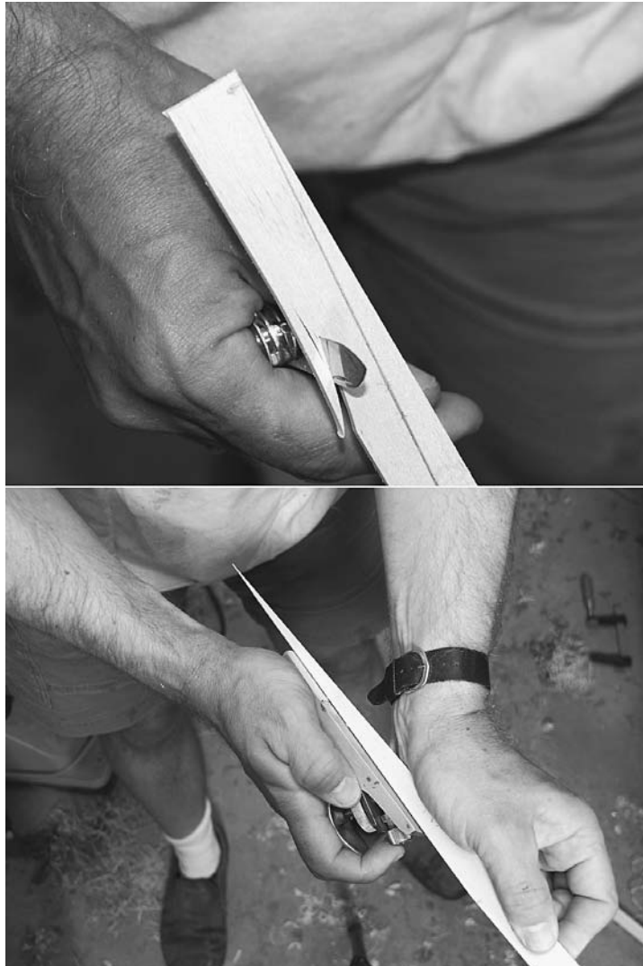
Figure 12-19. Use a jackknife to roughly remove the excess material on the strip end.
