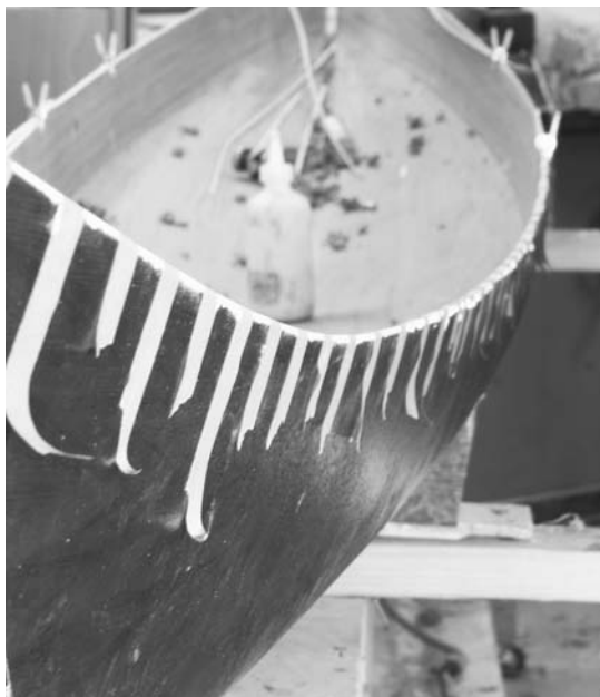
Figure 8-2. Staining some of the wood stains all of it. If you want an accent strip, it may be easiest to add it after the wood has been stained. Here the outside of the hull has been stained and fiberglassed. I'm applying a thin strip of wood to the top edge, and then I'll glass the inside. I'll glass the outside when I attach the deck.
