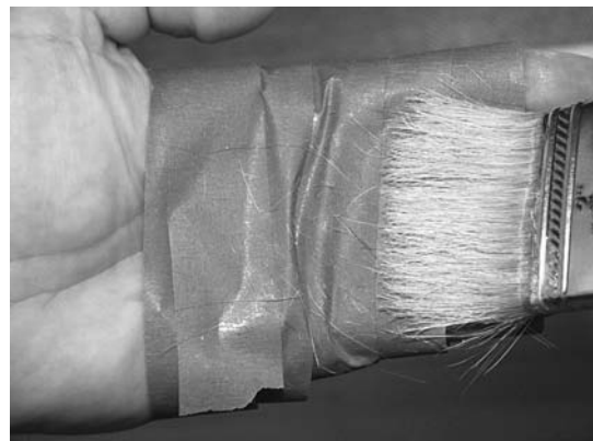
Figure 9-29. Most of the bristles that are still loose after gluing can be removed by vigorously wiping the brush against tape wrapped around your hand with the sticky side out. You may find an occasional stray hair as you paint epoxy on the boat that you can lift off with the tip of your brush.
