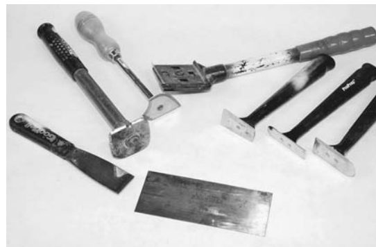
Figure 3-4. A paint scraper has a variety of uses, from removing glue drips to shaping concave surfaces. My favorite is the one at the top left with the thick handle. This started out with a square blade, but I have ground a variety of different curves at the corners and sides to conform to a variety shapes. I was hoping the wood-handled unit to its right would prove useful since it is preshaped to some good contours, but it was too light. The cheap hardware store version on the top right is much better. The three little ones to the right are useful despite being light. They reach into small spaces well. At the bottom is a cabinet scraper. This does not get much use on softwoods, but it can quickly level off a sag in epoxy. The putty knife to the left can be used as a scraper, as a lever for aligning kayak decks, or even for applying putty.
