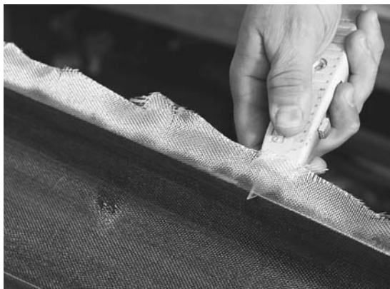
Figure 9-24. Run the edge of a utility knife right up against the edge of the wood to get a very close trim. Cutting off a small amount of wood only means you are getting a smooth, flush trim.
