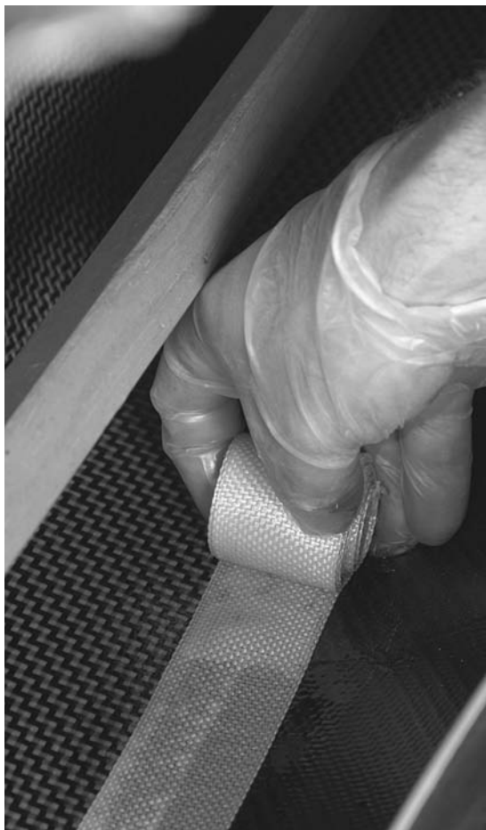
Figure 13-69. Bonding the deck-hull seam is no fun, but it is over quickly, and it is really the best, strongest, lightest solution. As described in Chapter 9, you must run a length of prewoven tape down the inside seam. Here I am using a 1½-inch wide Kevlar tape. I'll roll it by hand as far down the seam as I can reach, then break out the brush-on-a-stick.
