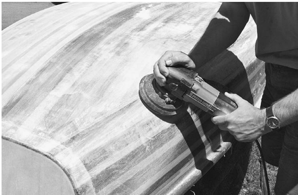
Figure 11-38. The fill coat should leave a quite smooth surface, but a good finish often requires some serious sanding. Start with 60-grit sandpaper on your random orbit sander. On the boat shown there were some rough spots along the edge where the fiberglass doubled up. The goal is to feather in these edges and level any irregularities in the surface so there are no shiny spots left on the surface. Along the edges of additional layers you will need to sand into the glass a little bit. However, if you start seeing signs of the fiberglass showing up elsewhere in the surface immediately adjacent to shiny spots, stop sanding that area. You will need to add another fill coat.
