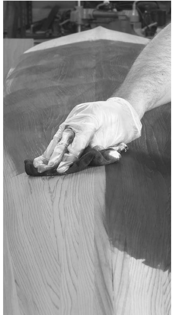
Figure 8-1. Alcohol- and water-based stains dry quickly. Get your rag very wet with stain, and move it quickly. A dry rag will create a splotching color. If you want a lighter color, follow the stain manufacturers instructions, which typically involve adding a thinner or reducer to dilute the color.
