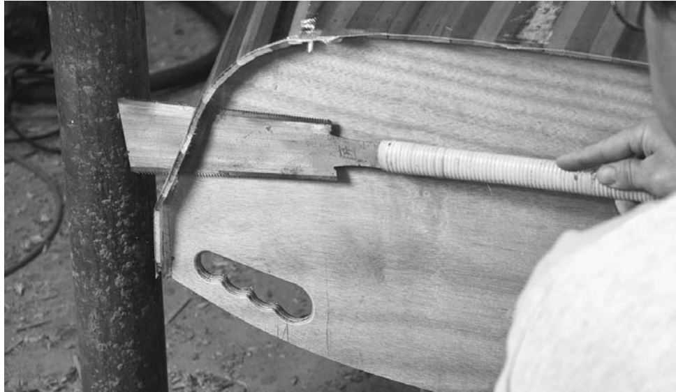
Figure 11-22. Trim the ends of the strips even with the transom. A Japanese pull saw does a good job trimming quite flush, but it is possible to get out of alignment and scar the transom. Be careful that the blade is not scratching up the transom as you cut. Round over the corner with a block plane and sand it to prepare for fiberglassing.
