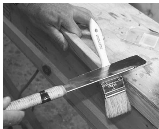
Figure 9-34 Unless you have really long arms, you will need a special tools to access the far reaches of the deck/hull seam—enter “brush-on-a-stick.” Screw a chip brush to the end of a 1-inch by 1-inch by about 8-foot stick, and then saw off the brush handle.
