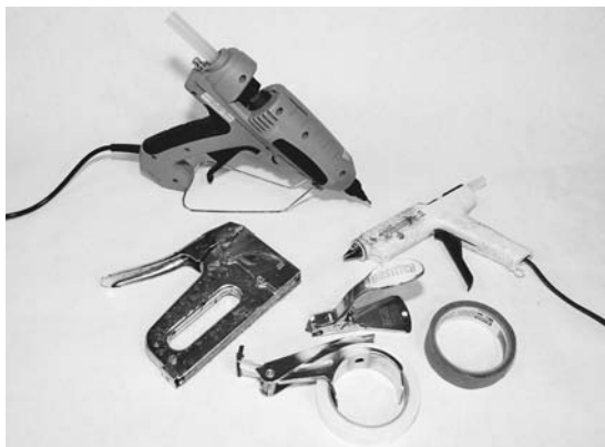
Figure 2-7. The strip planks need to be temporarily secured to the forms. The widely available T-50 utility staple on the lower left is the standard. I like the Bostitch heavy-duty staple remover. It does a good job of pulling the staples without damaging the strips. If you prefer, hot-melt glue can be used instead of staples. The glue sticks are strong enough to hold the plank in place but weak enough to break when you are done. Masking tape or strapping tape also provides a good, quick, temporary clamp to hold together adjacent strips.
