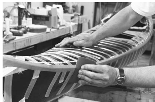
Figure 9-33. Apply tape across the seam every 4 to 6 inches to be sure the seam does not pop while you are working on it. When the seam is aligned and secure, apply a strip of masking tape along the seam to keep the epoxy in. Burnish down the tape so there is no room for epoxy to collect.
