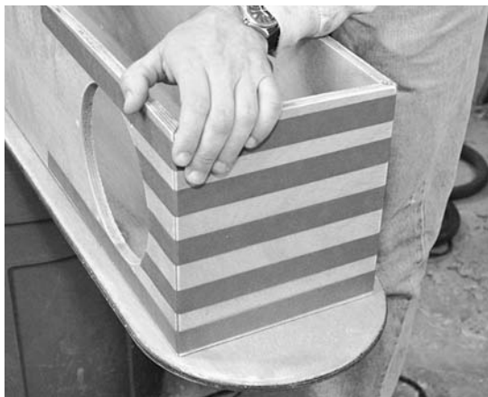
Figure 11-31. With the seat support parts laid out flat and edge to edge, tape across the joints with masking tape. When you fold the parts into position on the seat, this tape will keep the joints tight. Spot-weld all the parts in place with CA glue before removing the tape. Use a heat gun to heat up the all the joints, and then paint in some unthickened epoxy. Capillary action will suck the resin into the joint. Apply fillets of dookie schmutz along the joints between the supports and the seats, as well as the corners between the seat support parts, to create the final bond.
