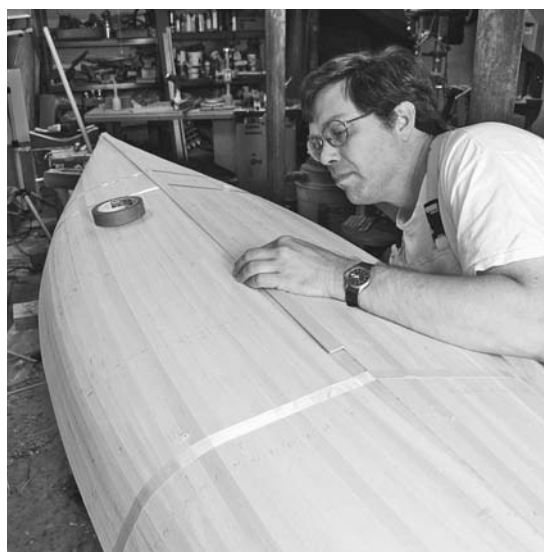
Figure 6-39. Eventually there will be a last strip. Remember to make the edges of the second to last strip, and maybe the third to last strip, square so you don't need to try to fit the ends down into long holes created by a cove. Place a strip over the hole and reach in underneath to trace the shape of the hole on the underside. Without moving the strip, also mark the ends of the hole on top. Bend a scrap strip over the marks you made to indicate the approximate shape of the hole. Either whittle away most of the excess wood or cut it off with a band saw.
