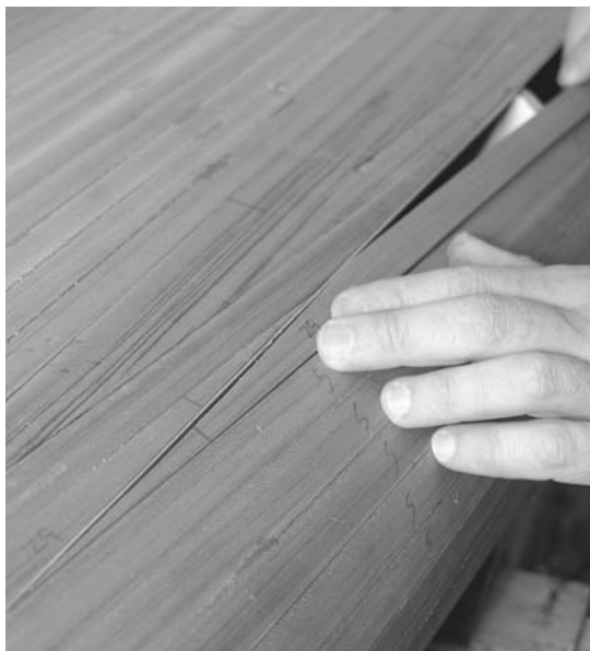
Figure 13-32. With careful marking, cutting, and fitting I was able to make the strips on either side of the line continue with minimal interruption of the grain.
