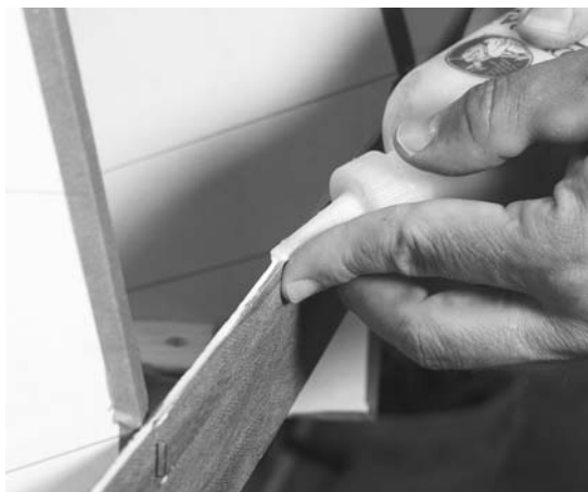
Figure 12-13. It doesn't take a lot of glue to secure the \frac{1}{8} -inch-thick strips in place, but it can be hard to direct it onto the narrow edge. It pays to have a fairly small hole in your glue dispenser so you don't get big drips coming out everywhere. With cove-and-bead strips it is quite easy to run the tip of the glue bottle down in the cove, but if you are applying glue to the bead or on a square-edged strip, you may find it helps to hold the bottle with your finger against the tip as a guide to run along the side of the strip.
