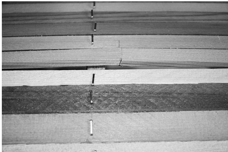
Figures 6-25 and 6-26. For really short cove-and-bead strips where you must fit them at both ends, there may not be enough room to bend and snap them in place. Instead I fit two separate pieces, one at each end, with enough length so they overlap in the middle. Cut an angled end on one piece and use it to mark the length of the second piece while they are dry-fitted in place. Then remove the strips and use the angled end of the cut piece as a guide to cut off the end of the second piece.
