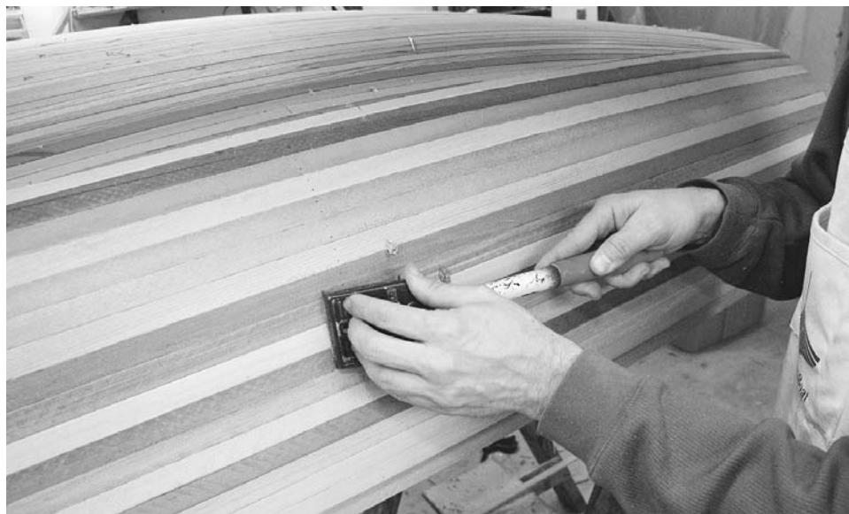
Figure 11-16. Use a sharp paint scraper to remove any glue drips. Hold the scraper with two hands, with one hand near the blade to keep it from chattering. Pull with the handle low and parallel to the boat surface. Since this boat uses cove-and-bead strips the surface is already pretty even. A quick scraping should get the surface into good shape to immediately start sanding. If there are any high spots, knock them down with a block plane.
