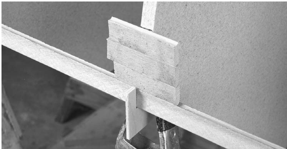
Figure 11-11. This boat has a little feature line approximately four strips down from the gunwale. To assure that it comes out even, stack up some strips, and align the top with that line so it will come out even later on. When the alignment looks right, run a staple through the strip into the form.
