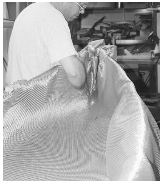
Figure 9-9. On the inside of this canoe I did not want any seams to disrupt the pattern of the carbon-Kevlar cloth, so I draped in the cloth in one piece and carefully trimmed near the stem. I initially left a little extra fabric around the stem area, and then cut it back to fit right up next to the stem. The top edge around the gunwale gets trimmed off about 1 inch above the edge.
