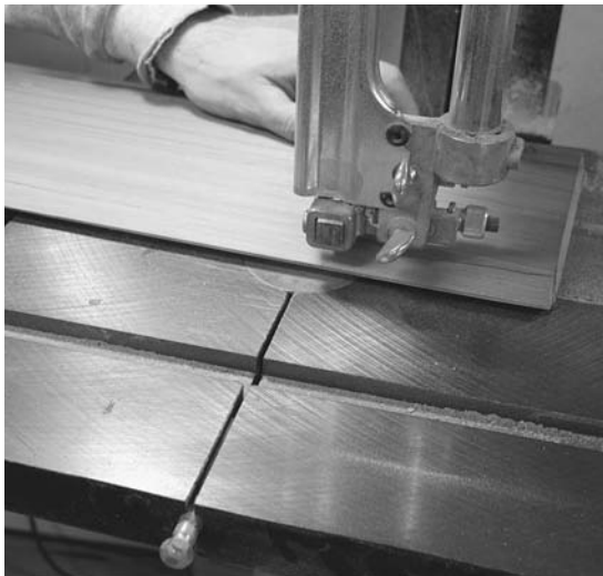
Figure 13-17. When the bevel is complete, cut the V-shaped stem off the board following the line for the back edge.
