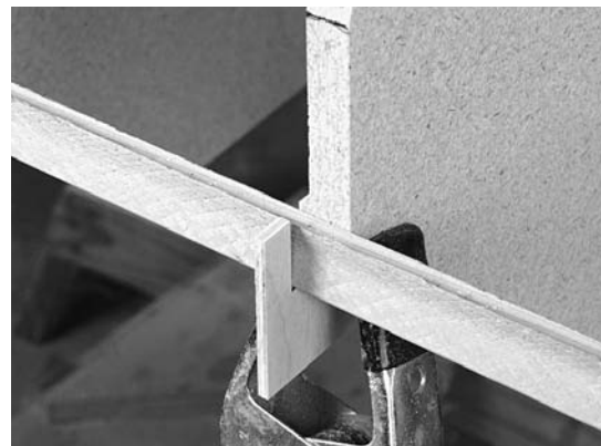
Figure 6-9. Getting the first strip aligned on the forms to create a smooth, fair curve may require a little finagling. Use some U-shaped jigs to temporarily hold the strip in place while checking the alignment. When you have it right, secure the strip in place with a staple or other fastener.
