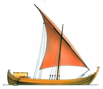
The steering oars were still brought within an extension of the upper hull; however, the stern and prow were far simpler, and the bowsprit gone completely. The ship's mast, stayed by shrouds, had a forward tilt to accommodate the double-sparred yard of a lateen sail, a feature probably copied from Arab vessels. Lateen sails could be trimmed much closer to the wind.
