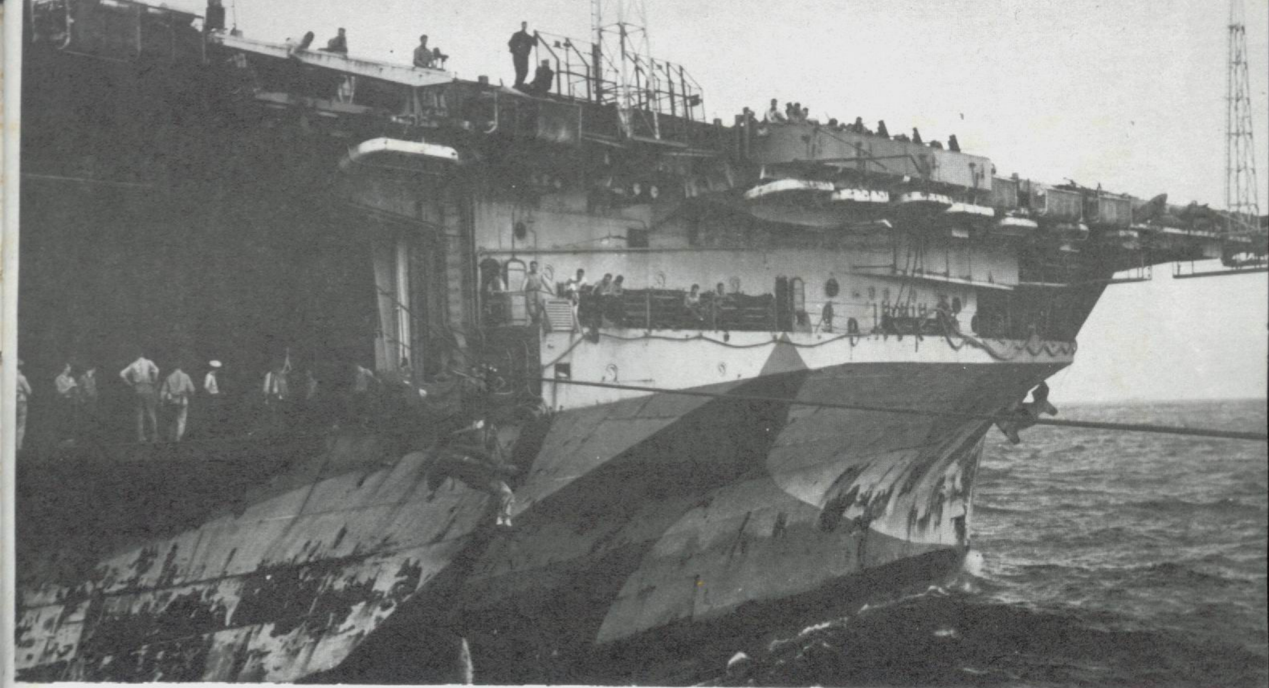
U.S.S. YORKTOWN (CV-10) off Formosa, January 21, 1945. Constant operations have taken their toll on her camouflage pattern. Dark green primer (84-D) and rust are in abundance. Note the difference between wet and dry paint and the contrast between the darkest panel (5-N) and the black boot topping. There appears to be no countershading under the flight deck overhang.
