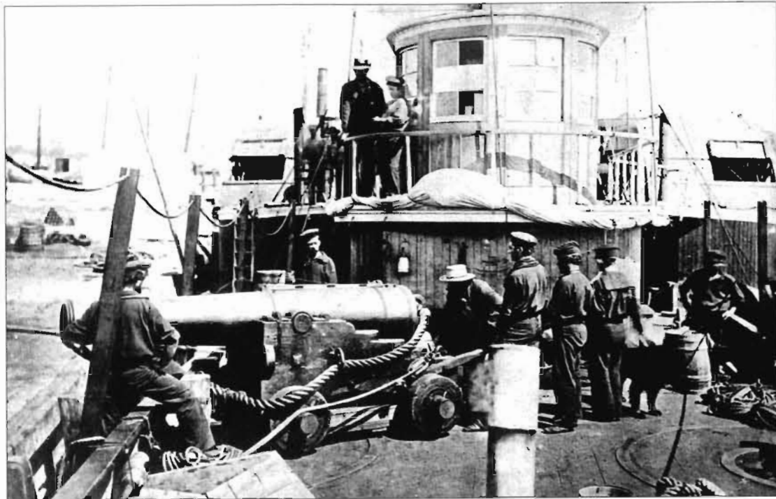
Even during the Civil War old guns and truck carriages were widely used, as may be seen in this photograph of US Navy steam tug Thomas Freeborn of the Potomac Flotilla in May 1861, shortly after the start of the war. (Naval Historical Foundation, NH 60990)
