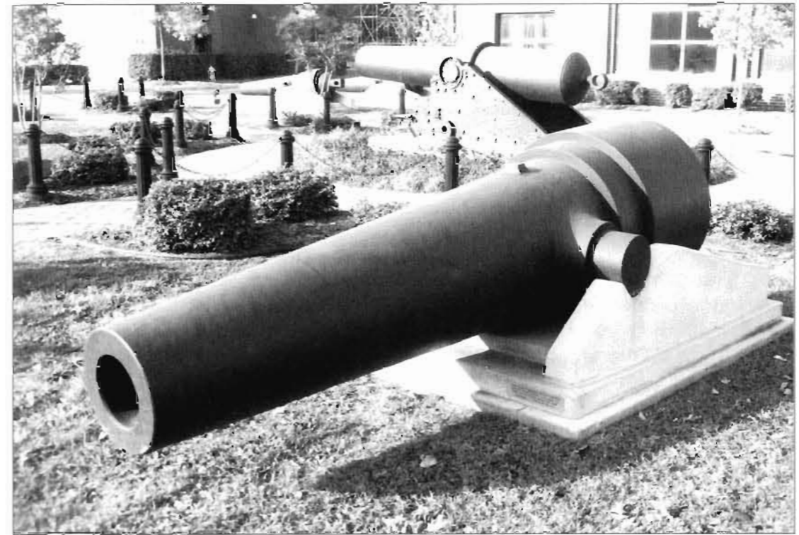
Confederate 10-inch Brooke double-banded smoothbore gun, reportedly cast for the ironclad Columbia . In the background is the Ericsson 12-inch wrought-iron smoothbore navy gun, made at the Mersey Iron Works in 1845 as the replacement for the 'Peacemaker': it apparently never saw service. (Washington Navy Yard, photograph by Malcolm Muir, Jr)
