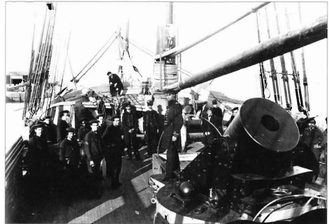
A 13-inch mortar aboard a US Navy mortar schooner. ( Library of Congress, B8184-10067 )
