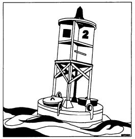
Figure 4-12.—Lighted buoy.
