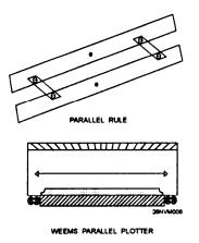
Figure 8-7.—A parallel rule (top) and a Weems parallel plotter.
