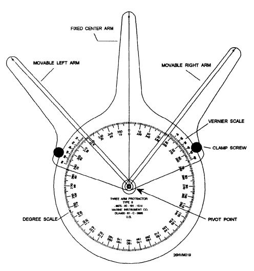
Figure 8-21.—Plastic three-arm protractor.
