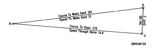
Figure 11-9.—Allowing for estimated current.
