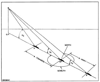
Figure 9-8.—Determining a LOP.
