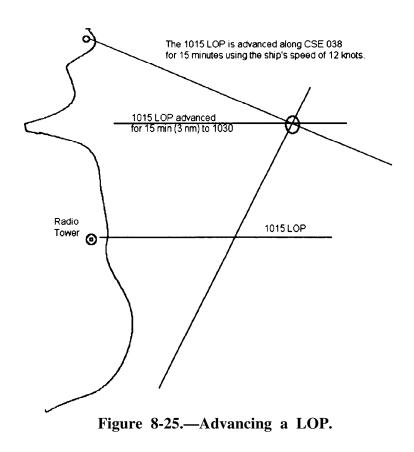
A running fix is labeled in the same manner as a visual fix except that the abbreviation R. fix is put beside the fix and fix time.
