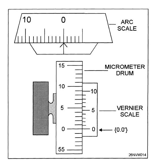
Figure 8-16.—A reading of 0.0 index error.
