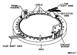
Figure 2-13.—Parts of a bearing circle.
