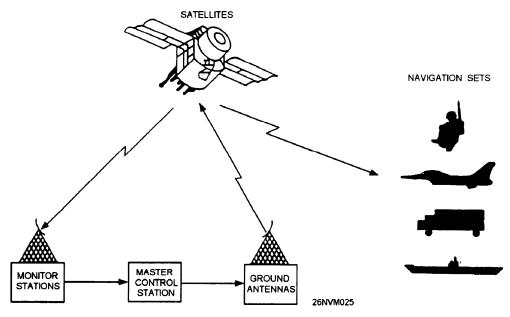
Figure 8-29.—Navstar global positioning system.
