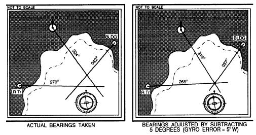
Figure 2-22.—Determing gyro error by adjusting bearings.
