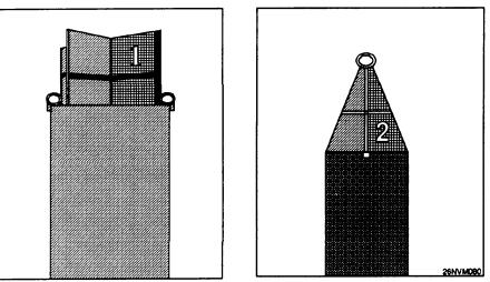
Figure 4-11.—Can buoy on the left and nun buoy on the right.
