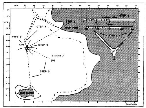
Figure 8-32.—Example of a radar fix.
