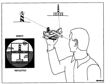
Figure 8-20.—Horizontal measurement of two objects.
