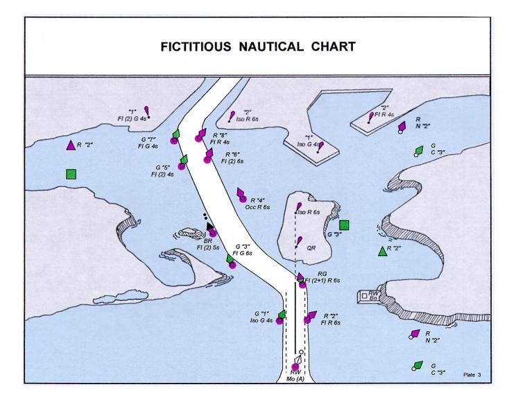
Figure 4-16.—How the visual guide would appear on a nautical chart.
