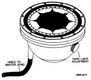
Figure 2-12.—Standard gyro repeater.
