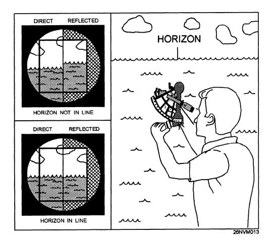
Figure 8-15.—Direct and reflected views of the horizon.
