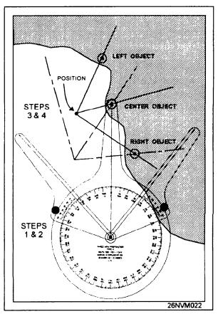
Figure 8-24.—Aligning the three-arm protractor.
