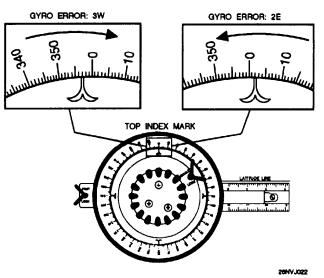
Figure 2-17.—PMP dialed in with gyro error.
