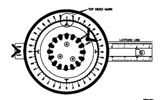
Figure 2-16.—PMP dialed in with 0° gyro error.
