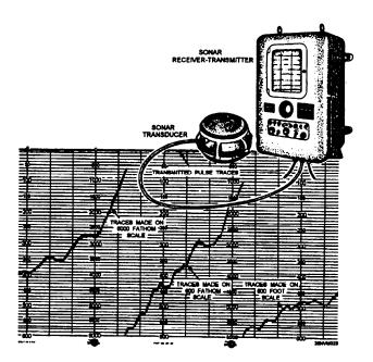
Figure 8-26.—Fathometer, transducer, and echogram.
