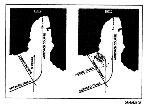
Figure 12-5.—Turn bearings and slide bar technique.
