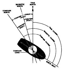
**Comment** Whether you are determining courses the helmsman is to steer, obtaining bearings to be plotted on a chart, laying track lines on the chart, or recording courses in the Magnetic Compass Record Book, knowing how to apply variation and deviation comes into play. The big question is "how do we convert one to the other?" Practice is needed to perform this task. However, keep in mind that you first need to reason each step, until later when the process becomes habit.
