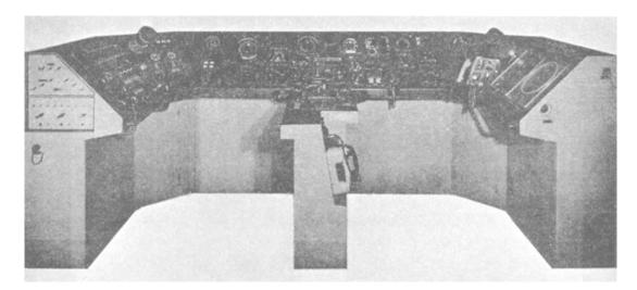
Figure 11-2.—FFG-7 class ship control console.
