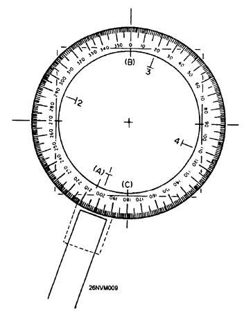
Figure 8-11.—PMP set up for relative bearing navigation.
