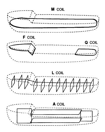
Figure 2-9.—Typical degaussing coil layout.
