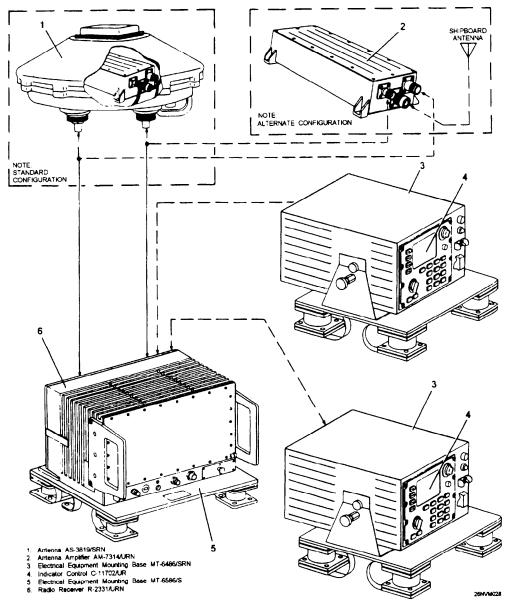
Figure 8-30.—Satellite Signals Navigation Set AN/WRN 6(V).
