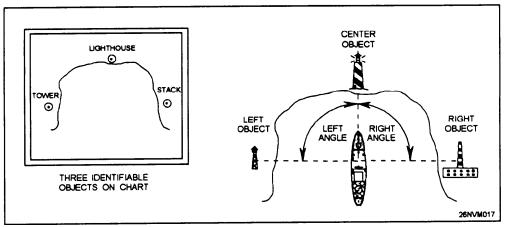
Figure 8-19.—Select three objects to obtain two angles.
