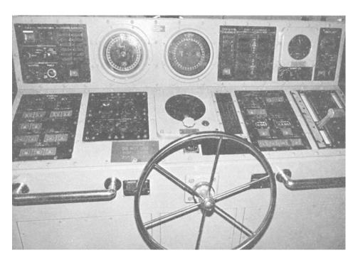
Figure 11-1.—DD 963 class ship control console.
