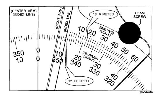
Figure 8-22.—Setting angle on the three-arm protractor.
