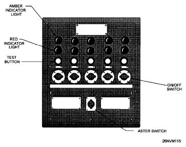
Figure 11-6.—Running light control panel.
