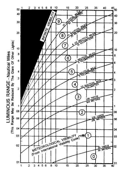
Figure 4-4.—Luminous range diagram.
