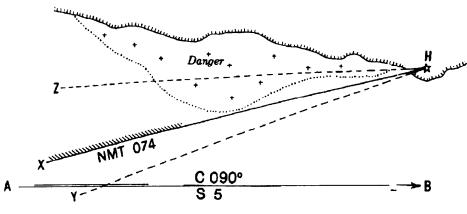
Figure 12-6.—Example of a danger bearing.
