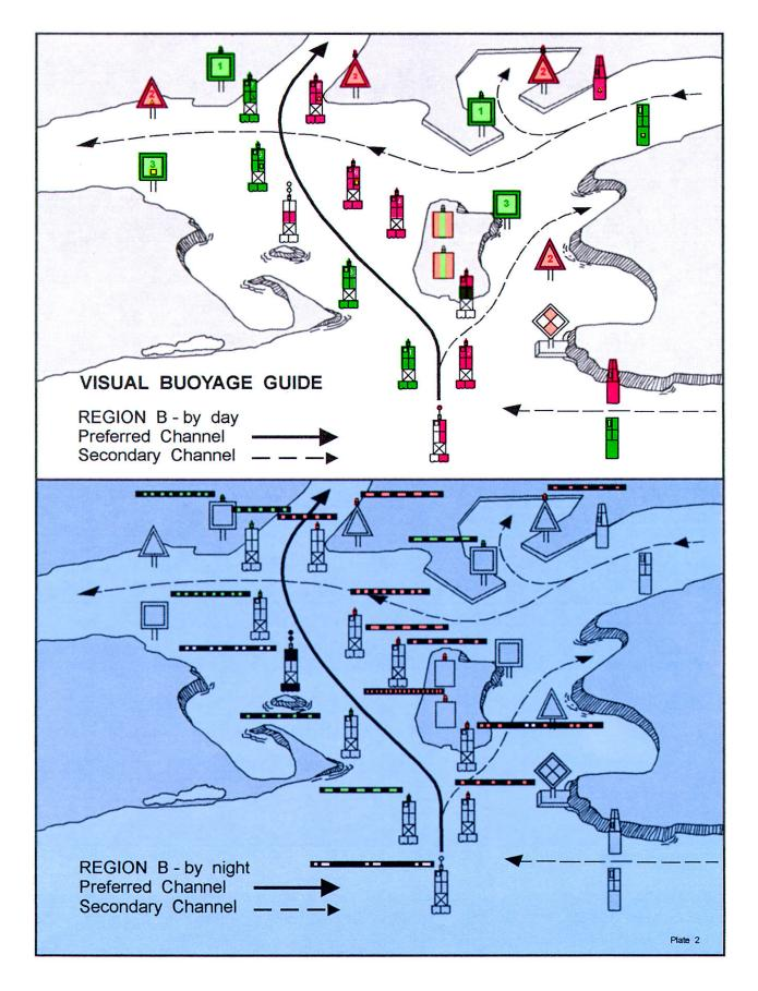
Figure 4-15.—Visual buoyage guide for IALA region B.
