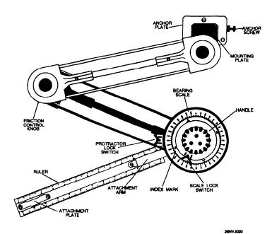
Figure 2-15.—Parts of a PMP.
