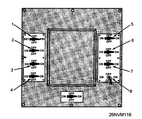
Figure 11-7.—Special light control panel.
