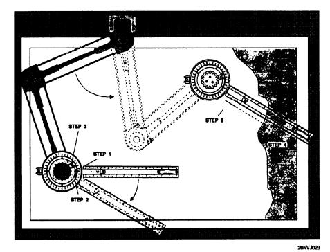
Figure 2-18.—How to plot with a PMP.
