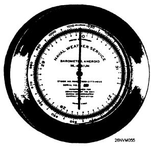
Figure 10-3.—Aneroid barometer.
