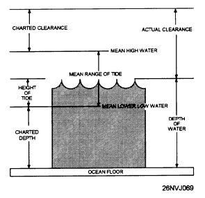
Figure 7-2.—Relationship of terms used when measuring heights and depths.
